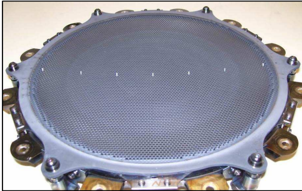
Figure 13: Ceramic pin arrangement for grid gap measurement
