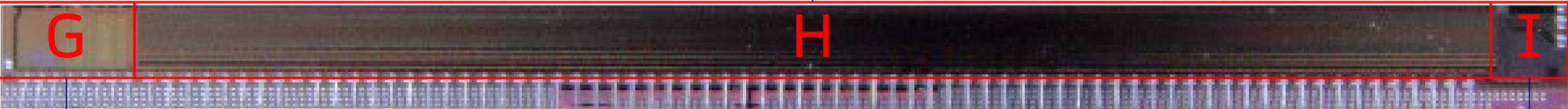
Bondpads for Analog supplies, digital supplies, IO, biases and tuners
