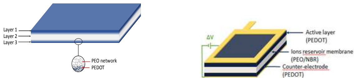
Figure 4 : Schematic representation of the tri-layer NBR/PEO/PEDOT IPN (up) and its connexion frame (down)
