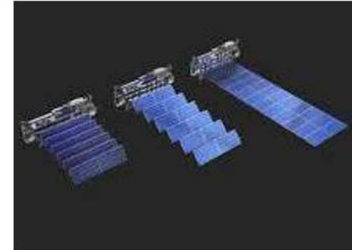
2: Accordion SA with central mast deployment on panel rear face
