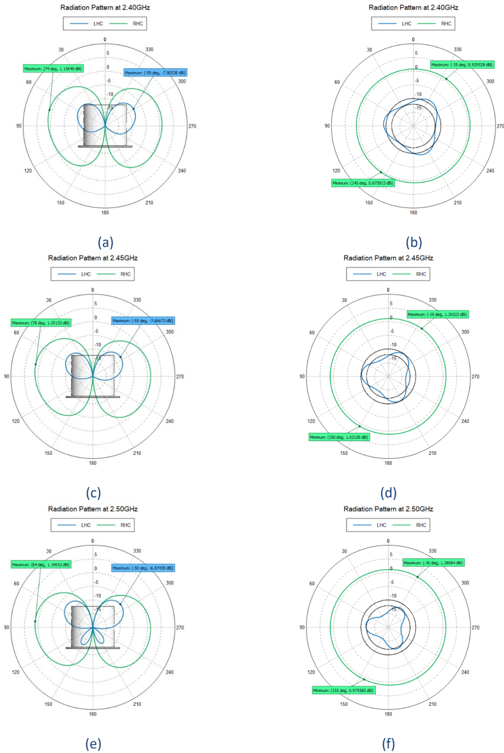
Figure 9. Antenna radiation performance at 2.40 GHz (a) side view and (b) top view, at 2.45 GHz (c) side view and (d) top view, and at 2.50 GHz (e) side view and (f) top view
