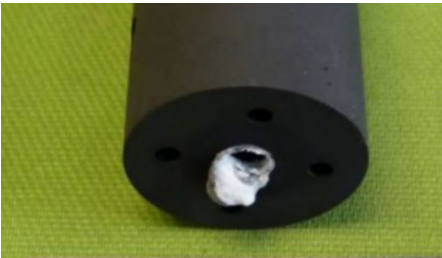
Damage to dispenser emitter
