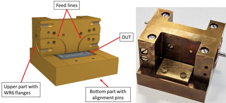
**Figure 4: CAD model of the optimized WR6-band measurement holder (left) and fully assembled measurement holder (right). DUT means device under test.**
