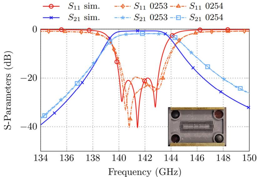
**Figure 5: Measurement results of the third order WR6-band GGW filters 04818\_0253 and 04818\_0254 compared to simulation.**
