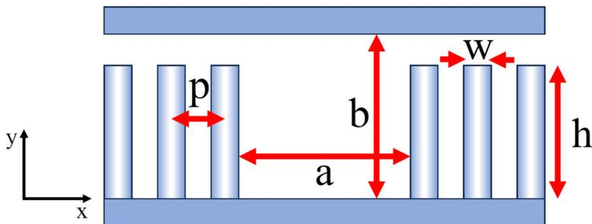
Figure 2: Cross-section of the GGW. Dimensions are as follows (all in mm):  $a = 1.651$ ,  $b = 0.8255$ ,  $h = 0.79$ ,  $p = 0.45$ ,  $w = 0.3$ .
