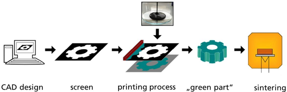
Figure 1: Process chain of the 3D screen printing process.
