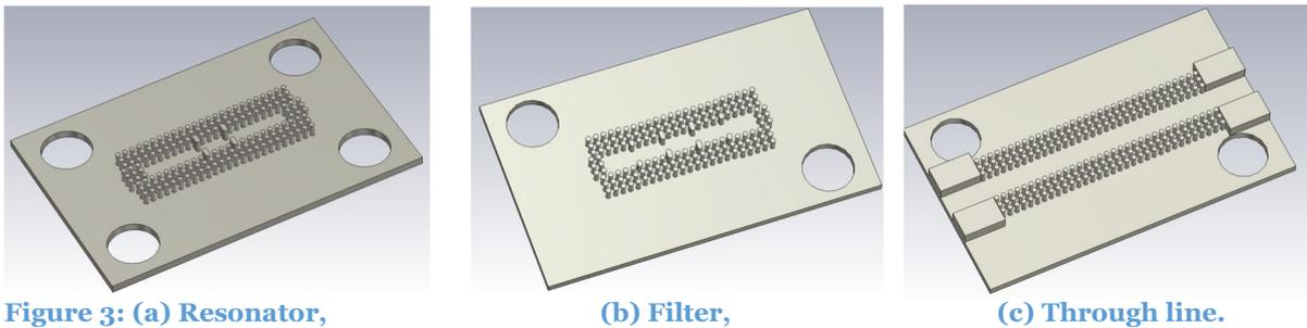
These components were characterized electrically and geometrically, with results showing that the 3D screen printing process can produce GGW components that perform well at high frequencies. The measured components showed good agreement with simulated designs, though there were some discrepancies in the exact center frequencies and insertion losses, which were attributed to minor dimensional deviations during the printing and sintering processes.
