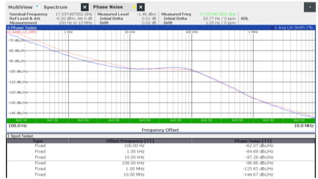
Fig. 7. Measured versus modelled LO Phase Noise @ 25°C, 17.0375 GHz
