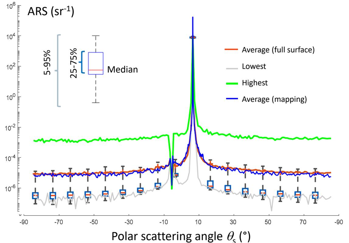
→ Efficient & robust full surface scattering assessment (30x30mm<sup>2</sup> in 1.5h; +/- 90° )
