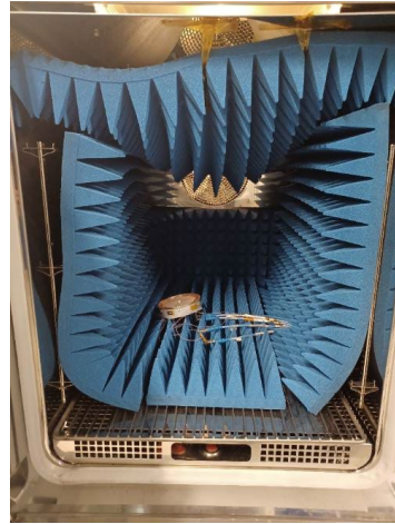
Figure 7-11 antenna element inside the thermal chamber covered with absorbers
