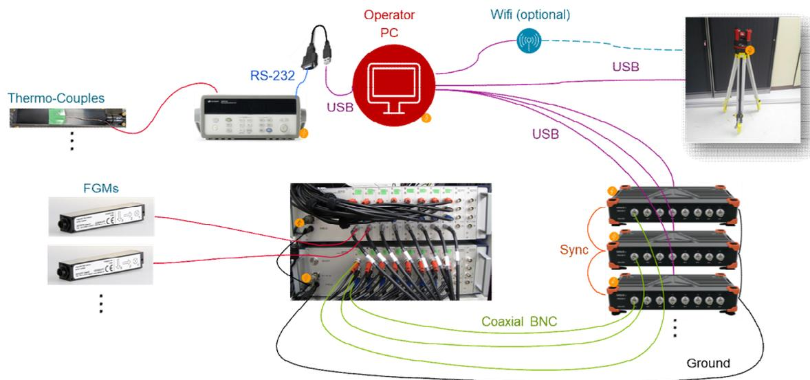
**Figure 1-11: Electrical interfaces.**
