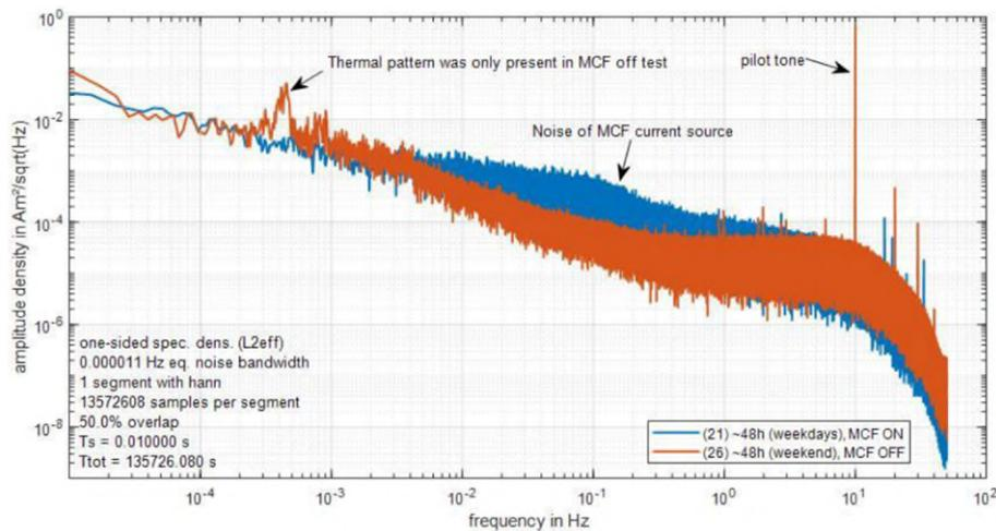
**Figure 1-6: Comparison between compensation coils ON (blue) and OFF (red), with pilot tone.**
