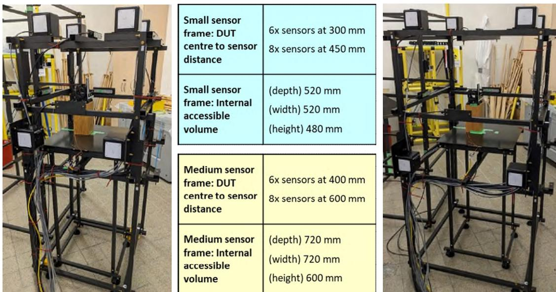
Figure 1-9: ADAM carbon fibre mechanical sensor frames (left) small (right) medium sized.
