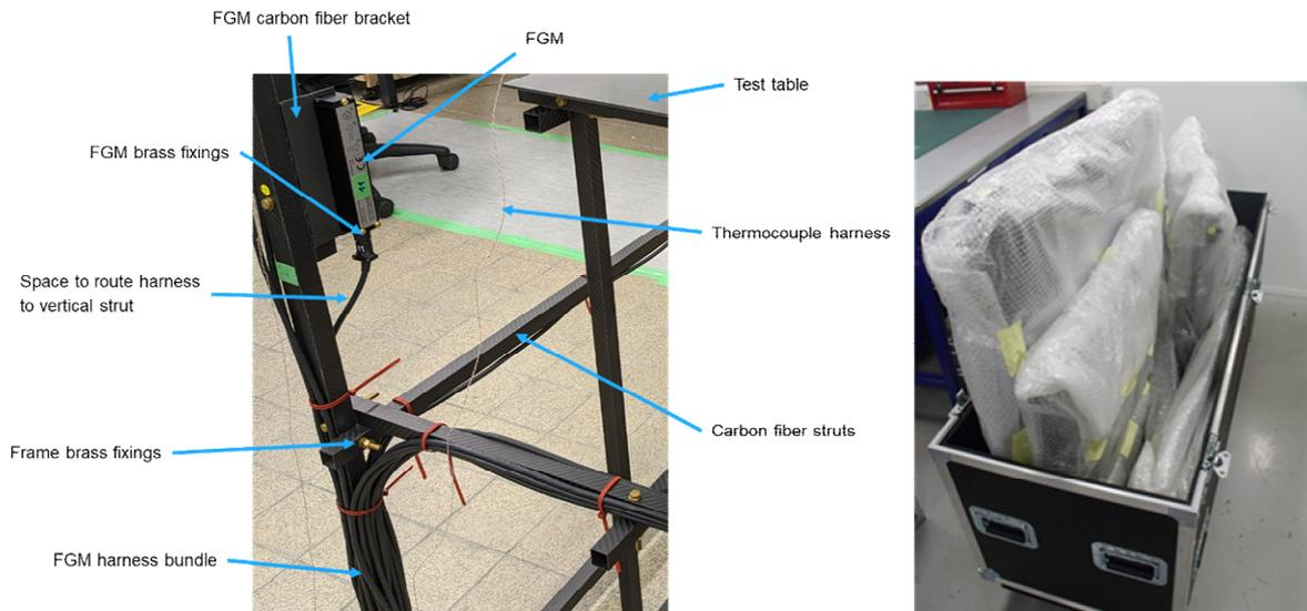
**Figure 1-10: (left) sensor frame elements (right) transportation case.**
