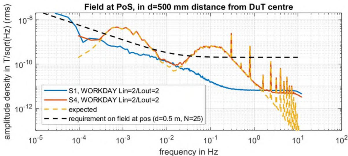
**Figure 1-14: Recovered DuT contribution matching predicted field closely.**
