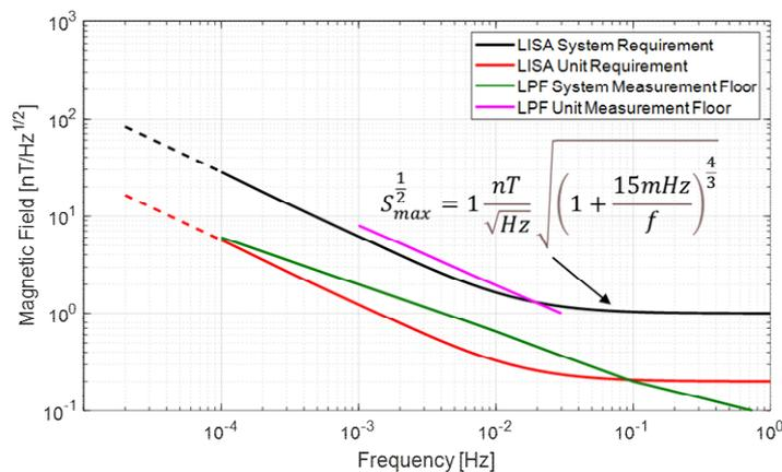
**Figure 1-2: ASD system level to unit level apportionment, compared to LPF facilities performance**
