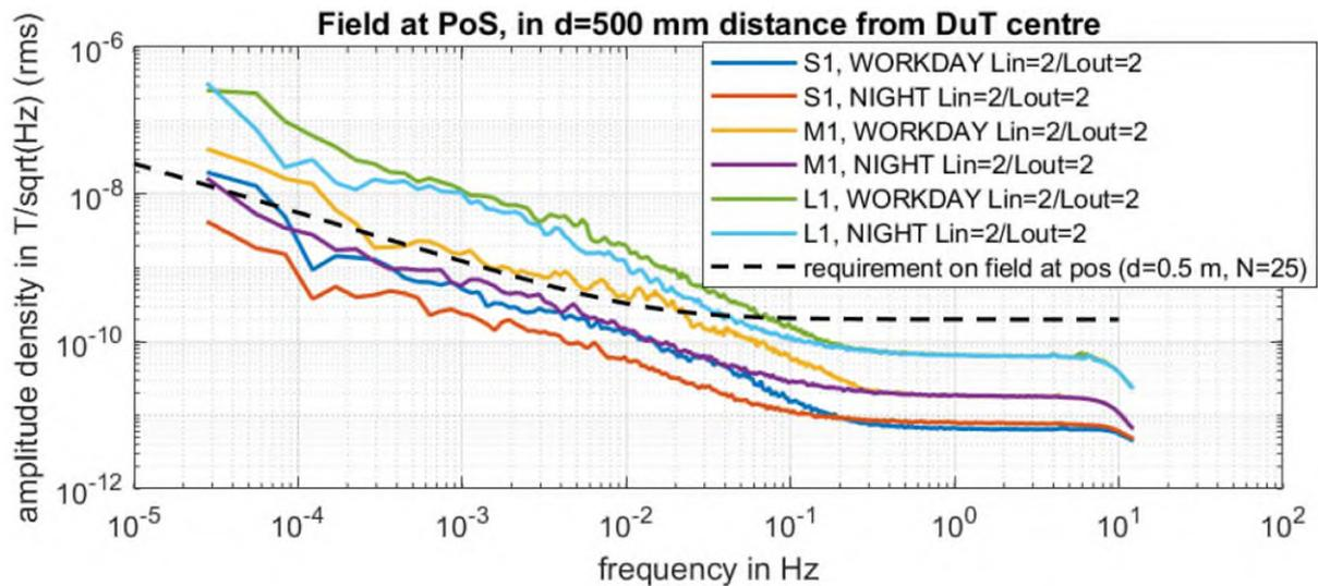
Figure 1-13: ASD ambient performance for all sensor frame scale sizes, during different times.
