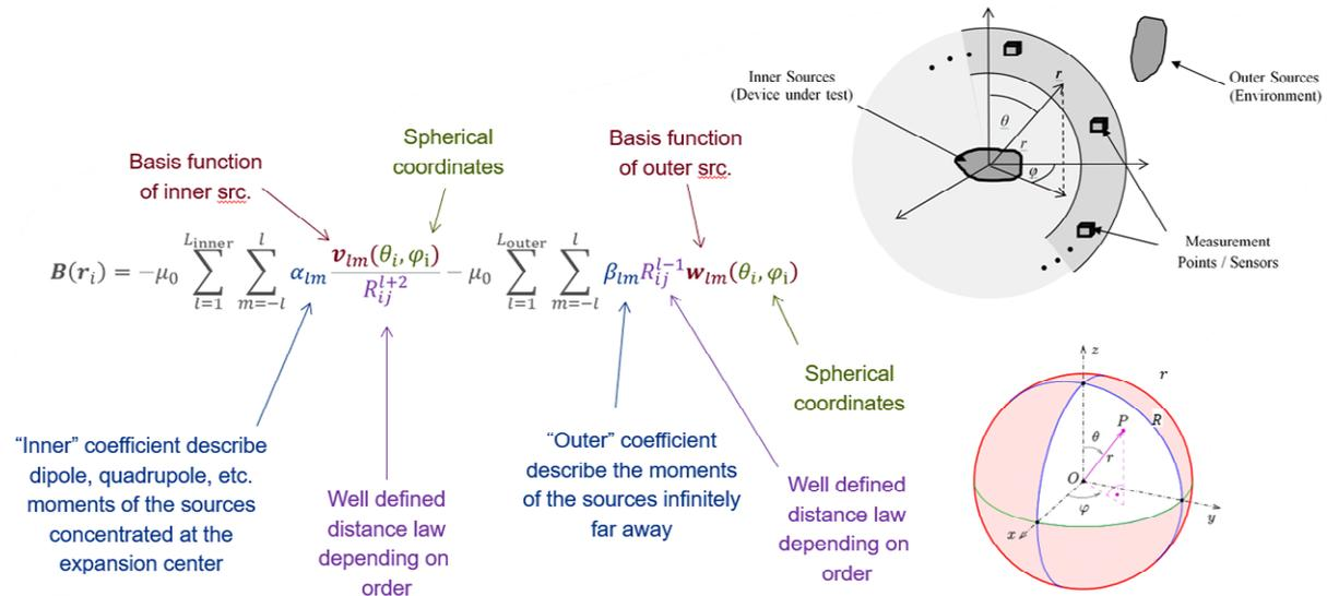
Figure 1-5: Spherical harmonics multipole expansion.
