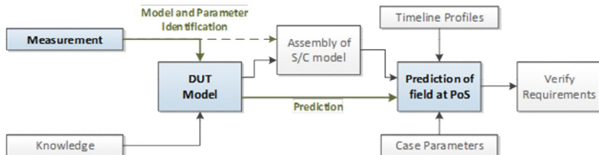
**Figure 1-4: Structure and Objective of Data Processing Methods**
