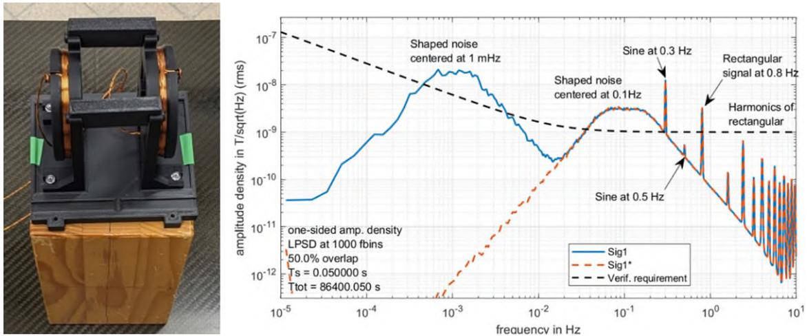
Figure 1-12: Synthetic DuT models (left) Quadrupole and Large Loop (right) shaped noise signal.
