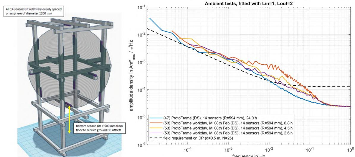
**Figure 1-7: (left) Model of the demonstrator frame (right) ASD of fitted dipole moment into ambient test data with demonstrator frame measured on a weekday, fitted with Lin=1, Lout=2.**
