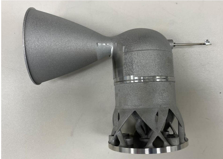
Figure 6-10: DM1a Hardware (assembled fully functional thruster with pc tube)
