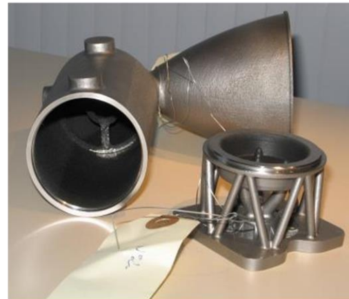
Figure 9-2: ALM printed 240N Roll control Thruster [RD 2]
