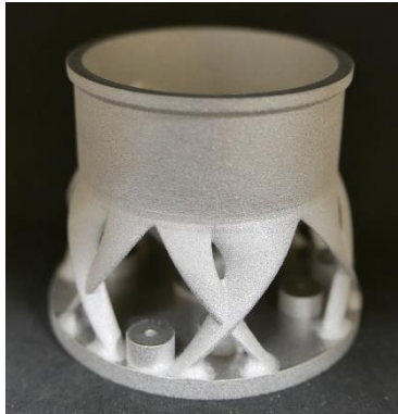
DM1a printed Heat Barrier (cat chamber at the top)
