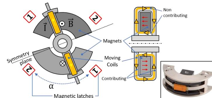
Voice coil configuration 1 (Rotary Voice Coil Actuator)
