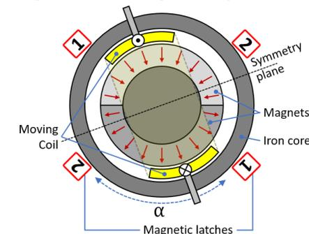
Voice coil configuration 2 (Cylindrical Voice Coil Actuator)
