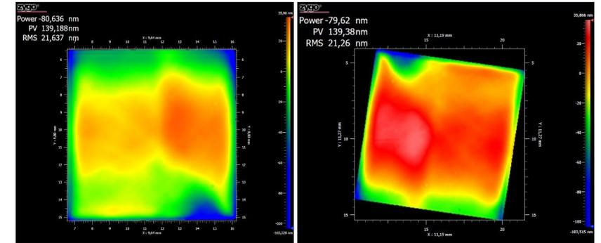
KTP laser crystal before and after soldering
