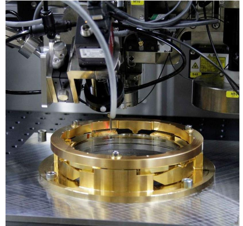
Lens Soldering Setup
