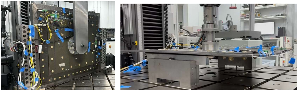
Figure 8 Component level - quasi static test set up , two load cases
