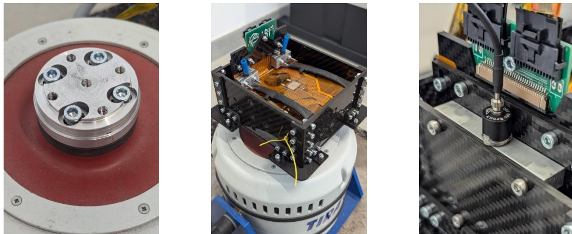
Figure 21. Setup of x-axis vibratory test of DSA-M. Left: the mechanical interface. Center: the DSA-M mounted. Right: the accelerometer.
