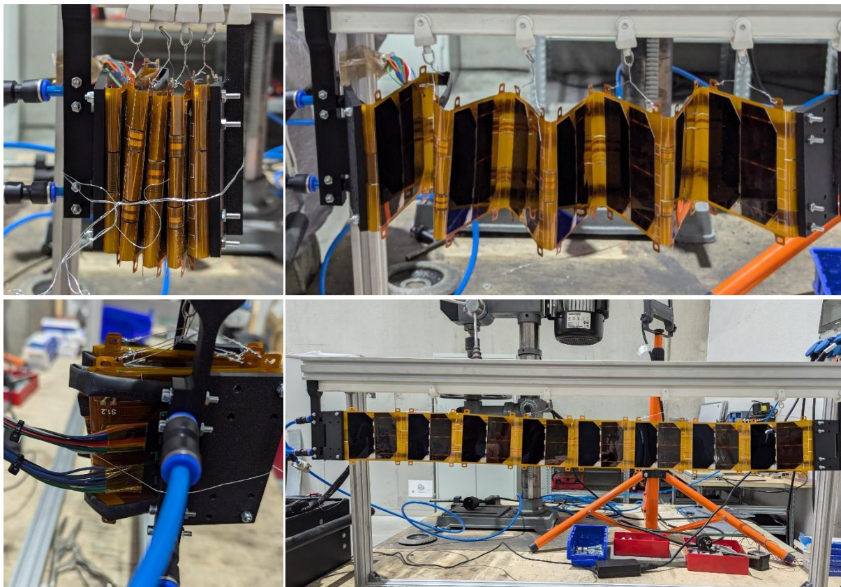
Figure 19. Setup of deployment test: the DSA-M mounted in stowed configuration (top-left), a highlight of the data interface of the DSA-M (bottom-left), the DSA-M released from stowed configuration (top-right) and the DSA-M deployed with inflation.
