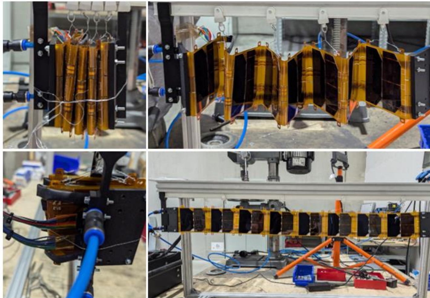
Setup of deployment test: the DSA-M mounted in stowed configuration (top-left), a highlight of the data interface of the DSA-M (bottom-left), the DSA-M released from stowed configuration (top-right) and the DSA-M deployed with inflation
