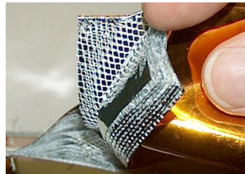
MLI Blankets showcasing internal fibre netting.
