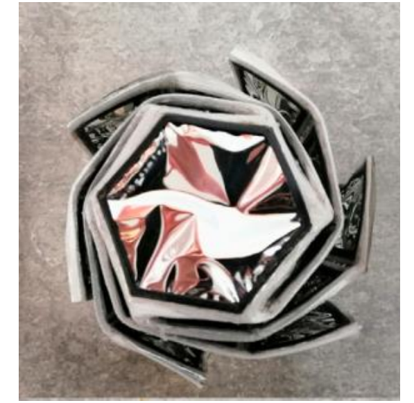
Deployed Solar Sail Mockup at DLR (left) and deployed/folded (center/right) solar sail feasibility model.
