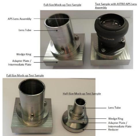
Figure 4-2: Star Tracker Test Sample configurations
