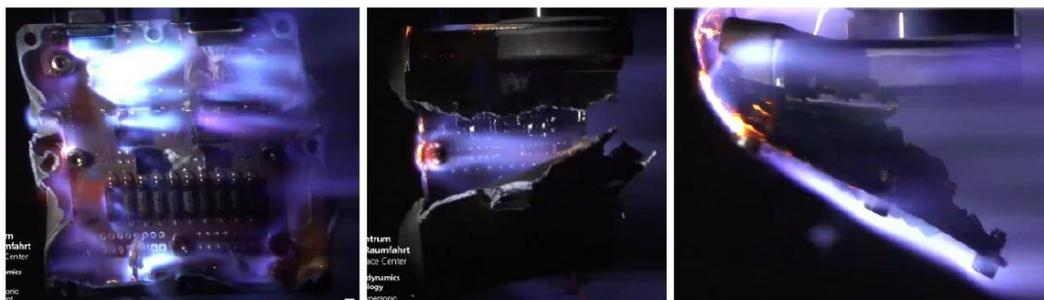
Figure 4-63: BCM after cover plate removal (left), failing of housing (centre) and board remains just before the end of the test (right)
