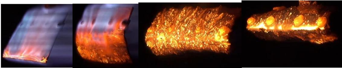
Figure 4-53: Delamination of GFRP layers at the leading after 5 s (left) and bending of the board around the sample holder after 25 s; Melting of EnMap board at the middle and just before the of the test (right)
