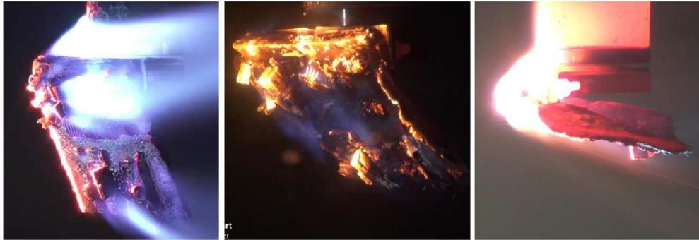
Figure 4-62: Images from video cameras of PD board test after 60 s (left), 108 s (centre) and 172 s (right) test time
