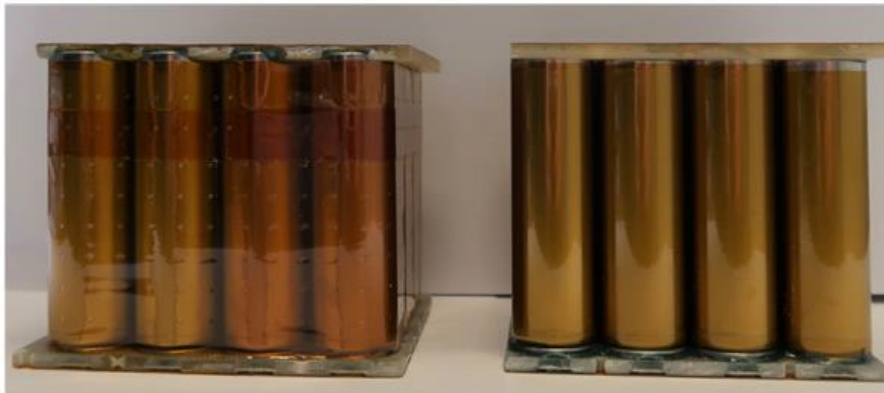
ABSL Mini-Module with Individually Wrapped Cells
