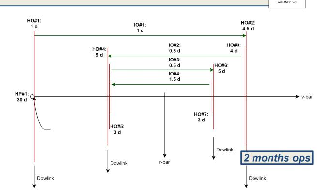
GS contact is established during the hold orbits, in the Communication phase, to downlink data and to check the spacecraft conditions before re-entering in the Inspection phase.
