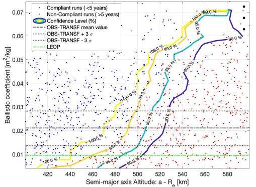
**Ballistic coefficient** and **initial mean altitude** strongly influence the decay time. During **LEOP** the panels are folded: lower ballistic coefficient  $\rightarrow$  lower safe altitude During **TRANSFER** and **INSPECTION** phases the panels are deployed: higher ballistic coefficient  $\rightarrow$  higher safe altitude
