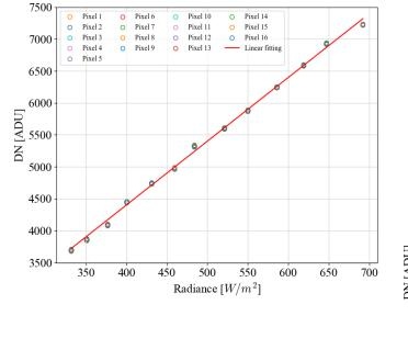
Camera response function varying camera-plate distances in **non vacuum;** plate temperature fixed at 39 °C.
