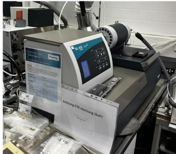
Figure 18 (left) Orientation of CTE samples relative to build-up direction of additively manufactured disc (red arrow). (right) Dilatometer used for CTE tests.
