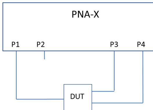
Figure 5-120 : Small-signal 3-port measurement setup, using the internal couplers in the PNA-X (limited to maximum 30 dBm output power per port).
