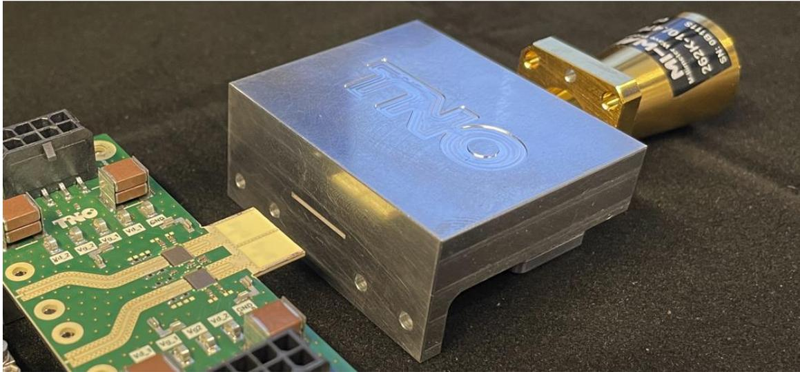
Figure 6-36 DRIFT waveguide viewed from the waveguide exciter side.
