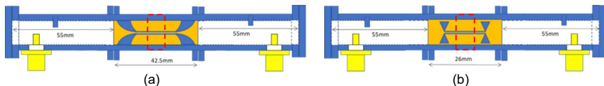
Figure 5-124: Alternative test for measuring the losses of the exciter options. The red dashed box in the centre indicates the piece of parallel line where it is outside the wave guide and connects to free space.
