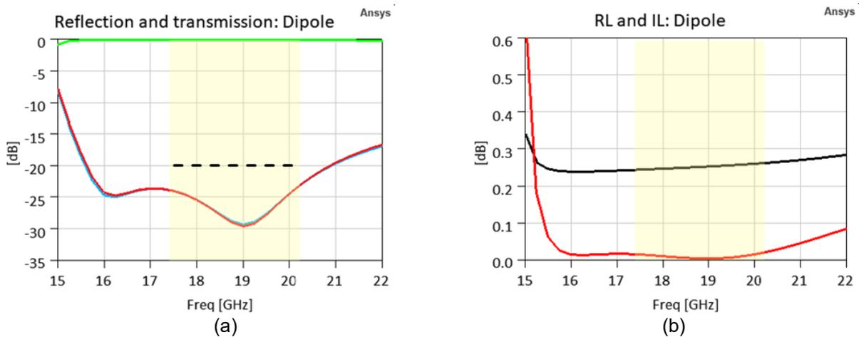
Figure 5-54: Dipole exciter tuned performances. (a) Reflection and transmission, and (b) reflection- (red) and insertion (black) losses. Results are valid referenced to indicated plane in schematic.
