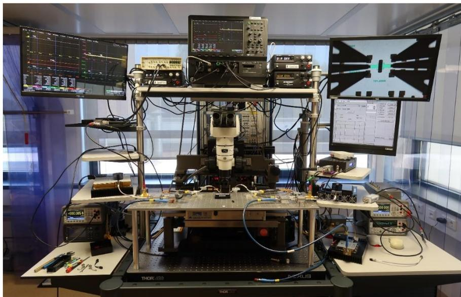
Figure 5-11 : Active load pull setup (with the ZVA at the back side of the probe station).
