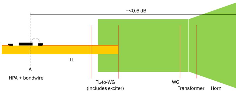
Figure 5-41: Schematic representation of the relevant front-end radiation section defining the loss indicated in Table 5-11.
