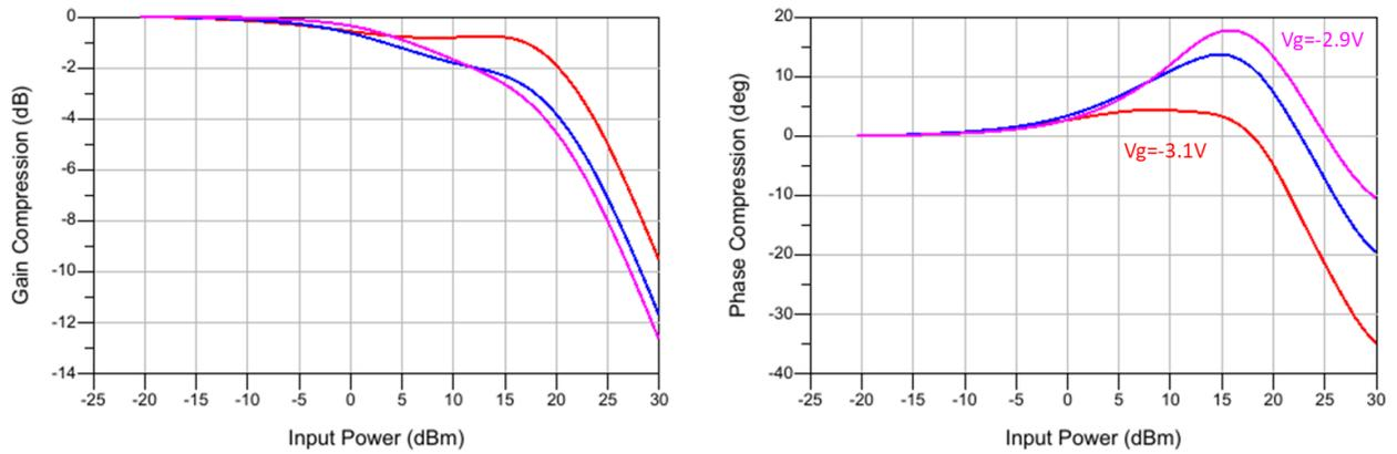
Figure 5-34 : Power sweep at 18.8 GHz,  $V_d=20V$ ,  $T_a=80^{\circ}C$ , for  $V_g=-3.1$  to  $-2.9$  V.
