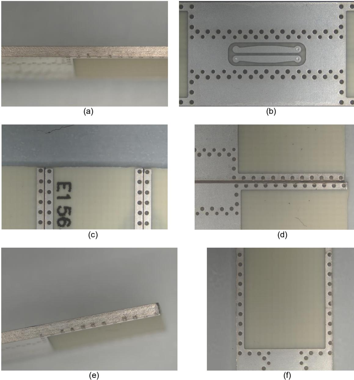
Figure 5-96: PCBs manufactured by Eurocircuits. (a) Silver plated edge, (b) parallel line with vias neatly placed in the pads. (c) View on the milled edges of the PCBs, (d) via placement on the edges in some cases is off centre, and (e) results in open voids on the PCB's edge. (f) Rough metal edges.
