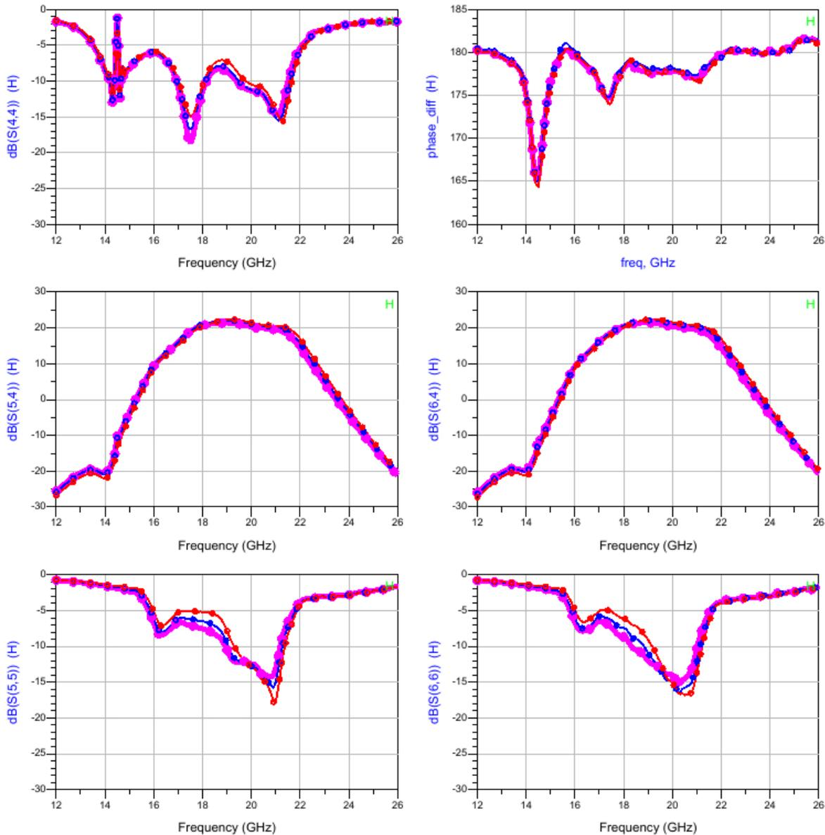
Figure 6-11 S-parameter measurements on sample R2C2 at  $V_d=20V$ ,  $V_g=-3.23V$  for  $T_a=25degC$  (red),  $50degC$  (blue) and  $75degC$  (magenta).
