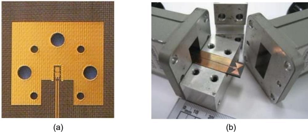
Figure 5-10 : Differentially-fed patch exciter at V-band [19] (a), slot line coupled bow-tie exciter at X-band [20] (b).
