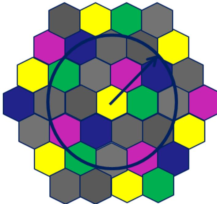
Figure 5-2 : frequency reuse scheme (7 colors)
