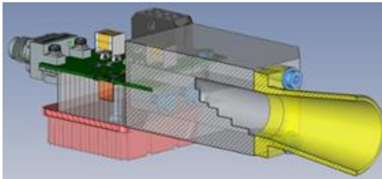
Figure 5-106: Cut-away impression of the designed septum polariser and COTS horn section with dipole exciter for the active demonstrator.
