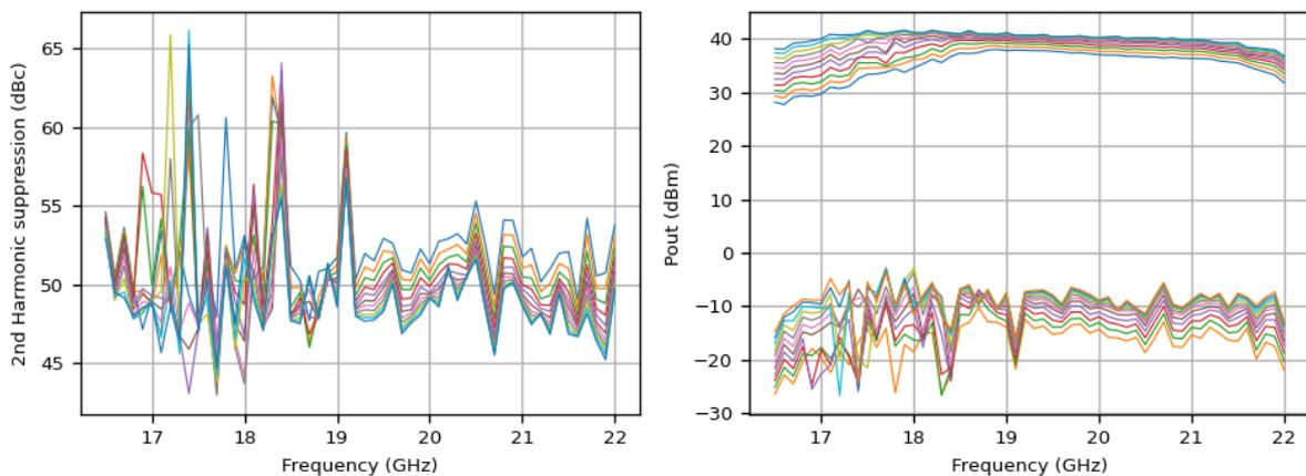
Figure 6-20 CW power-frequency sweep for a source power of 15-25 dBm (1 dB step), at the nominal quiescent bias current of 140 mA and 20V, 25degC, sample R2C1, showing the 2<sup>nd</sup> harmonic suppression and differential output power of the fundamental and 2<sup>nd</sup> harmonic.
