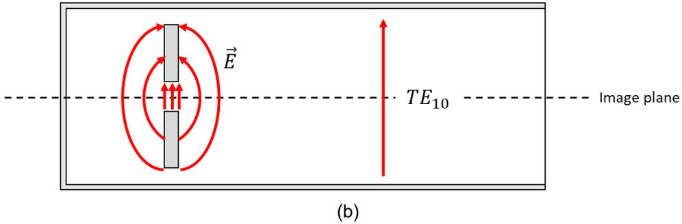
Figure 5-43 : (a) Monopole (E-probe) in waveguide to excite the fundamental waveguide mode, and (b) from image theory two monopoles generate the same field configuration and compose exactly a dipole.
