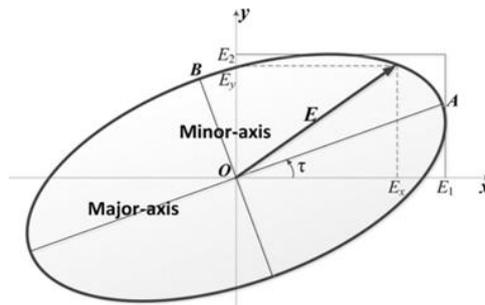
Figure 6-48: Polarisation ellipse, minor and major axis [21].
