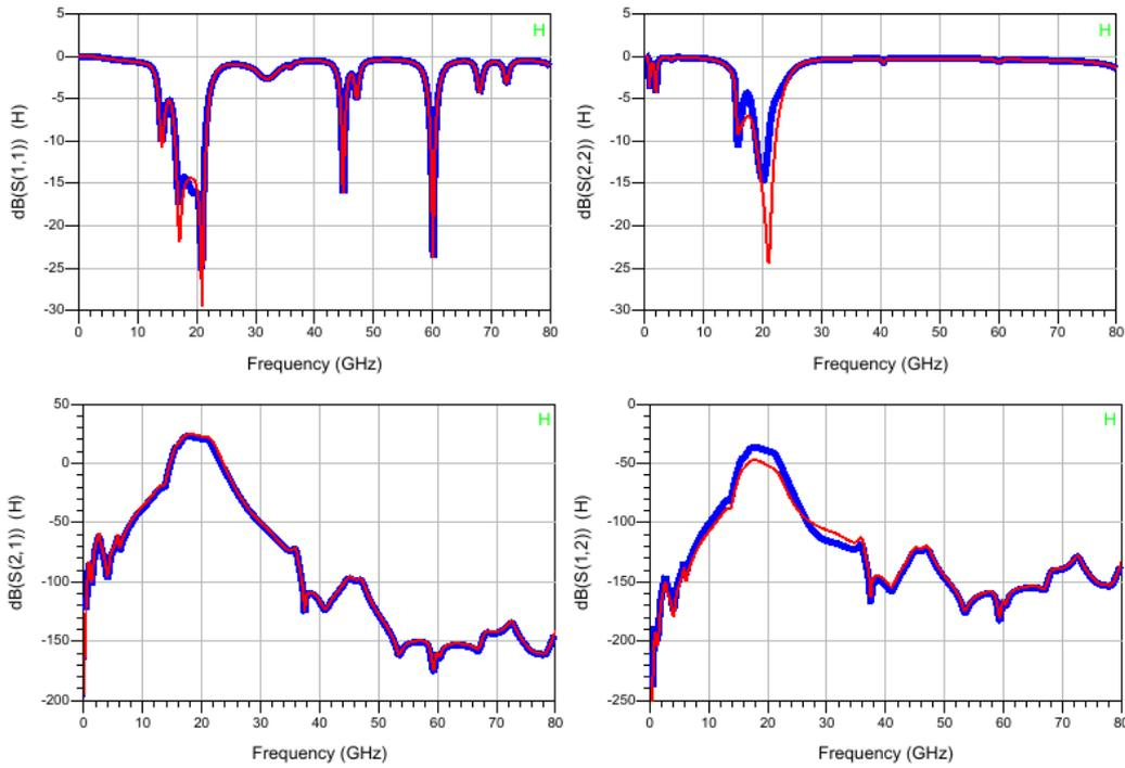
Figure 5-69 : Wide-band S-parameters for the HPA using an ideal balun at the output,  $V_g=-3.0V$  (20degC) and  $V_g=-3.1V$  (80degC),  $V_d=20V$ ,  $T_a=20degC$  (red) and 80degC (blue).
