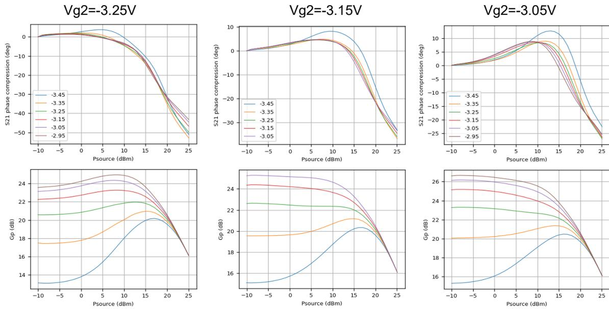
Figure 6-23 : Power sweeps at 19 GHz for different  $V_{g1}$ ,  $V_{g2}$  combinations at  $V_d=20V$ ,  $80degC$ , sample R2C1.
