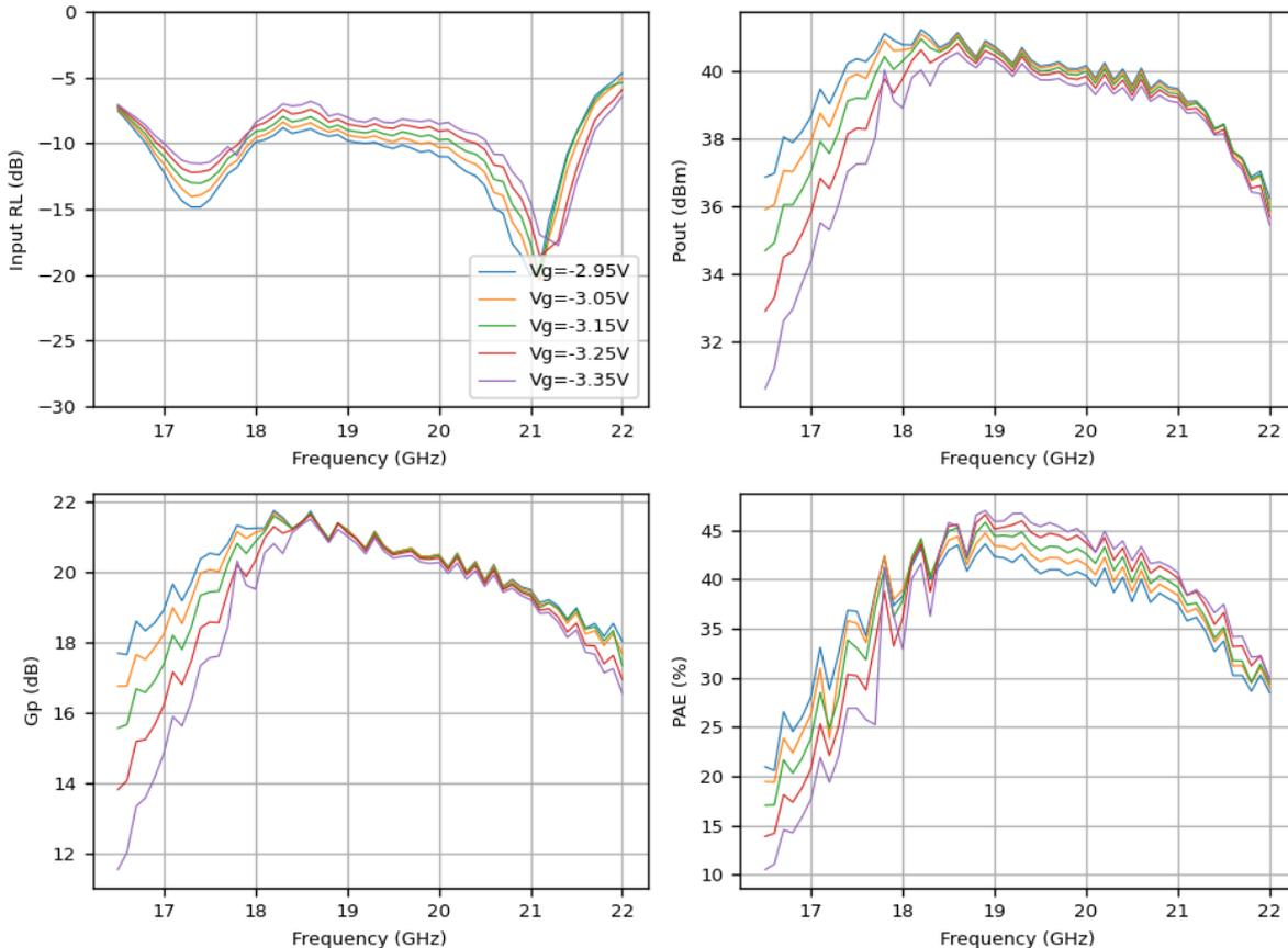
Figure 6-14 : Measured frequency sweep for a source power of 20 dBm, versus gate bias voltage at 20V, 25degC, sample R2C1.
