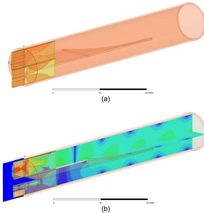
Figure 5-51: (a) Model including two exciters and the septum polariser. (b) Magnitude of the electric field distribution (logarithmic) at 19 GHz. Total length of the model is in the order of 55mm, excluding the length of empty circular waveguide.
