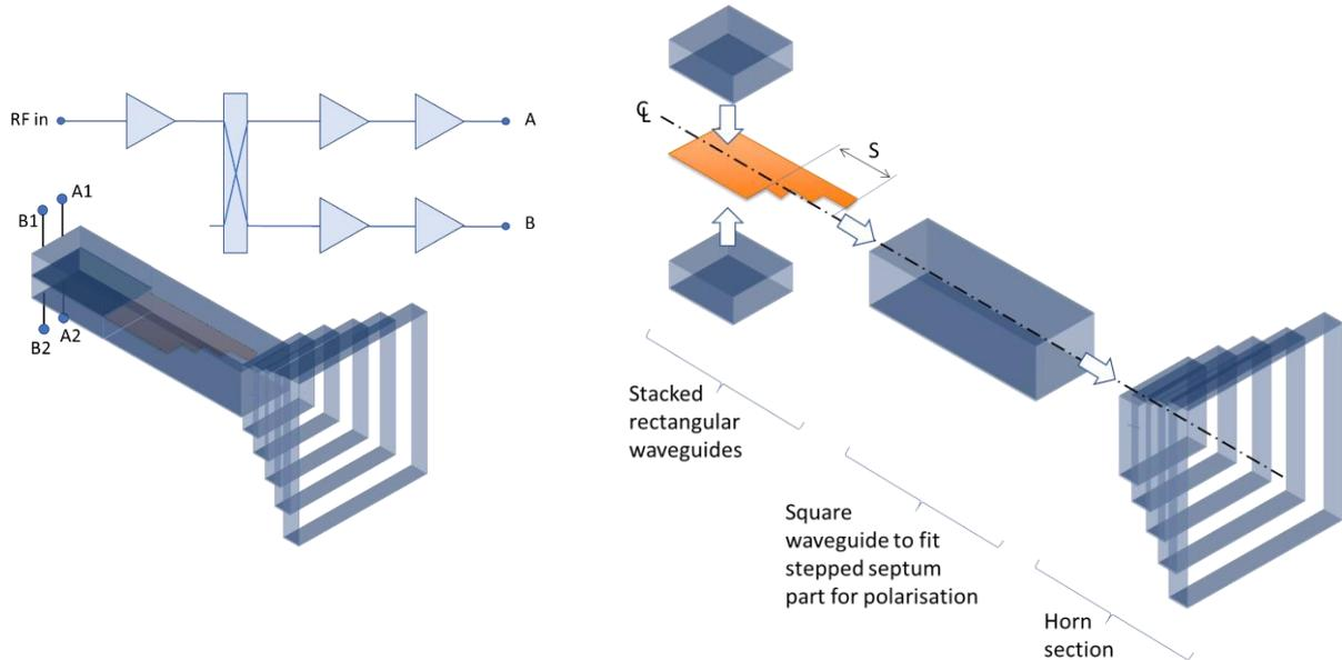
Figure 5-5: (a) 3D impression of the arrangement including the septum in a square waveguide to obtain the two dual circular polarisations. Note also that both rectangular waveguides will have access points to connect with a differential HPA. (b) Exploded view indicating the distinctive sections of the arrangement. The square waveguide will accommodate length  $S$  of the septum.
