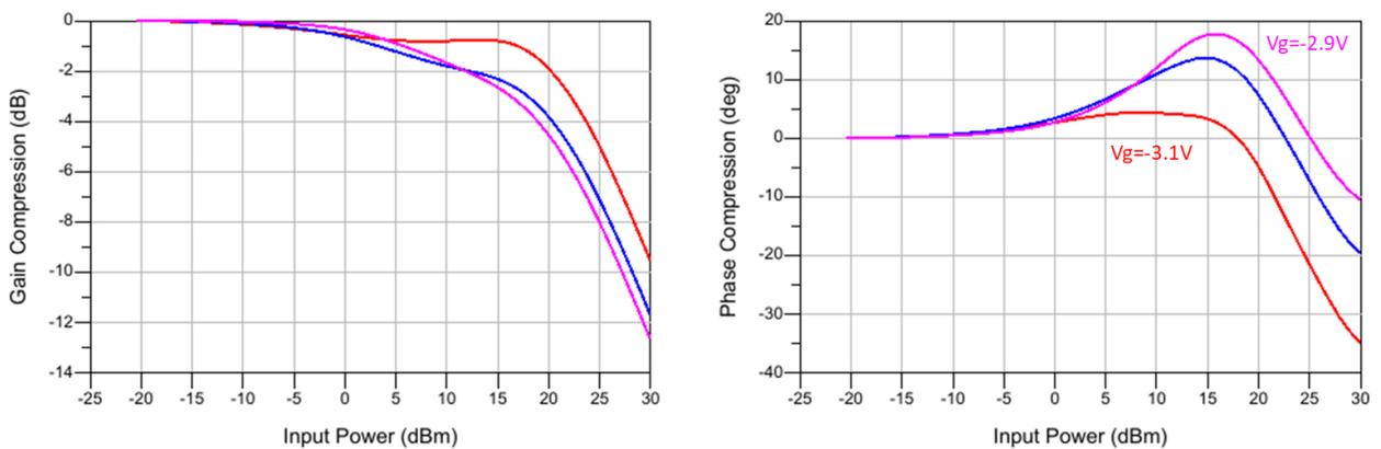
Figure 6-22 : Simulated power sweep at 18.8 GHz, Vd=20V, Ta=80°C, for Vg=-3.1 to -2.9 V.
