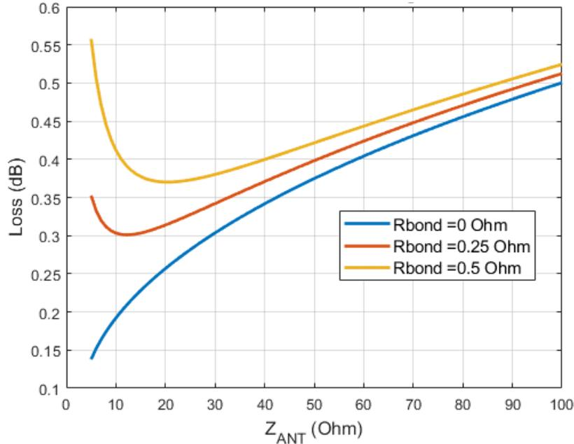
Figure 5-38 : Example simulation of the impact of the series resistance of a bondwire on the loss of the output matching at 18.8 GHz.
