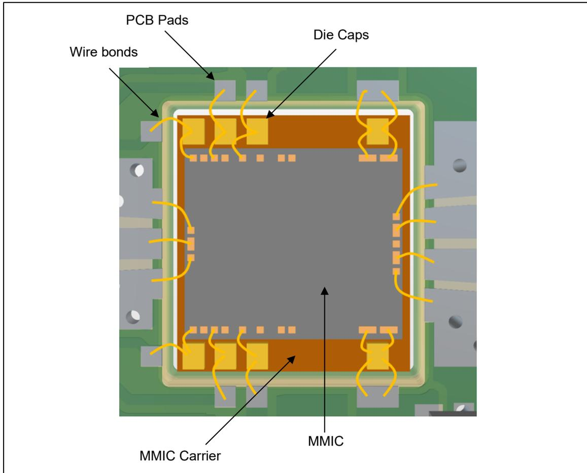
Figure 5-117 Detailed view of HPA MMIC assembly and wirebonding.
