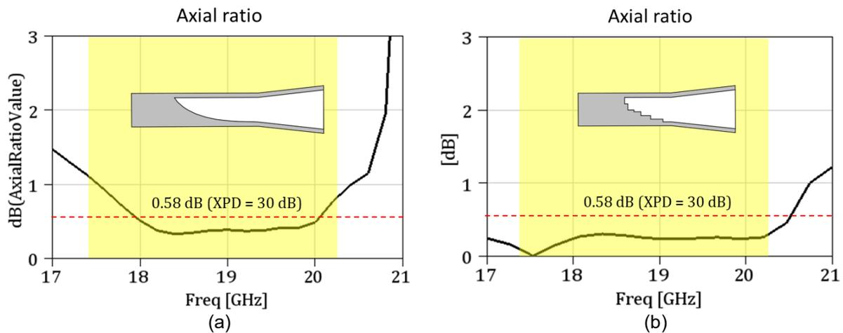
Figure 5-102: Simulated axial ratio for: (a) exponentially tapered septum, and (b) stepped septum.
