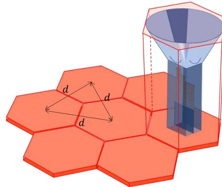
Figure 5-40: radiating front-end in a hexagonal grid
