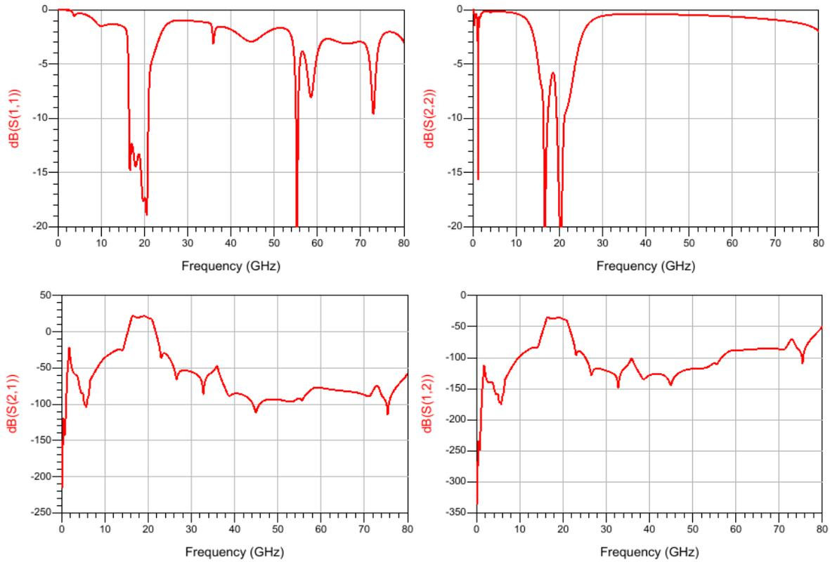
Figure 5-25 : Wide-band small-signal S-parameters for the HPA including an ideal balun at the output.
