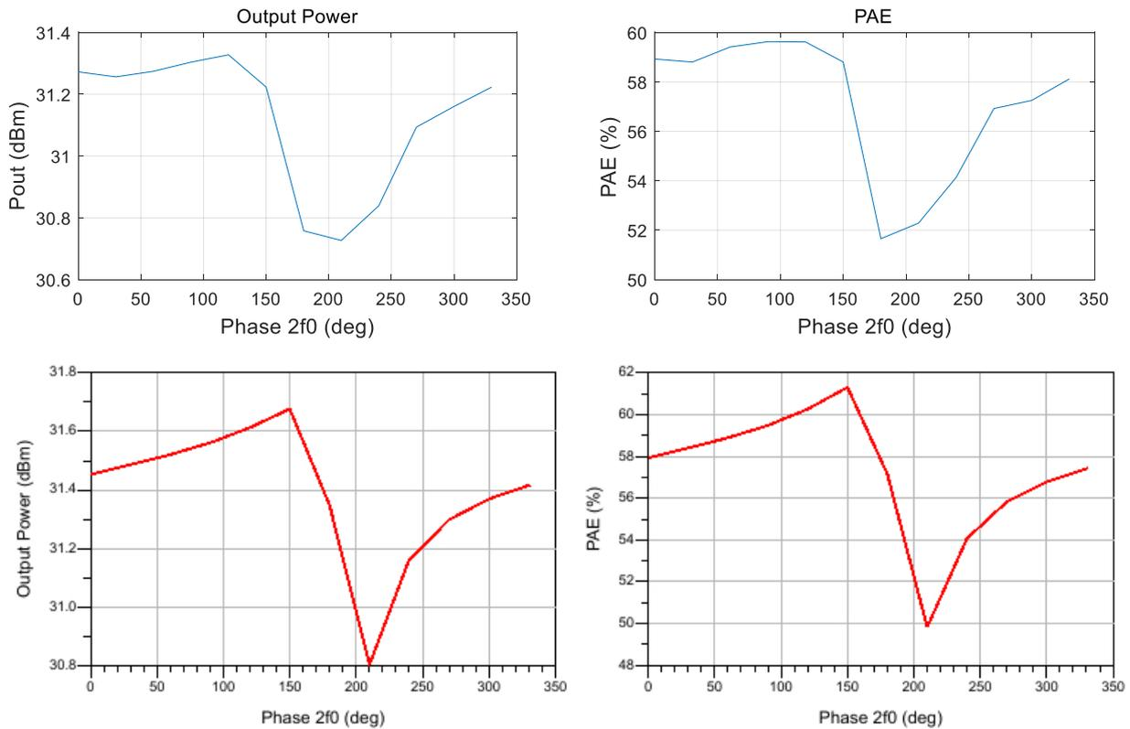
Figure 5-15 : Measured (top) and simulated (bottom) output power and PAE for the 8x50um transistor versus phase of the 2<sup>nd</sup> harmonic load (mag=1), at  $P_{avs}=27\text{dBm}$ ,  $V_d=20\text{V}$ ,  $V_g=-2.9\text{V}$ , 18.0 GHz,  $T_a=25^\circ\text{C}$ , fundamental load =  $-0.3 + j 0.6$ .
