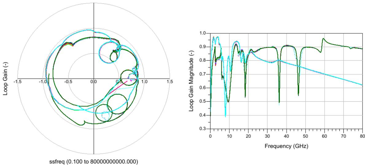
Figure 5-87 : Large signal loop gain analysis for a source power of 15 dBm at 17.3-20.3 GHz,  $V_g = -3.1V$ ,  $V_d = 20V$ ,  $T_a = 80degC$ , 50ohm output load.
