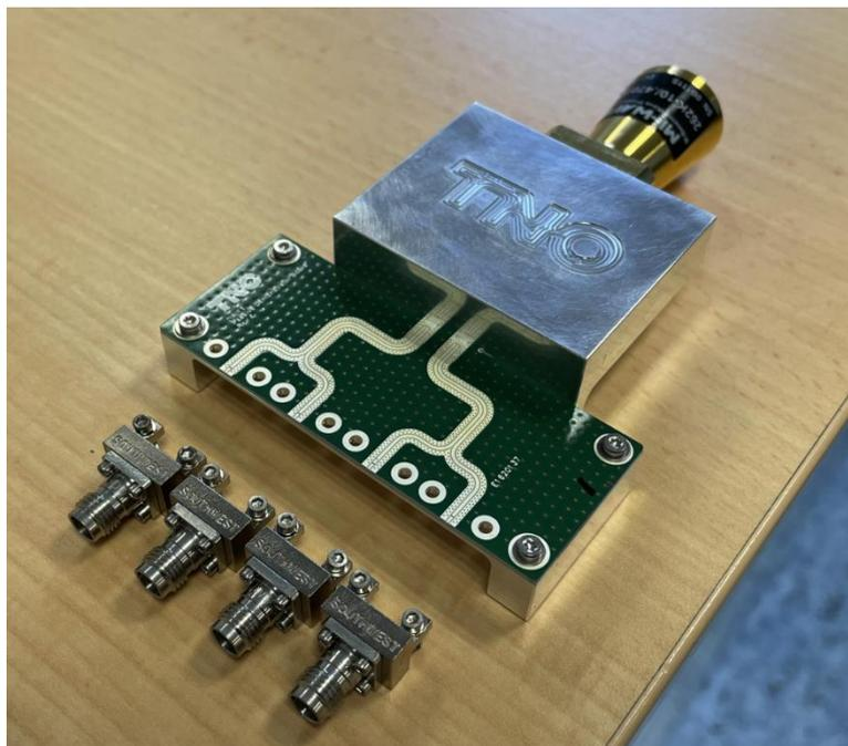
Figure 6-41 DRIFT assembled passive antenna demonstrator.
