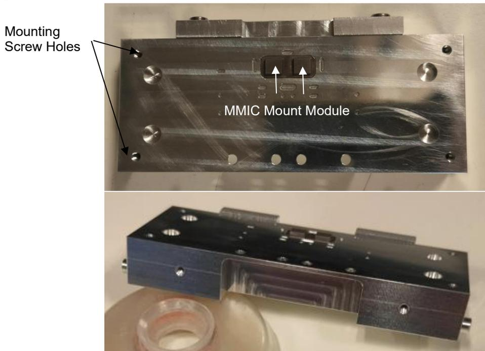
Figure 6-29 DRIFT PCB mounted structure with assembled MMIC mount module.
