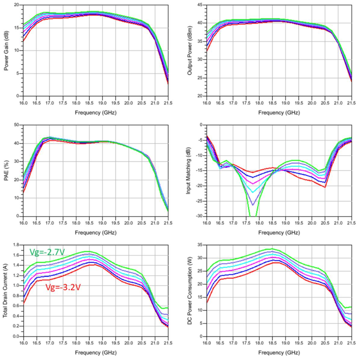
Figure 5-29 : Frequency sweeps at 23 dBm source power for  $V_g = -3.2$  to  $-2.7$  V.
