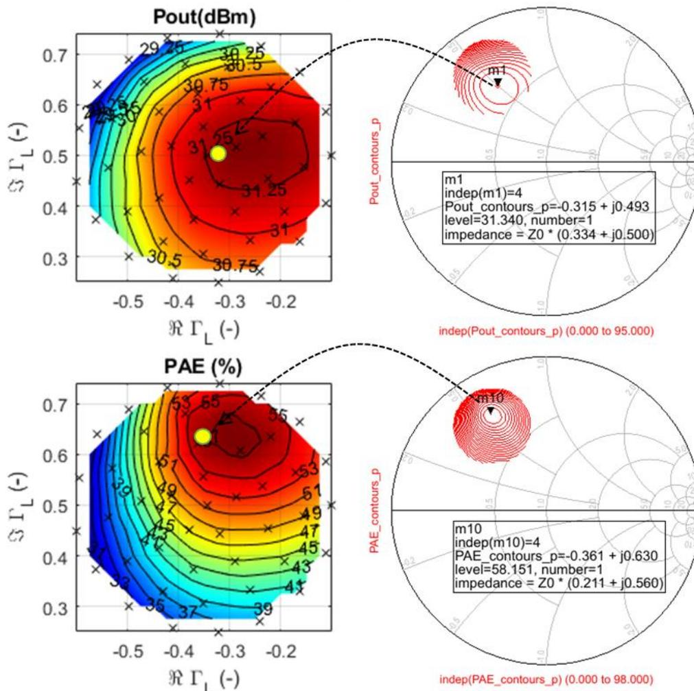
Figure 5-12 : Comparison of measured (left) and simulated (right) load pull contours for the 8x50um transistor, at  $V_d=20\text{V}$ ,  $V_g=-2.9\text{V}$ , 18.0 GHz,  $T_a=25^\circ\text{C}$ , without 2<sup>nd</sup> harmonic load optimization.
