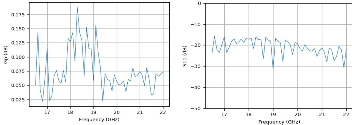
Figure 6-5 : Measured power gain and S11 of the THRU port 1 -> 2, with driver amp at 0dBm source power, directly after calibration, using the “actual waves” method.
