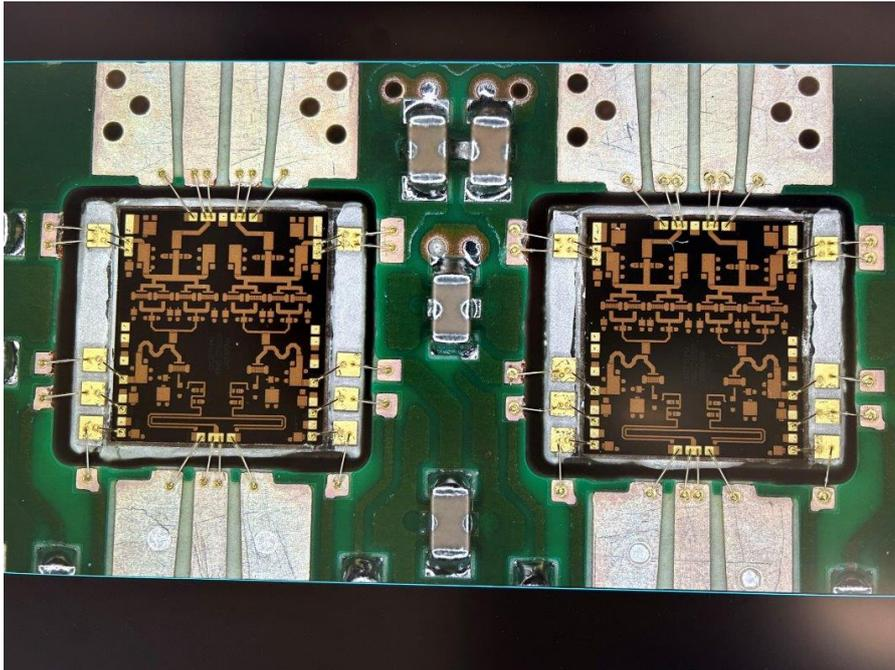
Figure 6-32 DRIFT MMIC and Die-Cap attach and wire bonding.
