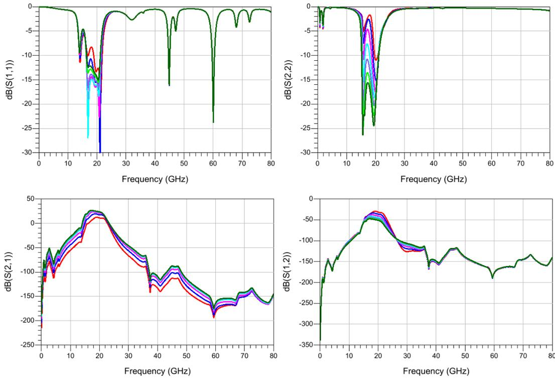
Figure 5-70 : Small-signal narrow- and wide-band S-parameters for the HPA, as function of gate bias voltage ( $V_g = -3.3$  to  $-2.7$ V).
