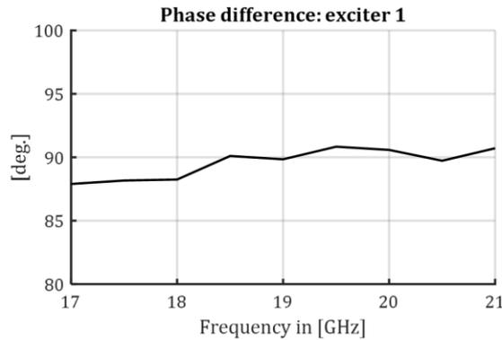
Figure 6-51: Phase difference measured across a more extended frequency range.
