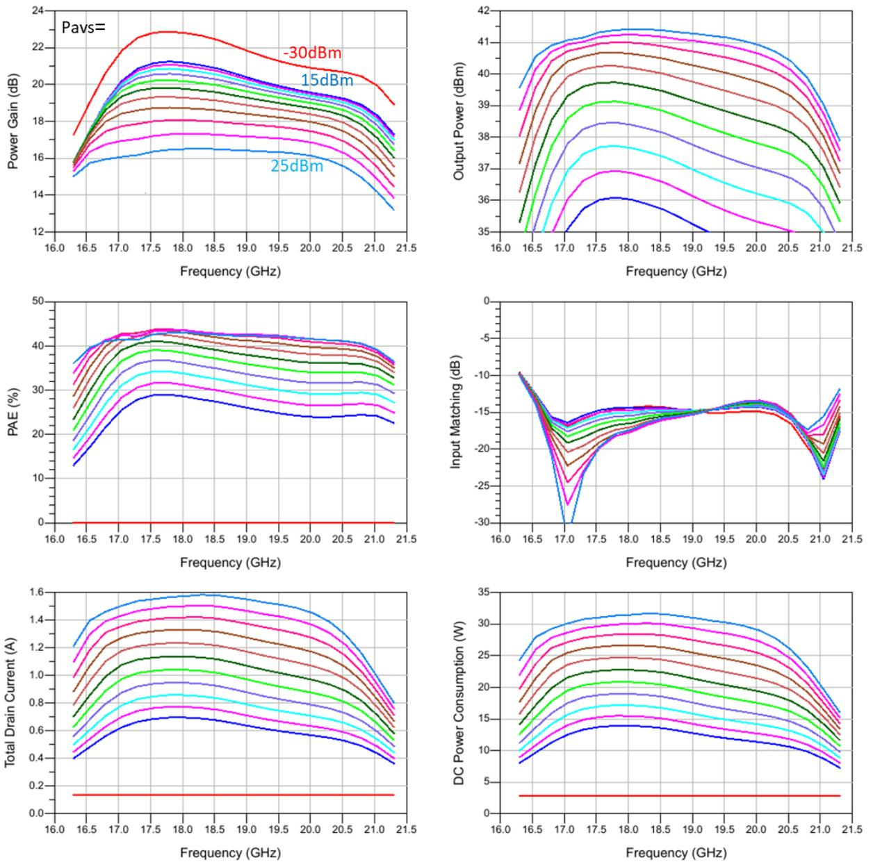
Figure 5-71 : Large-signal performance for  $P_{avs} = -30$  and  $15 - 25$  dBm,  $V_g = -3.1V$ ,  $V_d = 20V$ ,  $T_a = 80degC$ , using the dipole feed as load.
