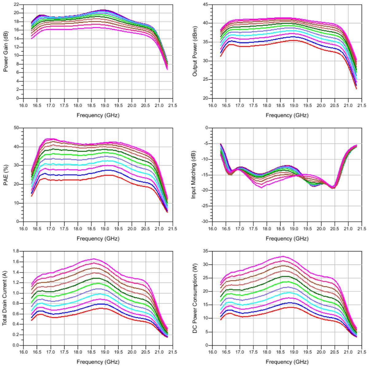
Figure 5-26 : Large-signal performance for  $P_{avs} = 15 - 25$  dBm.
