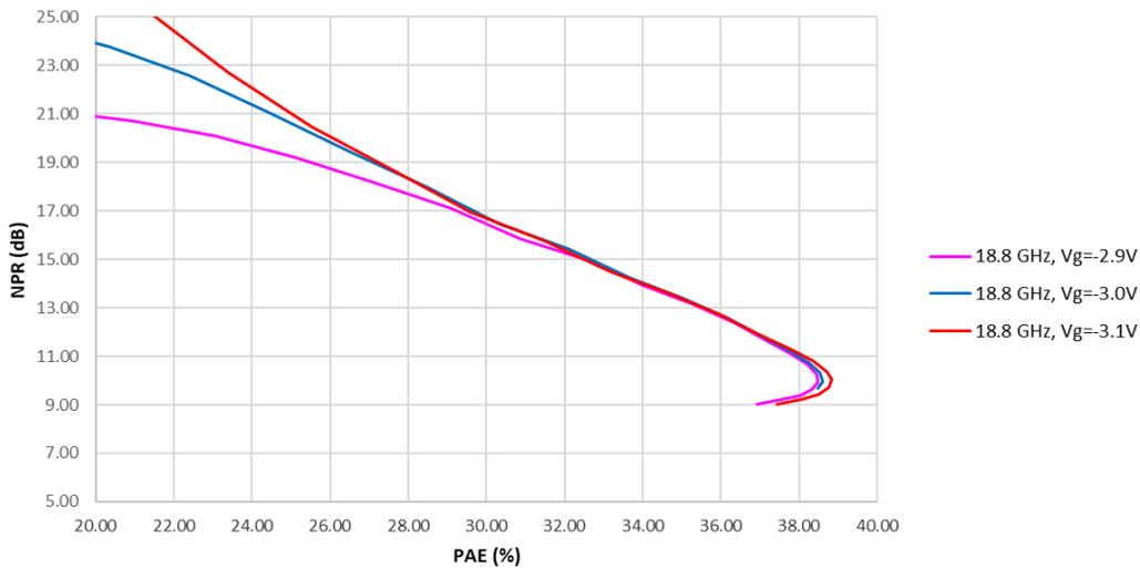
Figure 5-35 : IMAL calculation at 18.8 GHz,  $V_d=20V$ ,  $T_a=80^{\circ}C$ , for  $V_g=-3.1$  to  $-2.9$  V.
