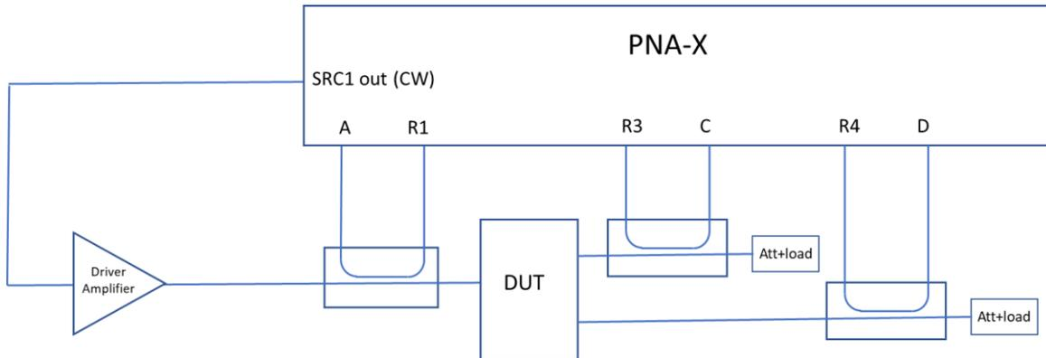
Figure 5-121 : Large-signal 3-port measurement setup.
