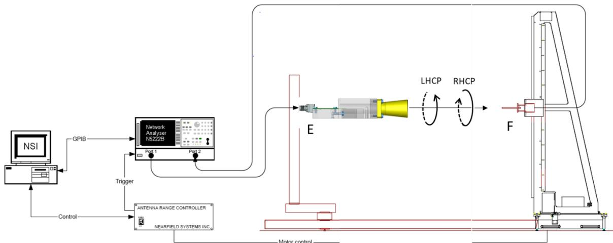
Figure 5-129 : Schematic of the polarisation test. Two lines run from the PNA-X to the receiving horn, however it is TBD whether a single or dual polarised horn will be used.
