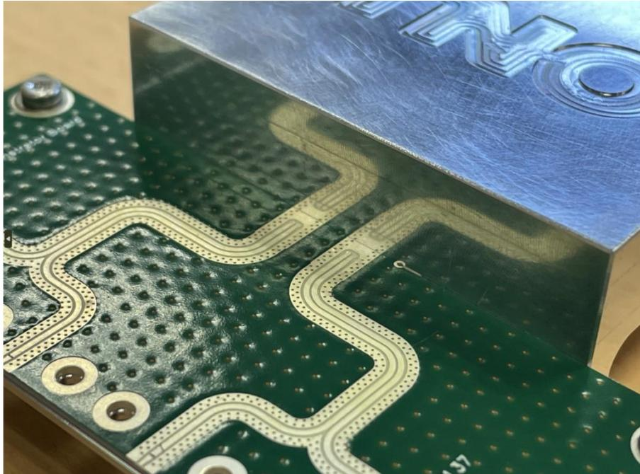
Figure 6-42 close up view of the waveguide exciters slotted into the waveguide.
