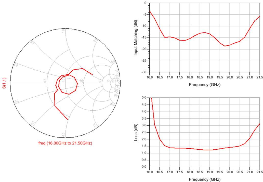
Figure 5-22 : Simulated performance of the initial input matching network, including the balun.
