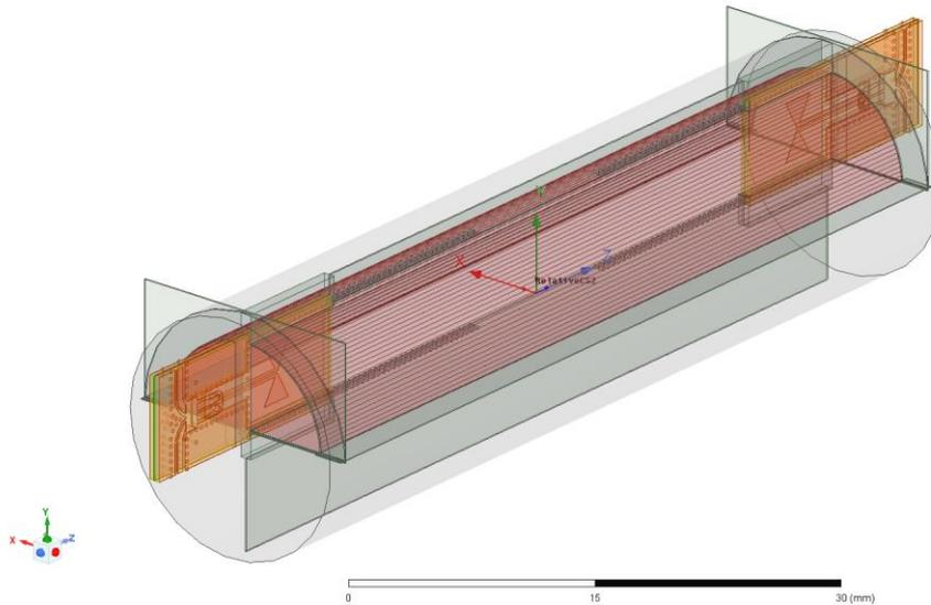
Figure 5-61: Model better representing the realised test assembly. The gaps as they are mentioned in the text are shown with a light green colour.
