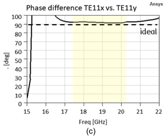
Figure 5-52: Septum polariser performance. (a) S-parameters: transmission to the fundamental orthogonal modes TE11x and TE11y (green solid and dashed), reflection (red) and cross-talk to other input (black). (b) Losses, reflection loss (red) and insertion loss (black). (c) Phase difference between the two orthogonal modes (solid black)
