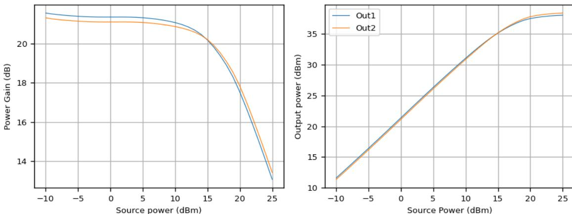
Figure 6-13 : Measured CW power sweep at 19 GHz showing the power gain and output for the two individual outputs, at the nominal gate bias at 20V, 25degC, sample R2C1
