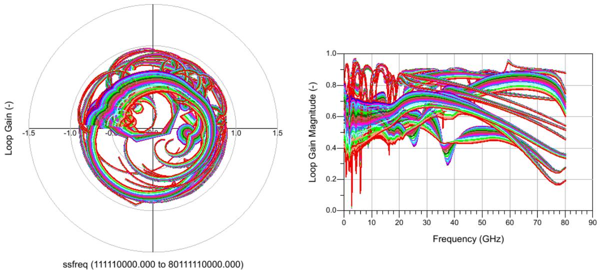
Figure 5-88 : Loop gain analysis for a source power range of +10 to +25 dBm at 18.8 GHz,  $V_g = -3.1V$ ,  $V_d = 20V$ ,  $T_a = 25degC$ , 50ohm output load, showing all 20 loops.
