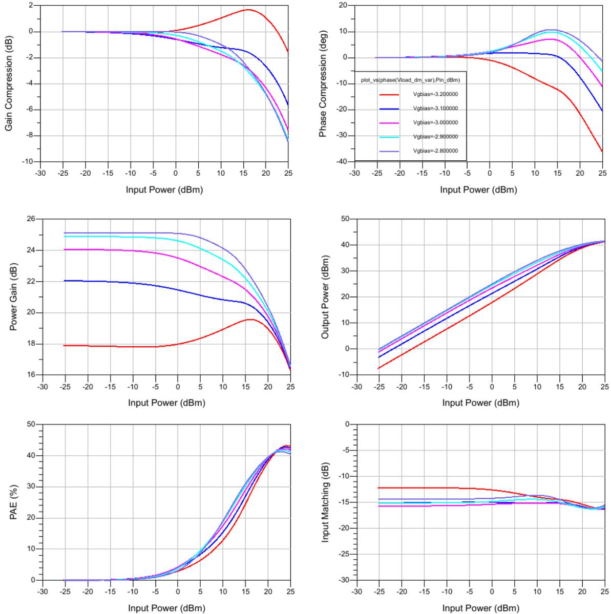
Figure 5-73 : Power sweeps at 18.8 GHz for Vg = -3.2 to -2.8 V, Vd=20V, Ta=80degC.
