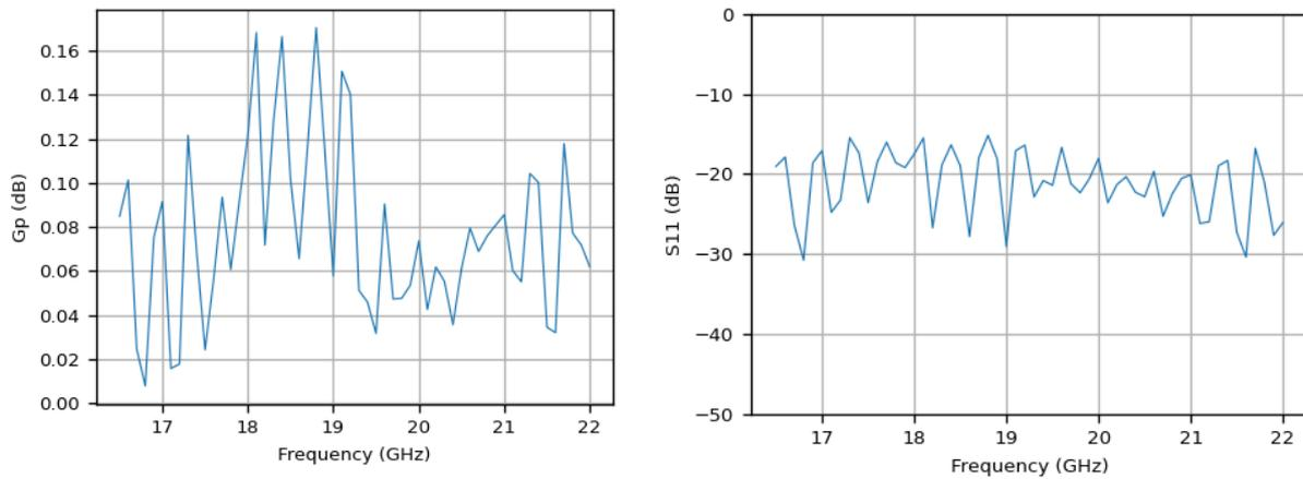
Figure 6-4 : Measured power gain and S11 of the THRU port 1 -> 2, without driver amp at -10dBm source power, directly after calibration, using the “actual waves” method.
