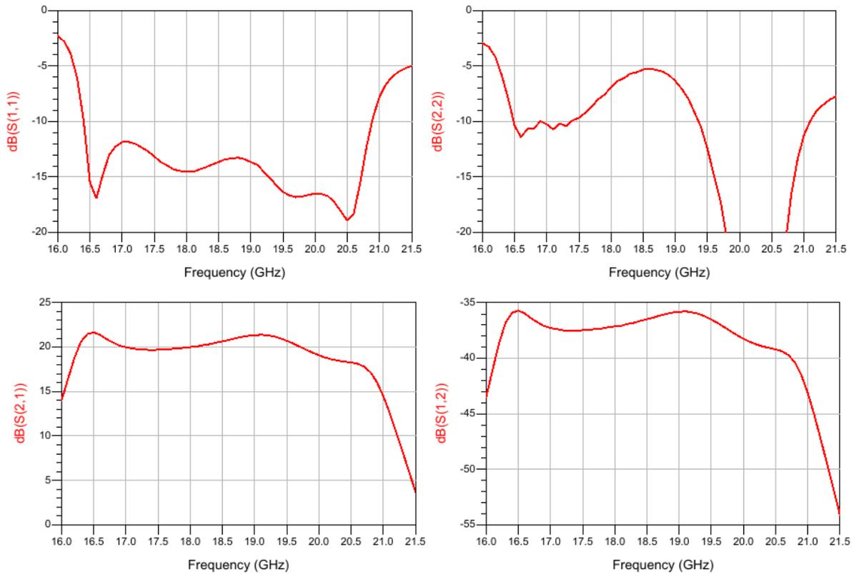
Figure 5-24 : Small-signal S-parameters for the HPA including the waveguide feed.
