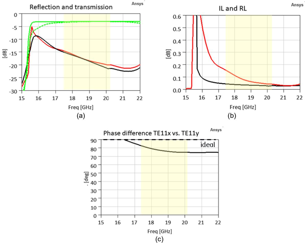
Figure 5-50: Septum polariser performance. (a) S-parameters: transmission to the fundamental orthogonal modes TE11x and TE11y (green solid and dashed), reflection (red) and cross-talk to other input (black). (b) Losses, reflection loss (red) and insertion loss (black). (c) Phase difference between the two orthogonal modes (solid black).
