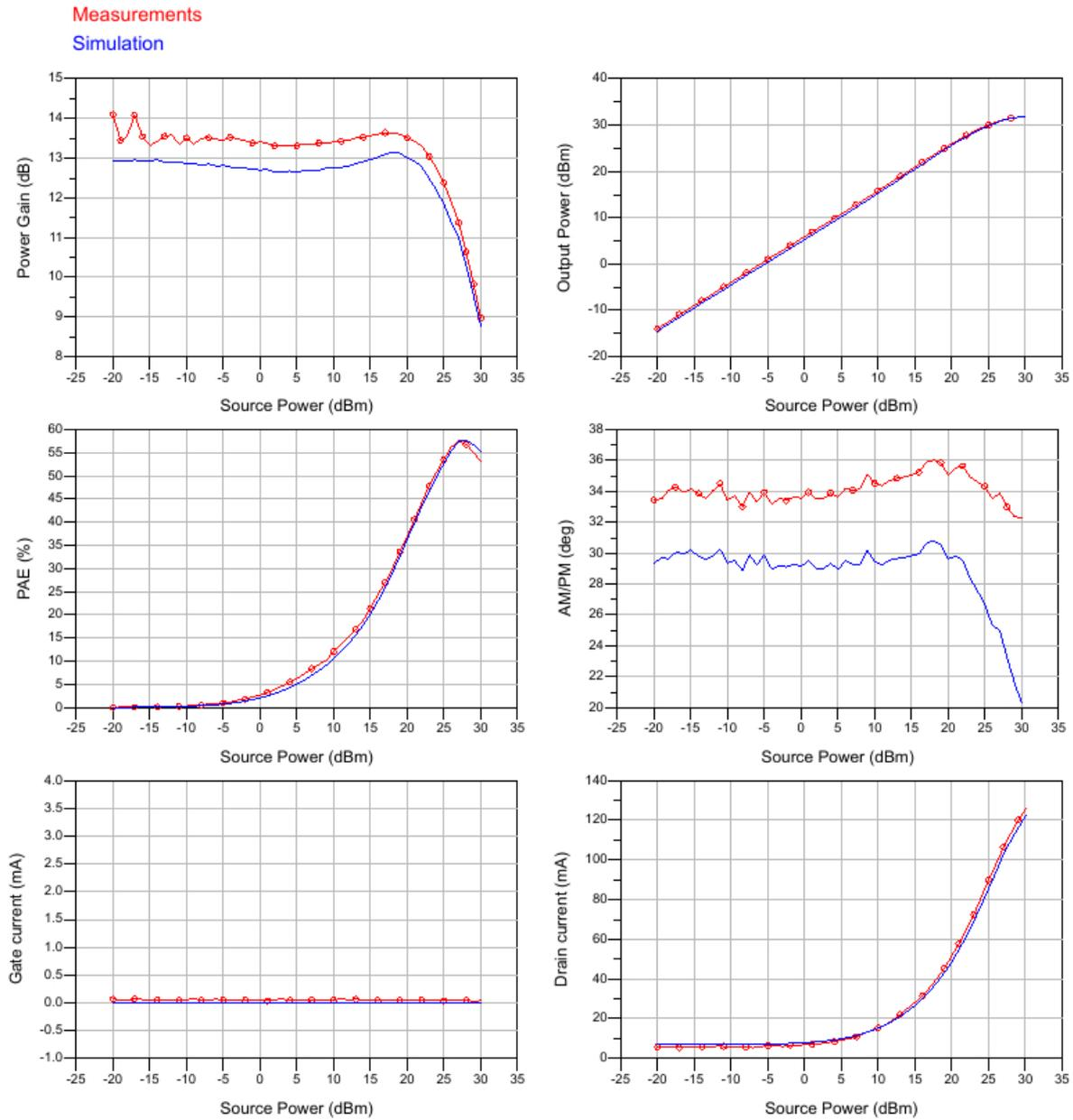
Figure 5-13 : Comparison of measured and simulated power sweep for the 8x50um transistor, at  $V_d=20V$ ,  $V_g=-2.9V$ , 18.0 GHz,  $T_a=25^\circ C$ , fundamental load =  $-0.3 + j 0.6$ , without 2<sup>nd</sup> harmonic load optimization.
