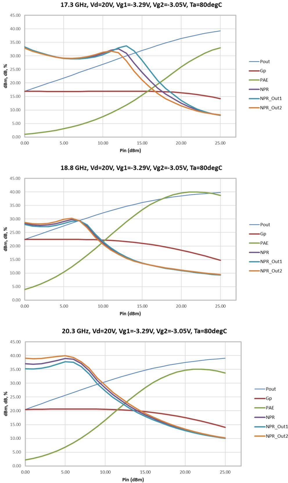
Figure 6-25 : IMAL calculations based on power sweep measurements at 3 frequencies.
