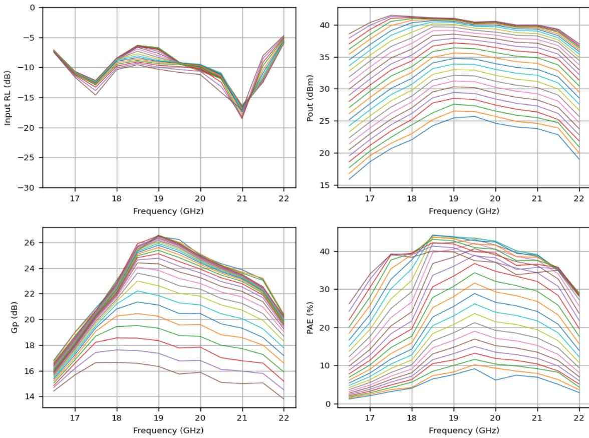
Figure 6-12 Measured CW power-frequency sweep for a source power of 0-25 dBm (1dB step), at the nominal gate bias at 20V, 25degC, sample R2C1.
