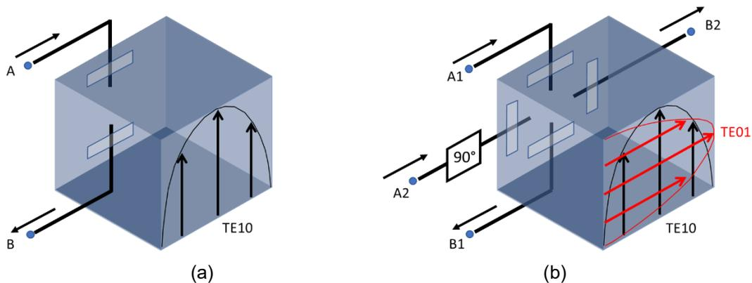
Figure 5-6: Feeding scheme of square waveguide supporting dual circular polarisation. (a) Differentially fed resulting in linear polarisation and (b) Differentially fed resulting in circular polarisation (only one polarisation sense shown). Amplifier output lines connect to parallel slots.
