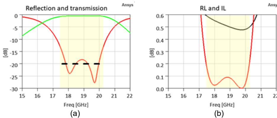
Figure 5-47 : (a) Reflection and transmission case patch exciter, and (b) losses RL (red), IL (black).
