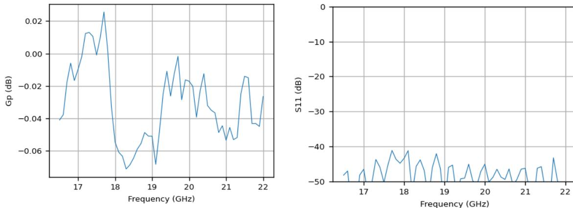
Figure 6-3 : Measured power gain and S11 of the THRU port 1 -> 2, without driver amp at -10dBm source power, directly after calibration, using the “match corrected” method.
