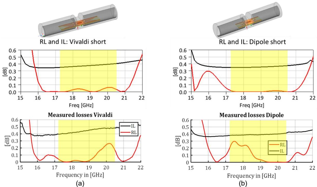
Figure 5-100: Comparison of the simulated and measured insertion loss in case of: (a) Vivaldi exciters, and (b) Dipole exciters.
