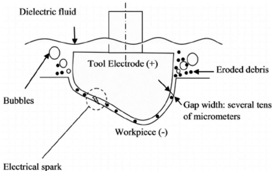
Figure 5-93: Concept of sink-sparking, schematic display
