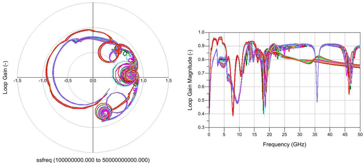
Figure 5-91 : Loop gain analysis for a source power range of -25 to +25 dBm at 18.8 GHz,  $V_g = -3.1V$ ,  $V_d = 20V$ ,  $T_a = 25degC$ , source impedance sweep magnitude 0.33, 0.66 and 0.99 with phase from 0-360deg, showing the loops at the gates of the input and output stage.
