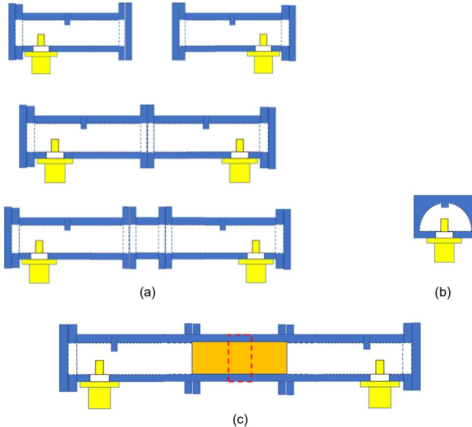
Figure 5-125: (a) Calibration standards based on semi-circular wave guides, from top to bottom: reflect, through and line. (b) Frontal view of the semi-circular wave guide including a tuning stub. (c) Anticipated test setup with the coax-to-semi-circular wave guide transitions in place and the test structure in between. The orange part represents a PCB and the red dashed box indicates the position in the centre where the parallel line is connected to free space.
