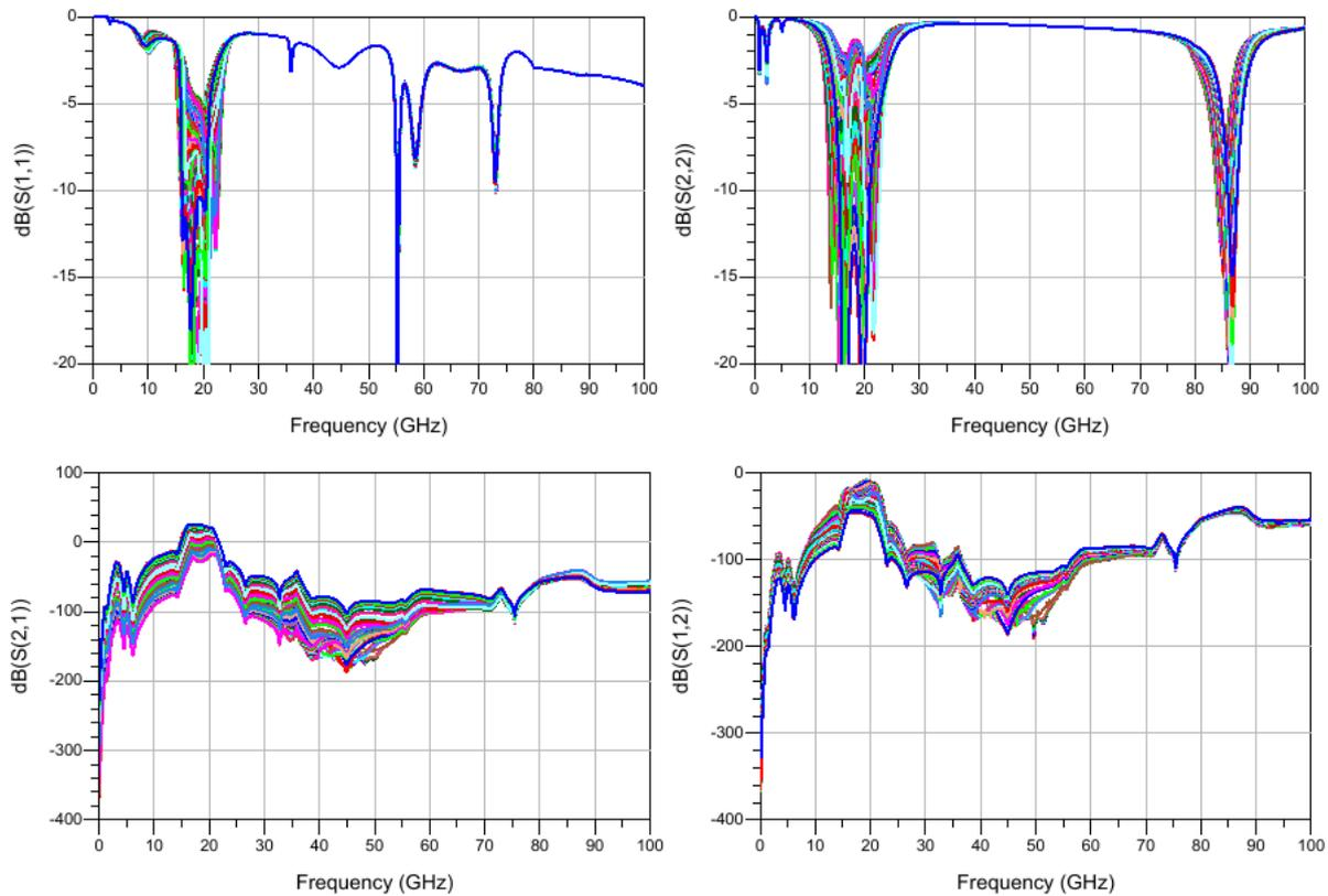
Figure 5-36 : S-parameters for  $V_d = 2$  to  $20$  V and  $V_g = -5$  to  $-2$  V.
