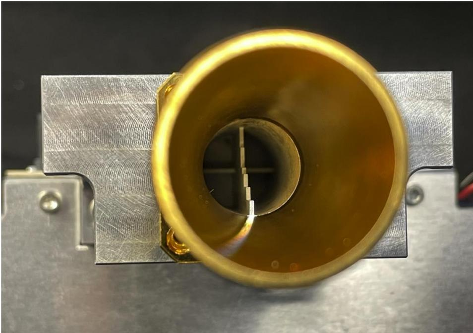
Figure 6-37 DRIFT waveguide front view looking into the waveguide and septum.
