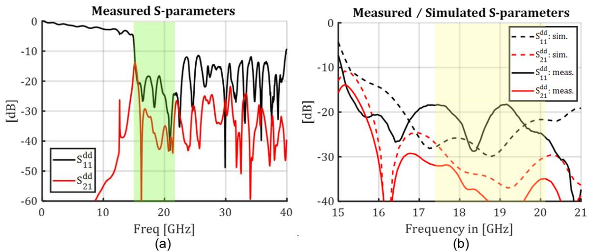
Figure 6-44: Measured reflection seen at a single differential input port and cross-talk between the two input ports. (a) Full band results with the green shade indicating the frequency band of interest, and (b) zooming in on that spectral range.
