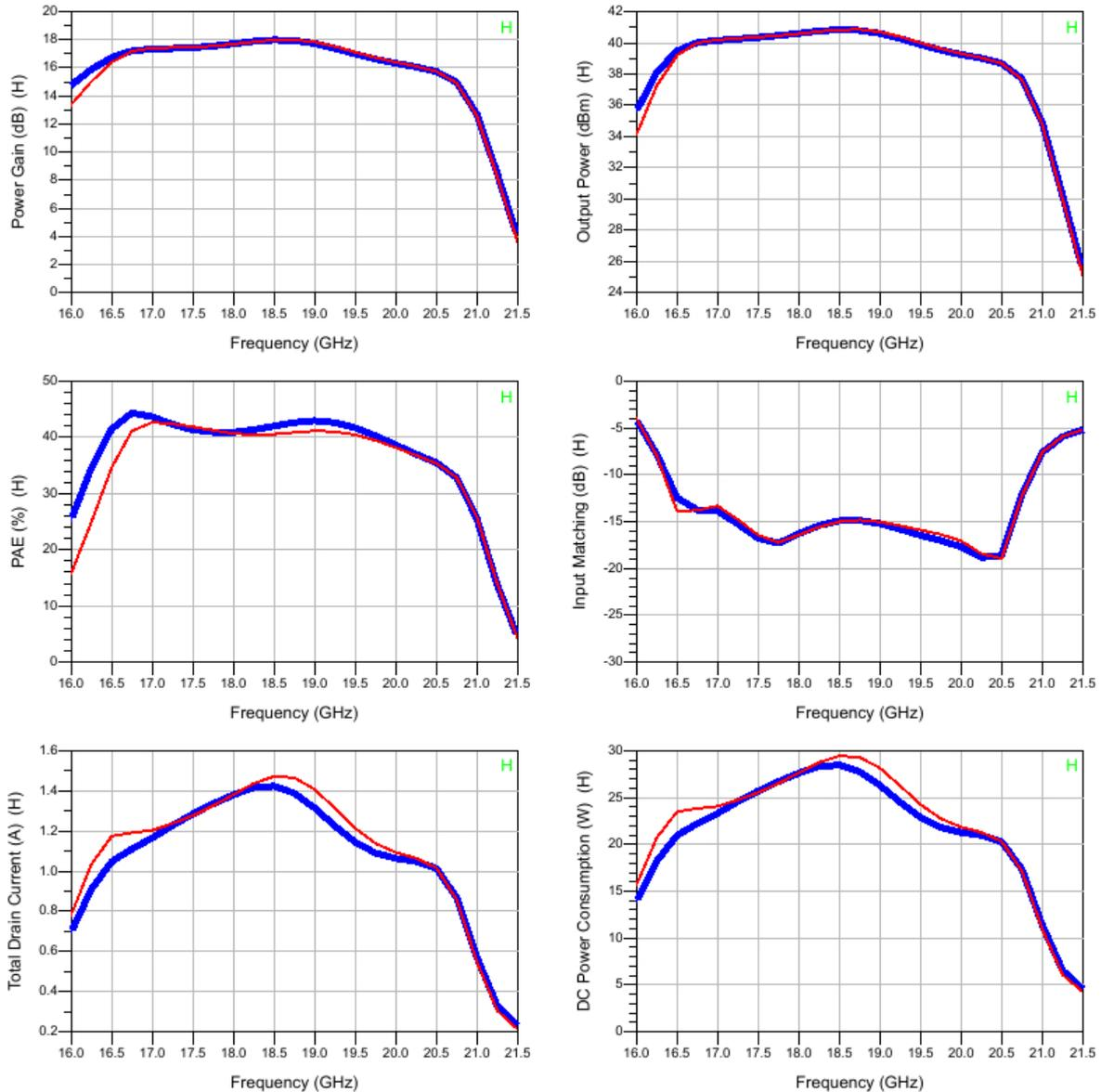
Figure 5-31 : Difference between the actual differential feed load (red) and an ideal 50ohm load (blue), at 23 dBm source power.
