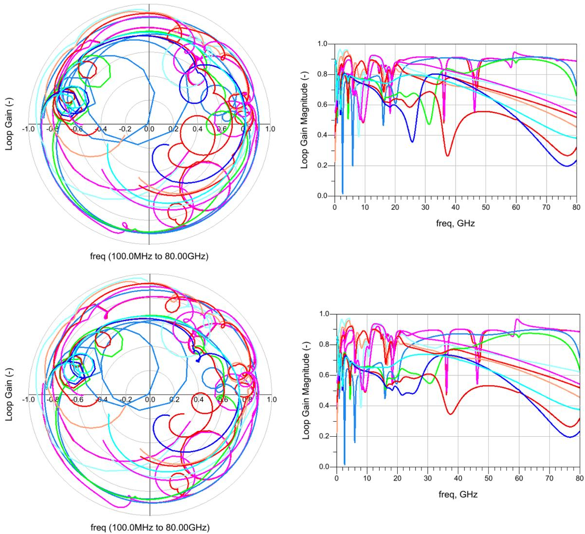
Figure 5-84 : Small signal loop gain simulation for the nominal operation at  $V_g = -3.1\text{V}$ ,  $V_d = 20\text{V}$  for  $T_a = 20\text{degC}$  (top) and  $T_a = 80\text{degC}$  (bottom), with the HPA loaded by  $50\text{ohm}$ .
