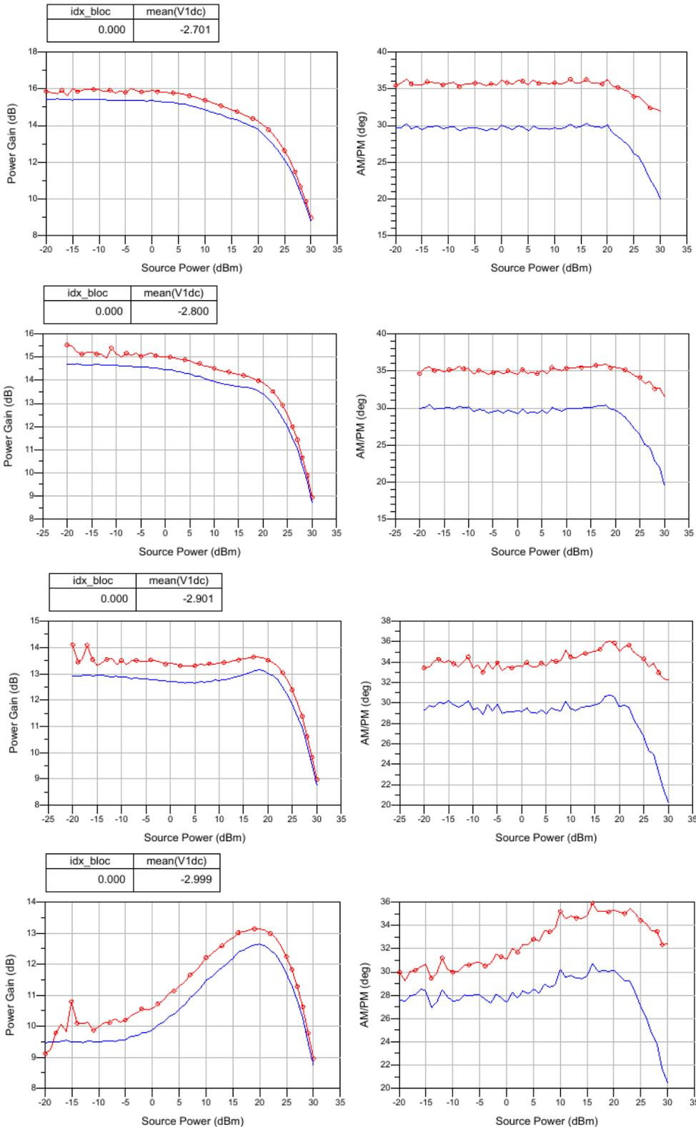
Figure 5-14 : Comparison of measured and simulated power sweep, showing the gain and phase compression for the 8x50um transistor versus  $V_g$ , at  $V_d=20V$ , 18.0 GHz,  $T_a=25^\circ C$ , fundamental load =  $-0.3 + j 0.6$ , without 2<sup>nd</sup> harmonic load optimization.
