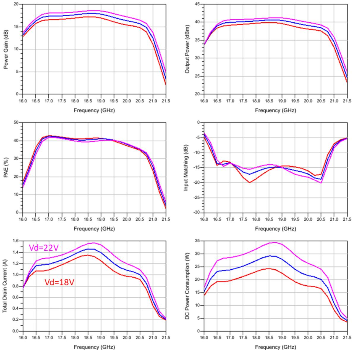
Figure 5-30 : Frequency sweeps at 23 dBm source power for Vd = 18, 20 and 22 V.
