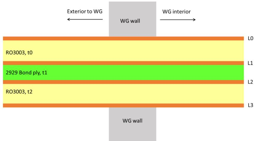
Figure 5-42: Layer stack definition for the waveguide feeder concepts. (a) L0 and L3 are closed copper GND planes connecting to the waveguide wall.
