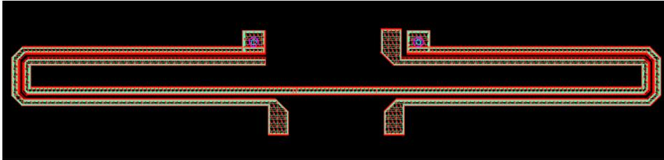
Figure 5-16 : Basic layout of the folded Marchand balun, line width 24µm, spacing 10µm, total height is 2 mm.
