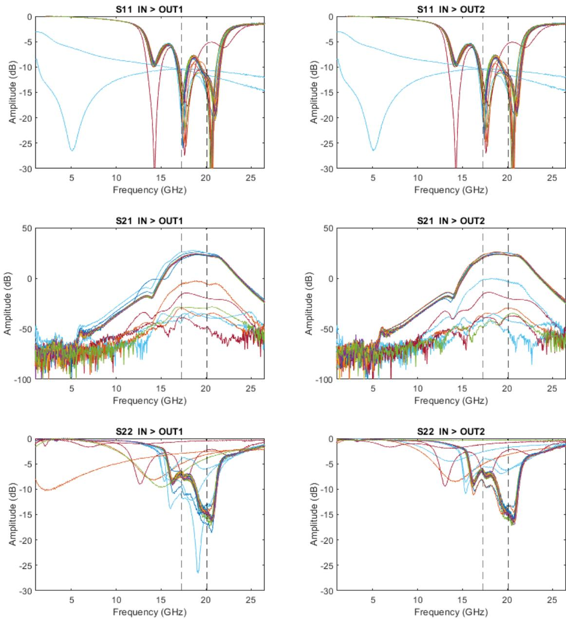
Figure 6-6 On-wafer S-parameter measurement data for all samples on the wafer.
