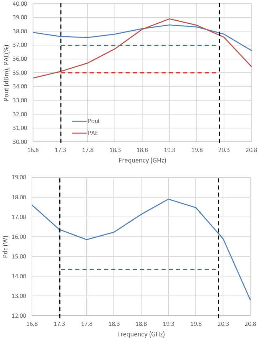
Figure 5-82 : Output power, efficiency and DC power consumption, calculated by IMAL for the 15 dB NPR point at  $V_g = -3.0V$ ,  $V_d = 20V$ ,  $T_a = 20degC$ .
