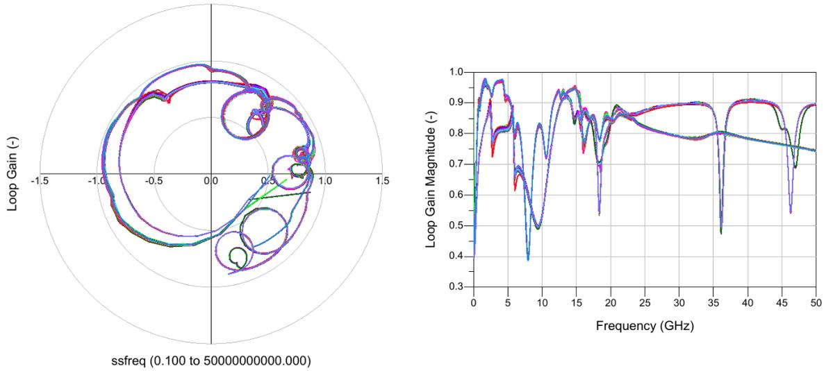
Figure 5-86 : Large signal loop gain analysis for a source power of 15 dBm at 16-21.5 GHz,  $V_g = -3.1V$ ,  $V_d = 20V$ ,  $T_a = 80degC$ , waveguide feed output load.
