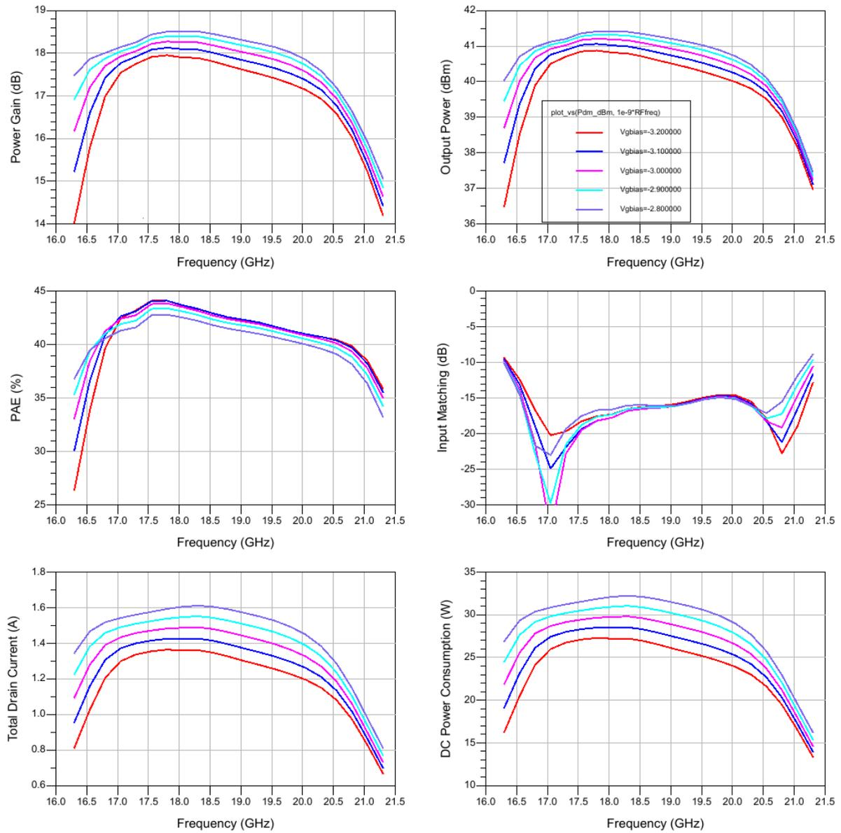
Figure 5-74 : Frequency sweeps at 23 dBm source power for  $V_g = -3.2$  to  $-2.8$  V,  $V_d=20$  V,  $T_a=80$ degC.
