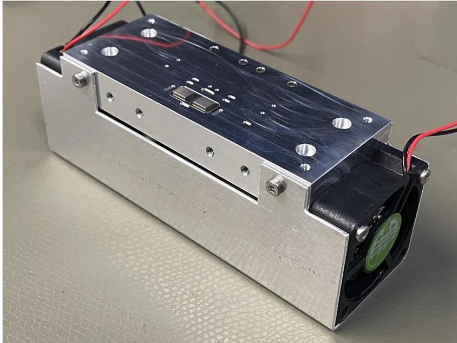
*Figure 6-30 Fully assembly PCB mounted structure with MMIC mount module and heatsink housing, fans and heatsink.*
