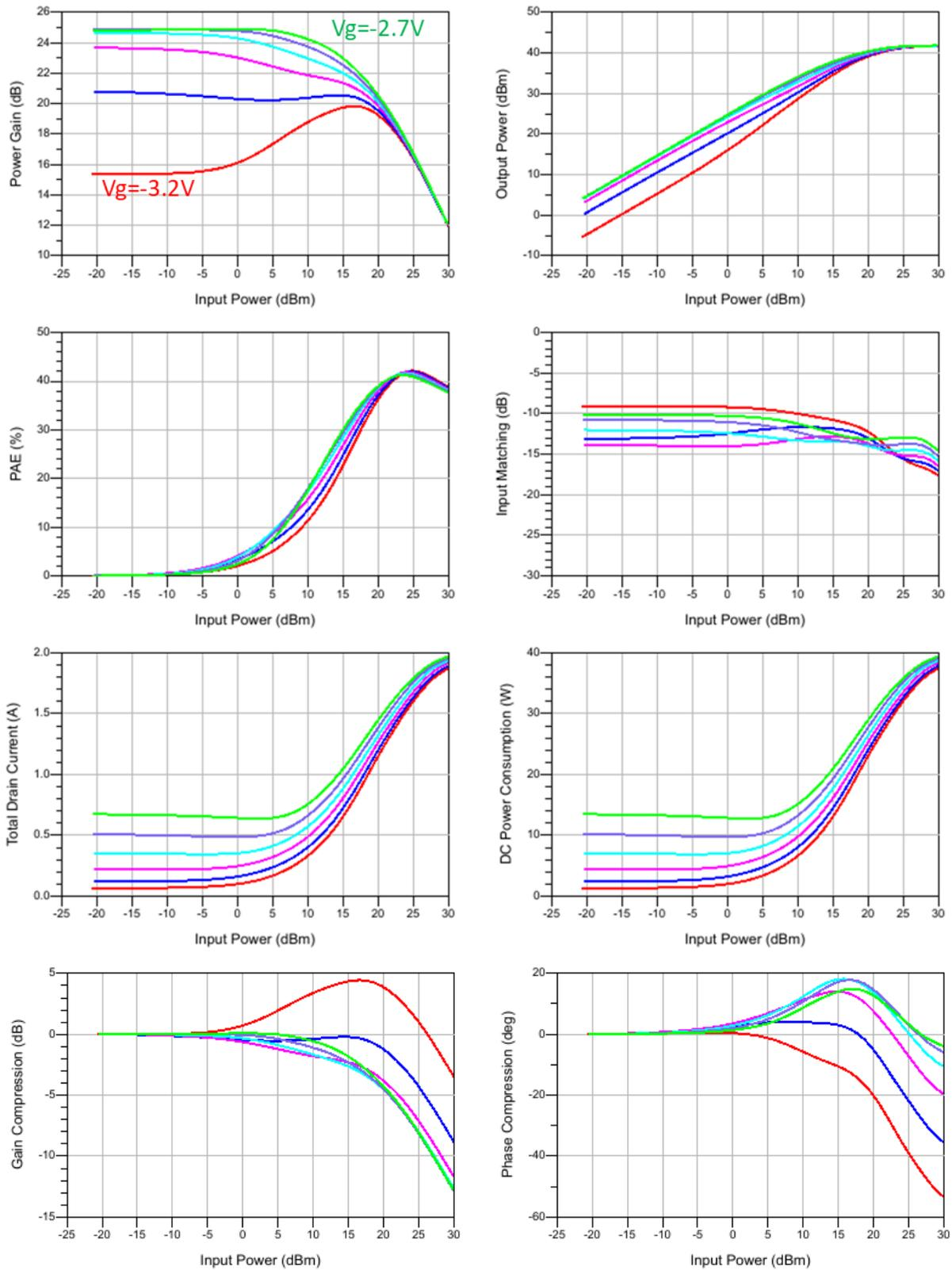
Figure 5-28 : Power sweeps at 18.8 GHz for  $V_g = -3.2$  to  $-2.7$  V.
