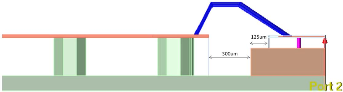
Figure 5-67 : Cross section of the 3D model of the input bondwire transition.
