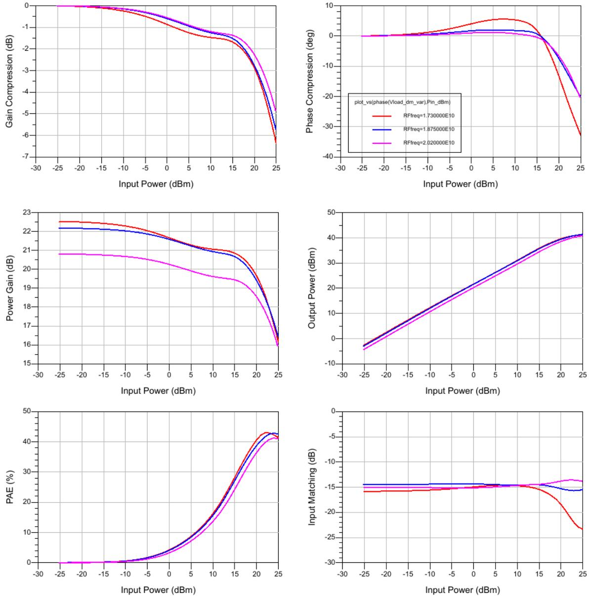
Figure 5-72 : Large-signal power-sweep at 17.3 GHz, 18.75 GHz and 20.2 GHz,  $V_g = -3.1V$ ,  $V_d = 20V$ ,  $T_a = 80degC$ .
