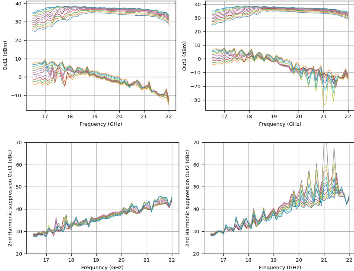
Figure 6-19 : CW power-frequency sweep for a source power of 15-25 dBm (1 dB step), at the nominal quiescent bias current of 140 mA and 20V, 25degC, sample R2C1, showing the fundamental and 2<sup>nd</sup> harmonic of the 2 outputs.
