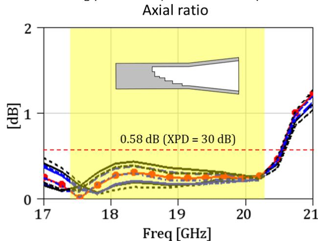
Figure 5-104: Axial ratio of the passive radiating front-end taking into account spark-erosion tolerance. Step sizes have been varied using a single factor to work on all step heights and a single factor to work on all step lengths. Nominal performance is represented by the red solid line with red circles.
