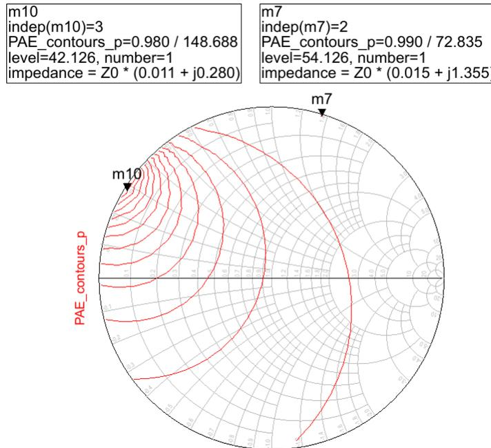
Figure 5-19 : Impact of the 2<sup>nd</sup> harmonic load impedance of the PAE.
