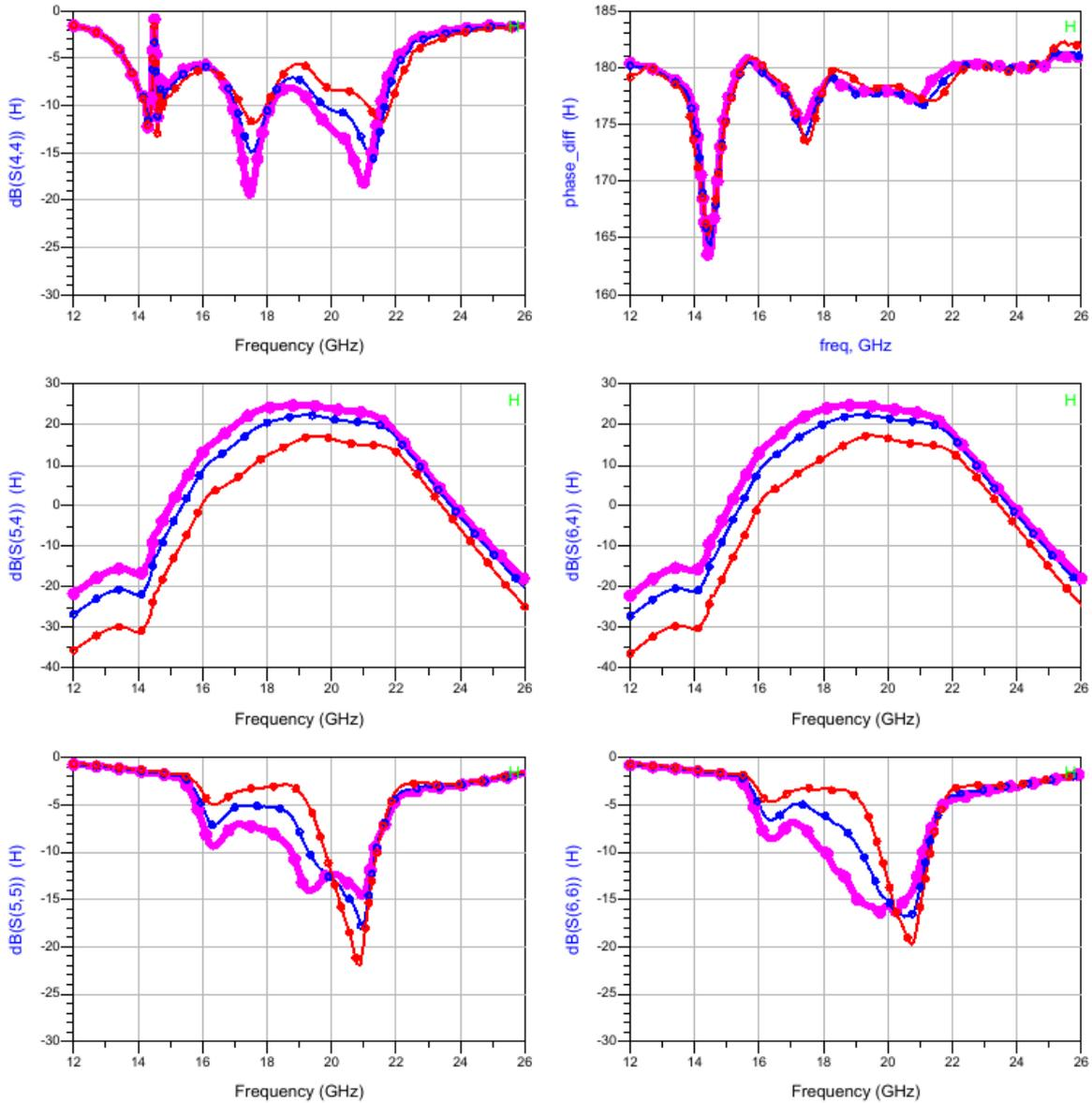
Figure 6-10 S-parameter measurements on sample R2C2 at  $V_d=20\text{V}$  and the nominal gate bias and +/-0.1V gate voltage variation,  $T_a=25\text{degC}$ .
