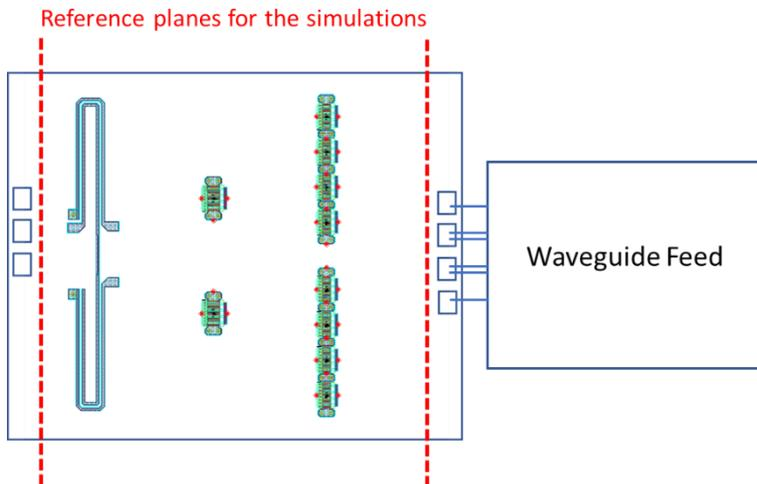
Figure 5-23 : Reference planes for the simulated HPA performance.
