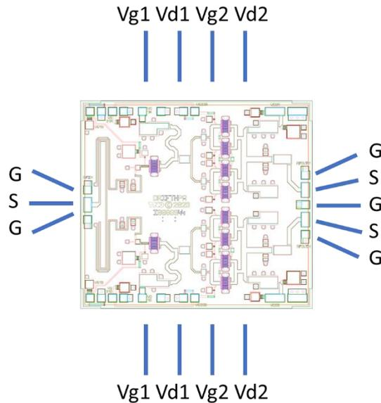
Figure 5-123 : On-chip probing.
