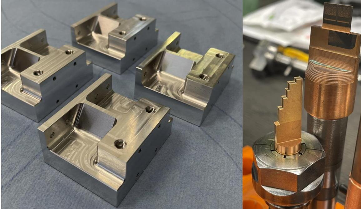
Figure 6-34 DRIFT waveguide initial structures (left), and tooling structures (electrodes) (right) to erode the septum and waveguide exciter from the initial structures.
