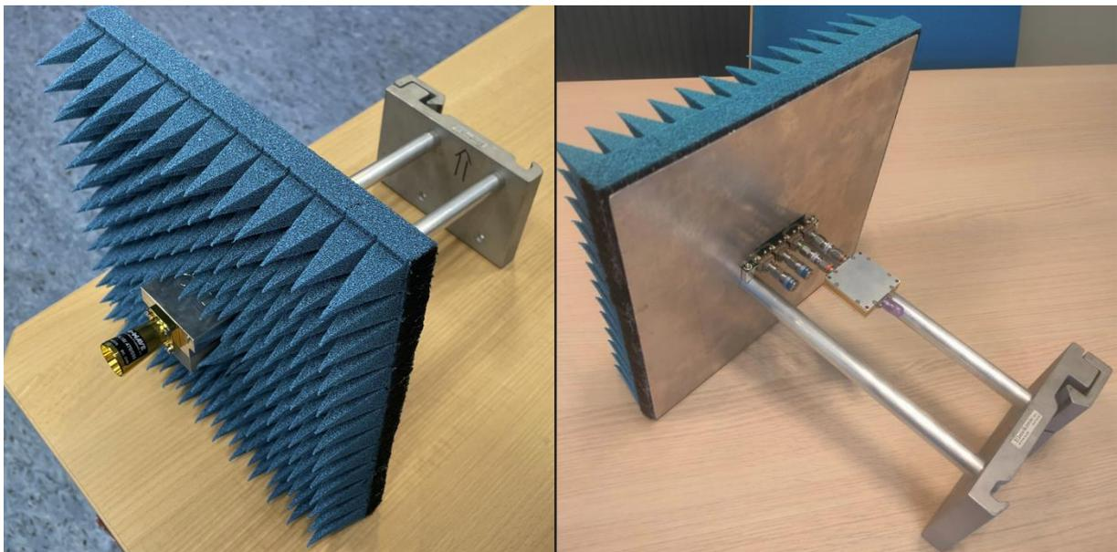
Figure 6-43 DRIFT fully assembled passive antenna demonstrator.
