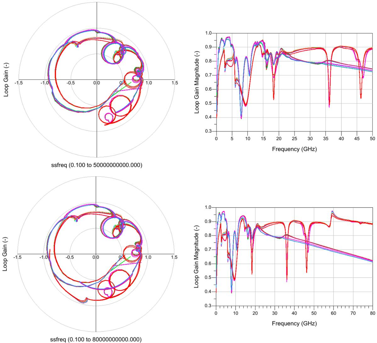
Figure 5-85 : Large signal loop gain analysis for a source power range of -25 to +25 dBm at 18.8 GHz,  $V_g = -3.1V$ ,  $V_d = 20V$ ,  $T_a = 80degC$ , waveguide feed output load (top) and 50 ohm load (bottom).
