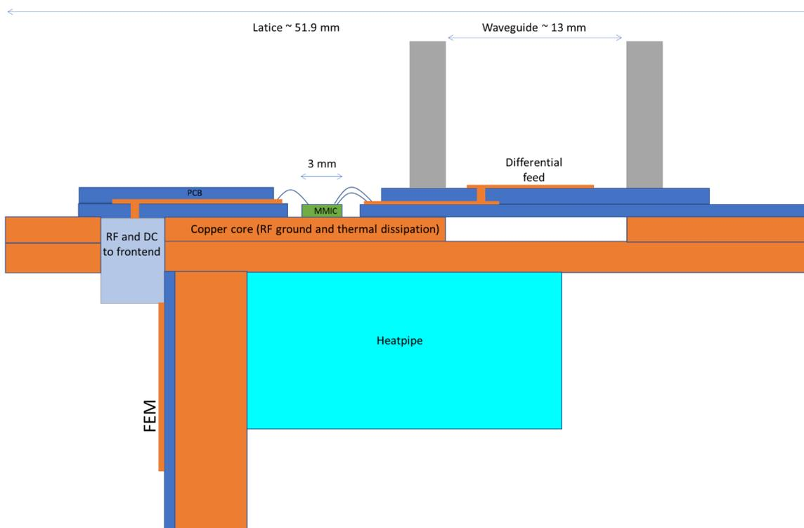
Figure 5-8 : Cross-section example for the case of a planar waveguide feed (hybrid architecture), with the MMIC and waveguide both on the top side of the PCB, showing only 1 polarisation (not fully to scale).
