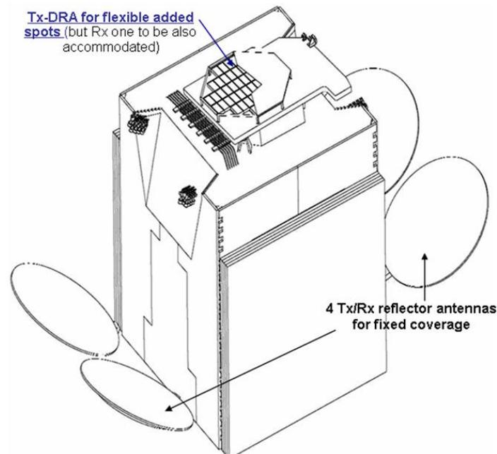
Figure 5-1: Example of combining 4 'SFB' reflector antennas on East-West walls, and a DRA on Earth panel
