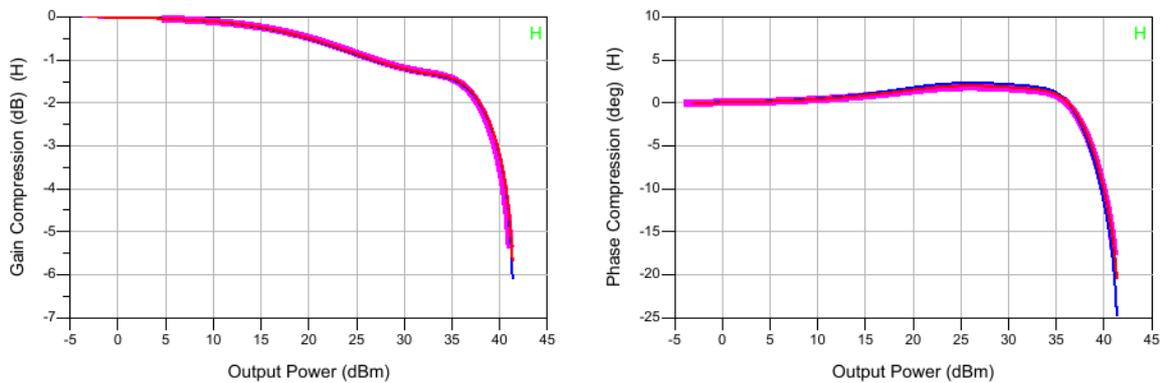
Figure 5-77 : Power sweep at 18.8 GHz with +/- 9% MIM capacitor variation,  $V_g=-3.1$  V,  $V_d=20$  V,  $T_a=80$ degC.
