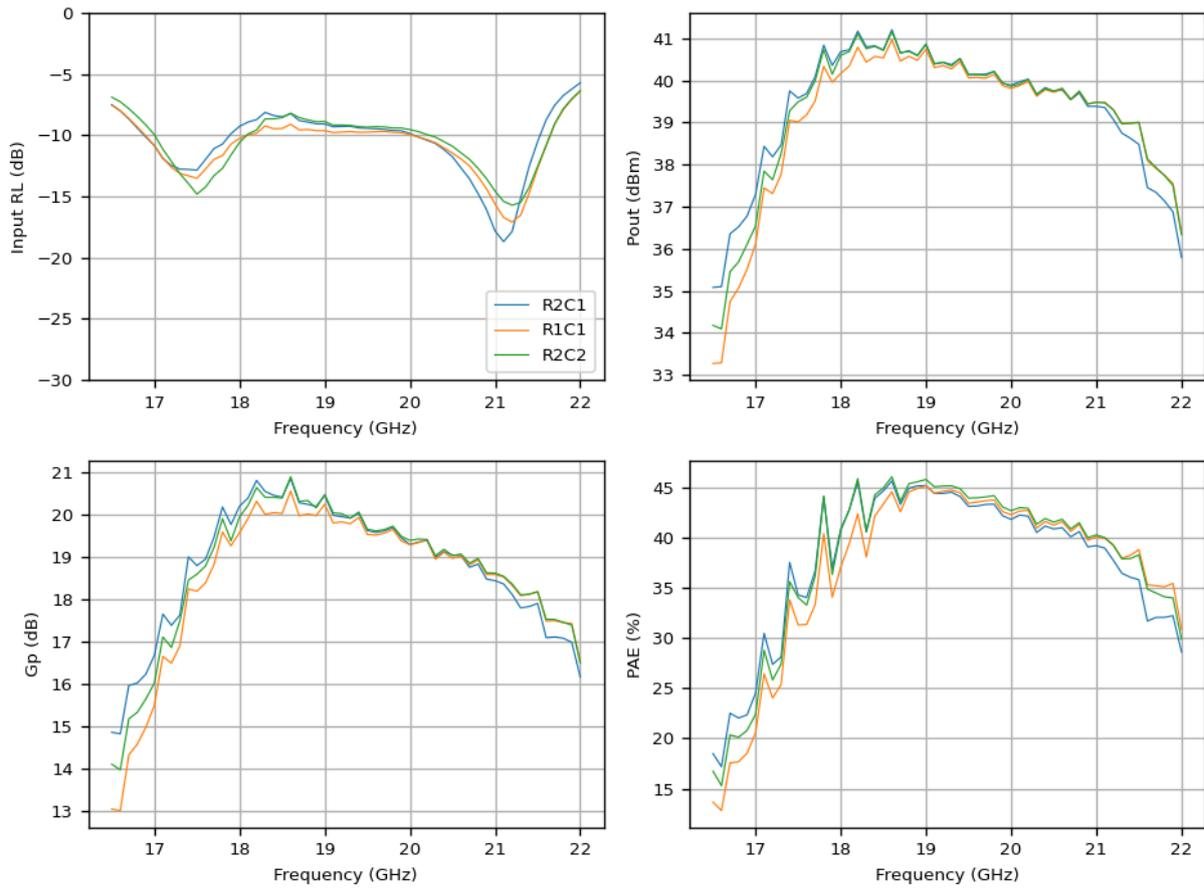
Figure 6-16 : Frequency sweep for all samples at a source power of 21 dBm, at the nominal quiescent bias current of 140 mA and 20V, 25degC.
