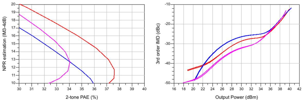
Figure 5-33 : Estimated NPR-PAE performance and IM3 at 17.3 GHz (red), 18.8 GHz (blue) and 20.3 GHz (magenta).
