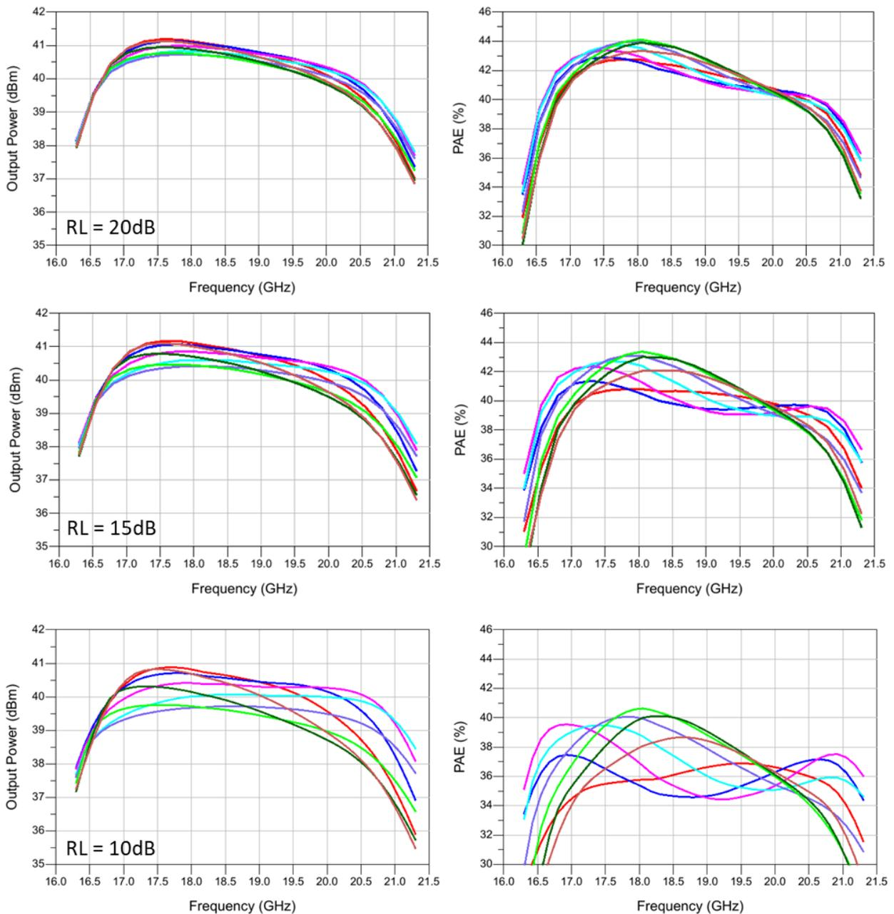
Figure 5-79 : Impact of 20, 15 and 10 dB return loss (with varying phase) at 23 dBm source power,  $V_g = -3.1V$ ,  $V_d = 20V$ ,  $T_a = 80degC$ .
