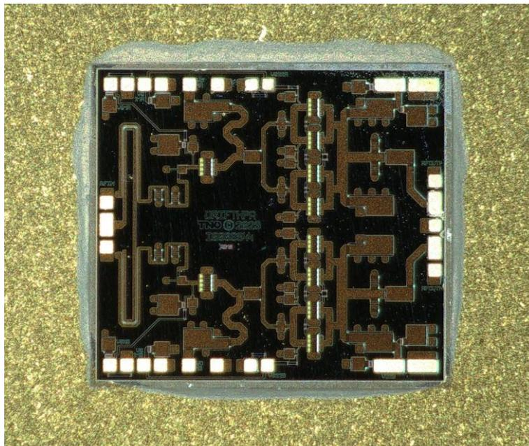
Figure 6-2 : MMIC mounted with silver sintering on CuMo carrier.
