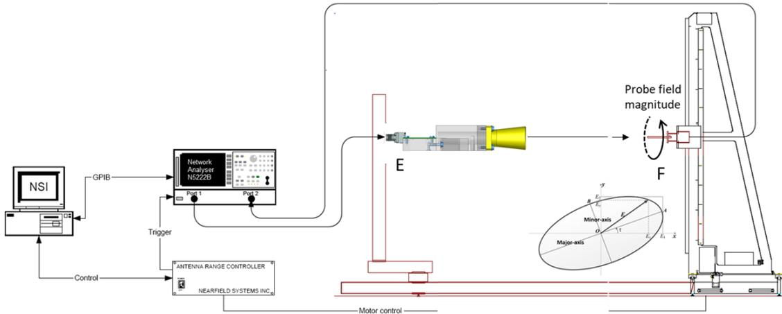
Figure 6-47: Passive radiating frontend for validating the AR performance schematically shown in a near-field test setup.
