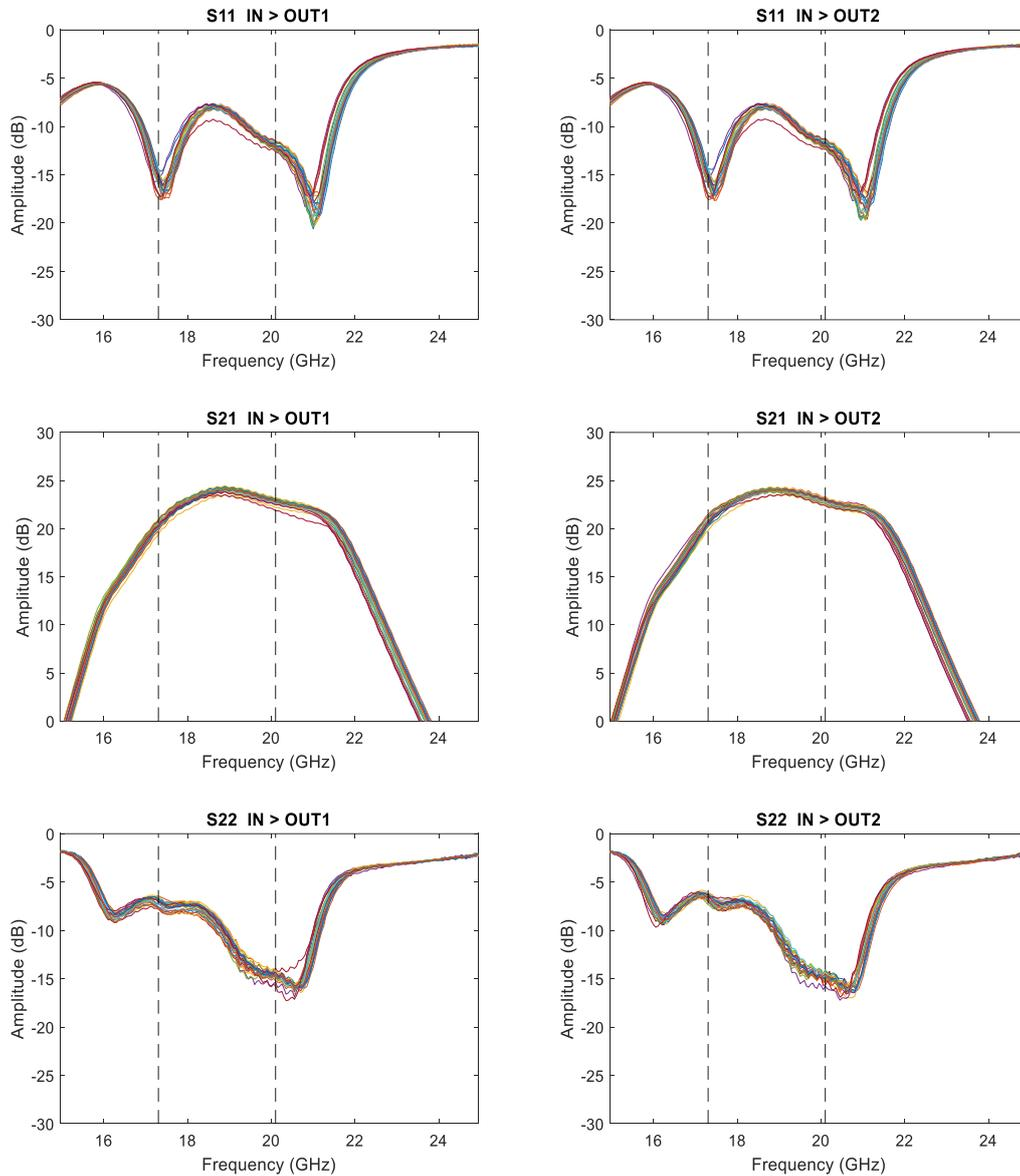
Figure 6-7 : On-wafer S-parameter measurement data for the functional samples on the wafer with 2 additional outliers removed.
