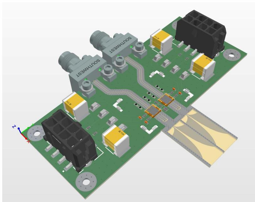
Figure 5-116 DRIFT Demonstrator PCB with Vivaldi.
