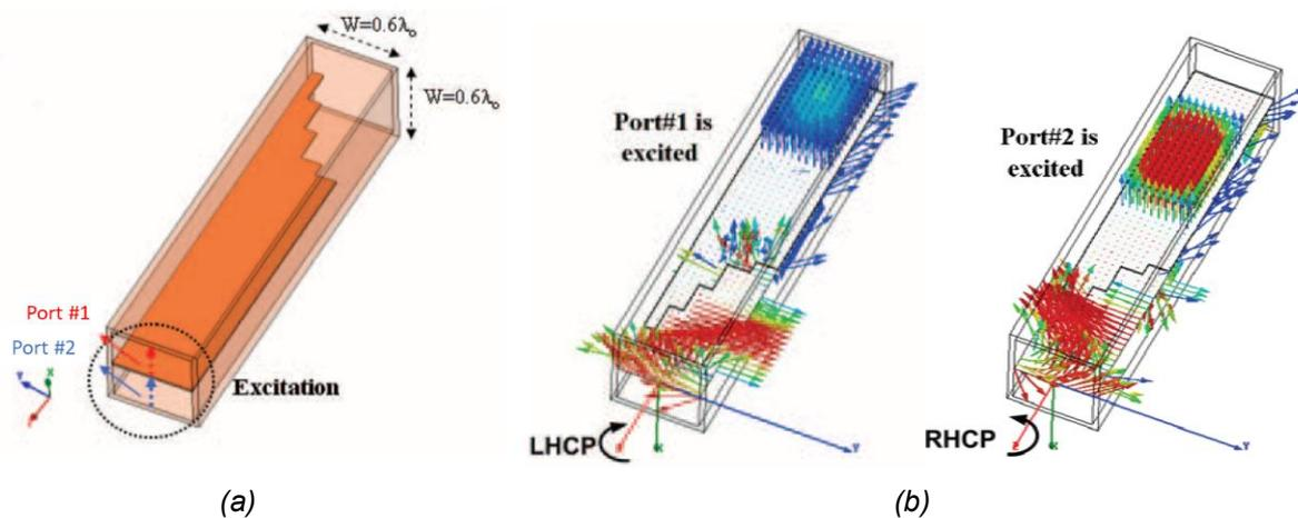
Figure 5-4: (a) Geometry of the square waveguide with a stepped septum circular polariser from [[13]], and (b) field distribution due to even mode excitation (left) and odd mode excitation (right). Note that the length orientation of the waveguides in (b) is opposite to the one shown in (a).
