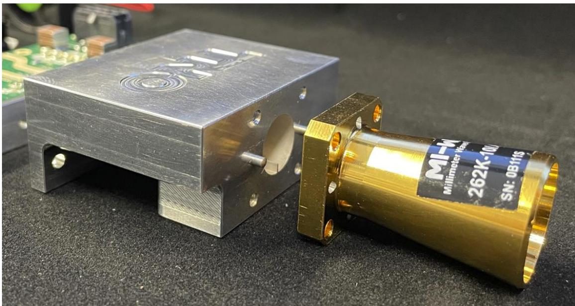
Figure 6-35 DRIFT waveguide viewed from the horn connection side.
