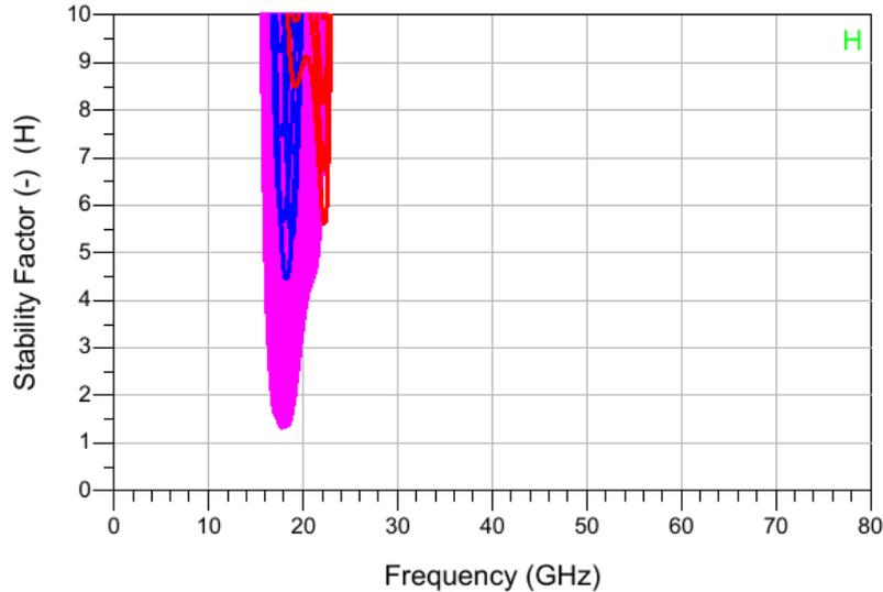
Figure 5-83 : Stability factor for  $T_a = -40\text{degC}$  (red),  $20\text{degC}$  (blue) and  $80\text{degC}$  (magenta), at  $V_g = -4.0$  to  $-2.5\text{V}$ ,  $V_d = 20\text{V}$ .
