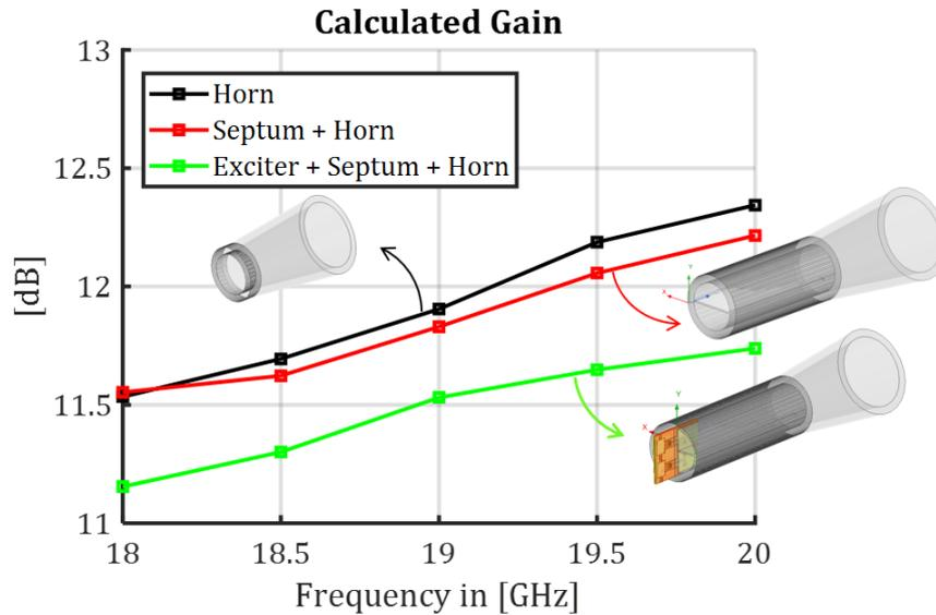
Figure 6-45: Calculated gain levels for the different structural portions of the passive frontend.
