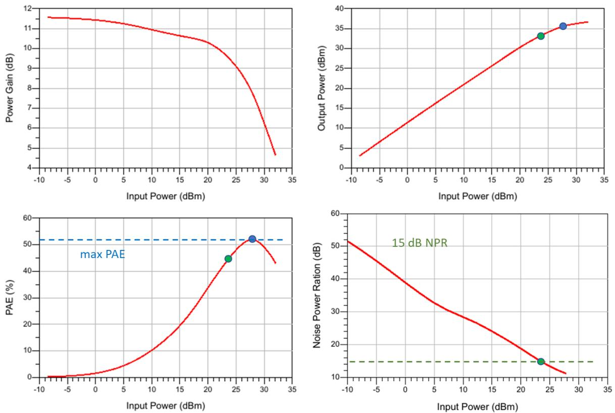
Figure 5-7 : Simulated 8x125um transistor performance at  $V_d=20V$ ,  $V_g=-3.0V$ , Frequency 20GHz, compromise load including harmonic source and load tuning,  $T_a=70^\circ C$ .
