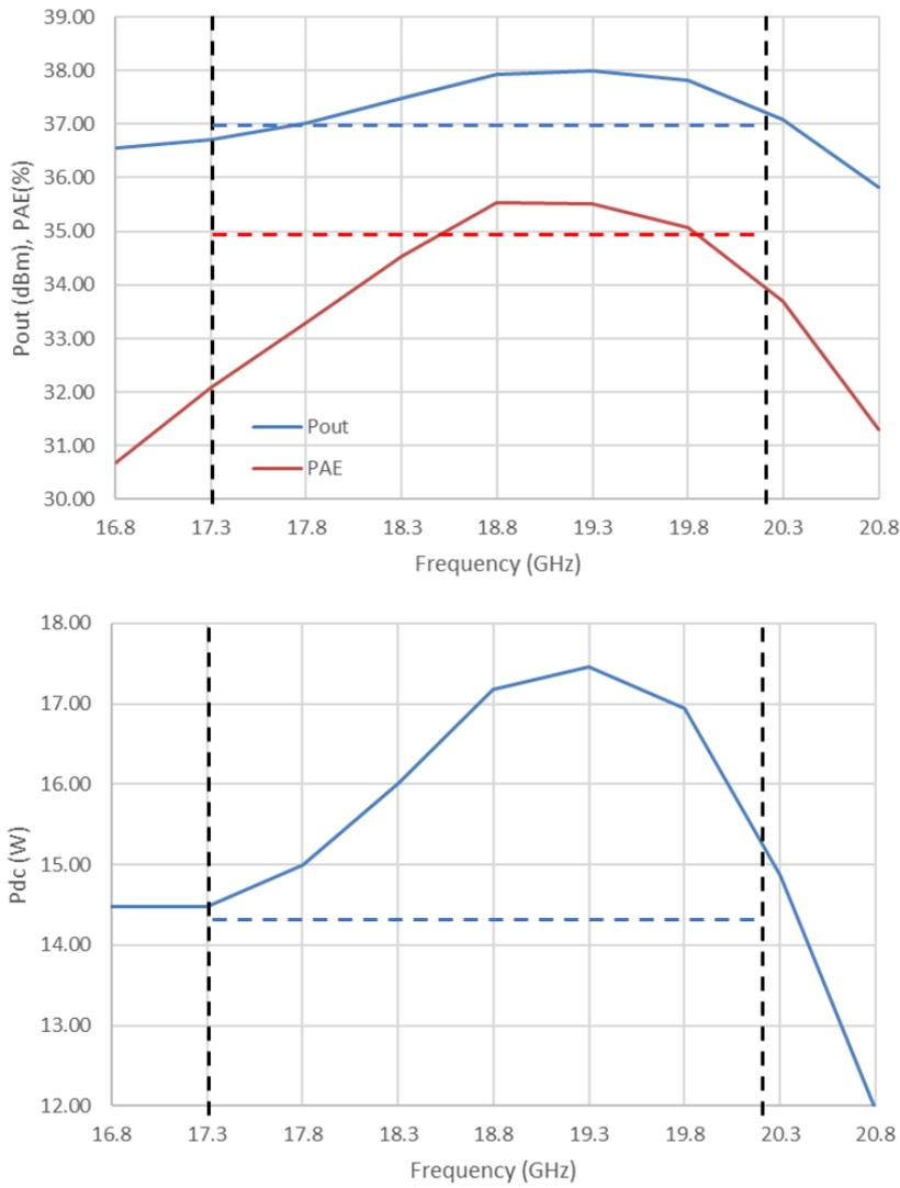
Figure 5-81 : Output power, efficiency and DC power consumption, calculated by IMAL for the 15 dB NPR point at  $V_g = -3.1V$ ,  $V_d = 20V$ ,  $T_a = 80degC$ .
