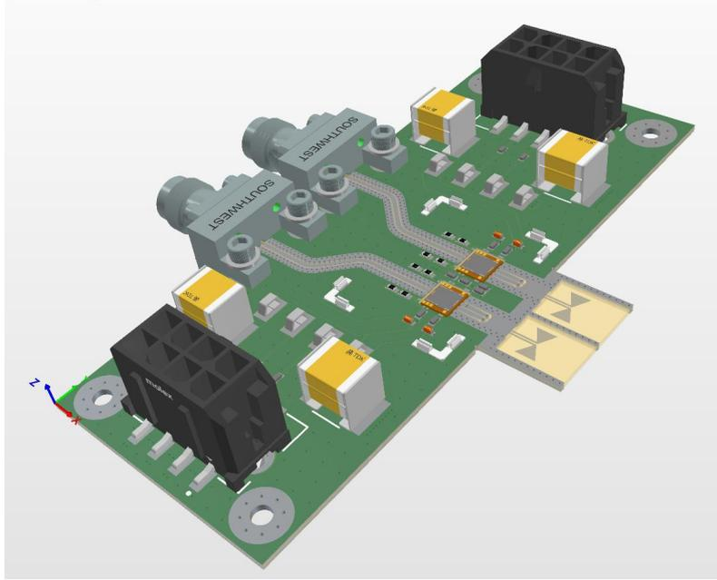
Figure 5-115 DRIFT Demonstrator PCB with Dipole.
