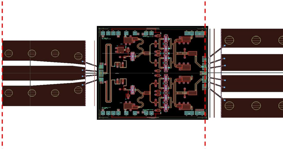
Figure 5-66 : Reference planes (red dotted lines) for the HPA performance simulations.
