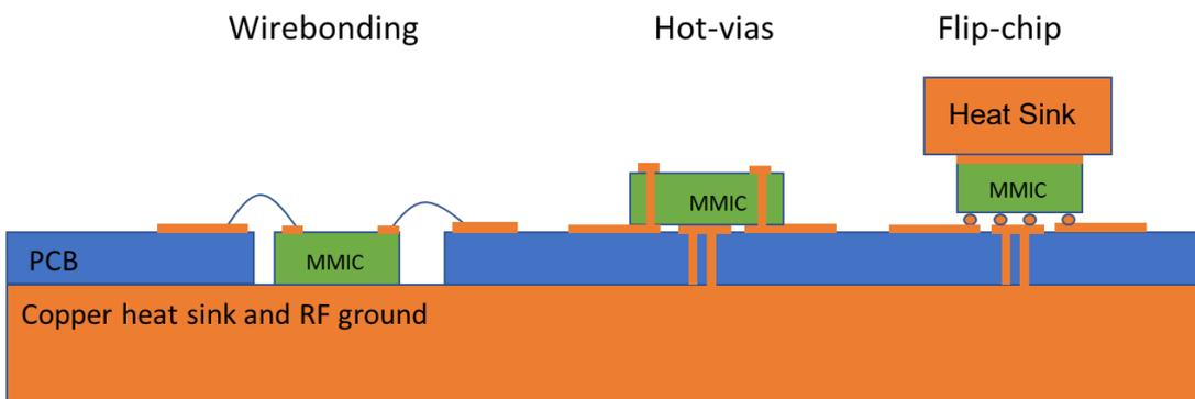
Figure 5-3 : Overview of MMIC mounting technologies.
