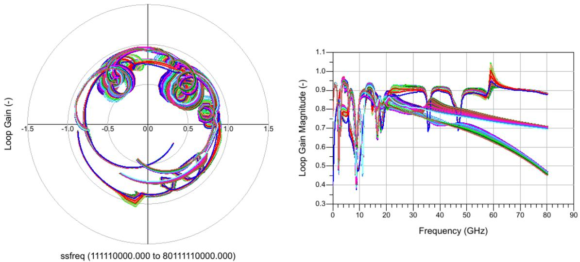
Figure 5-89 : Loop gain analysis for a source power range of -25 to +25 dBm at 18.8 GHz, gate bias range of -3.4 to -2.7V, at  $V_d = 20V$ ,  $T_a = 25degC$ , 50ohm output load, showing the loops at the gates of the input and output stage.
