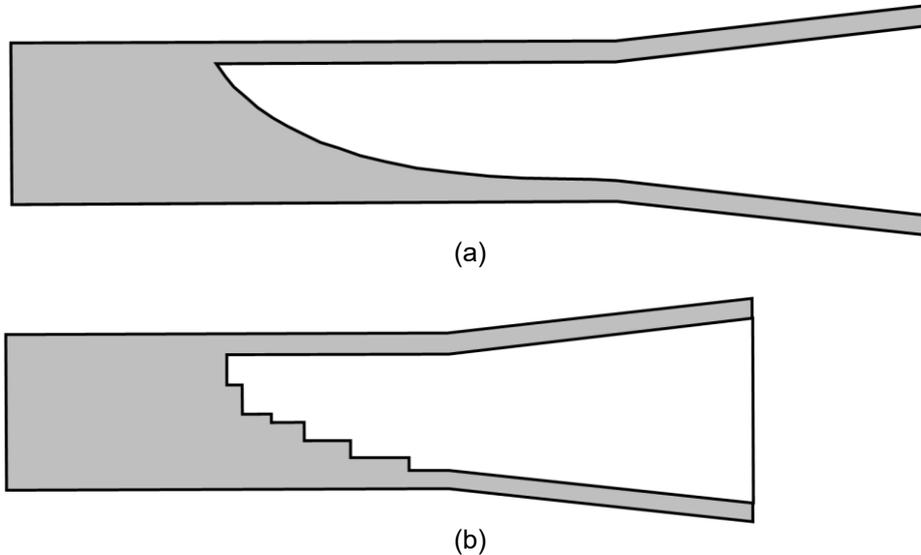
Figure 5-101: Different polarising septum solutions: (a) exponentially tapered 91mm, and (b) stepped 76mm.
