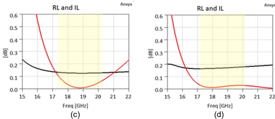
Figure 5-46 : (a) and (c) reflection (red) and transmission (green) performance in case of respectively the dipole and Vivaldi exciter. (b) and (d) losses idem, RL (red), IL (black).
