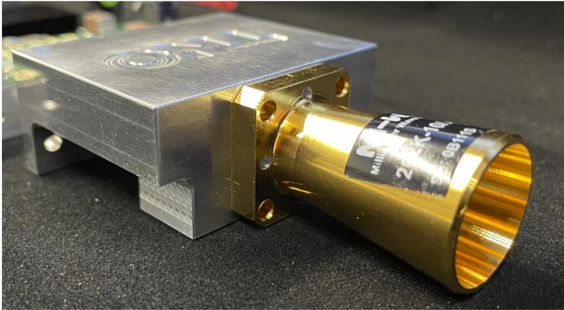
Figure 6-38 DRIFT waveguide and horn assembled.
