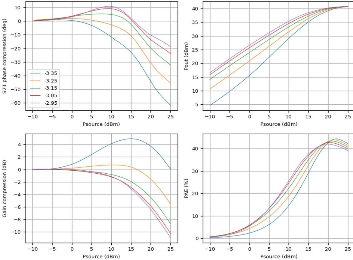
Figure 6-21 Power sweep measurements at 19 GHz versus gate bias at 20V, 80degC, sample R2C1.
