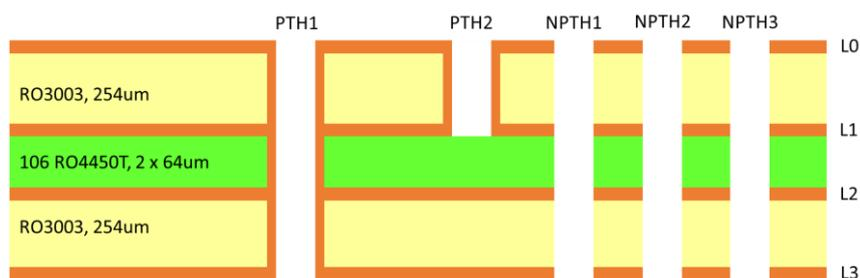
Figure 5-53: Layer stack used for the prototype PCBs. Also the different PTHs and NPTHs are indicated. The latter are necessary for mounting purposes (screws).
