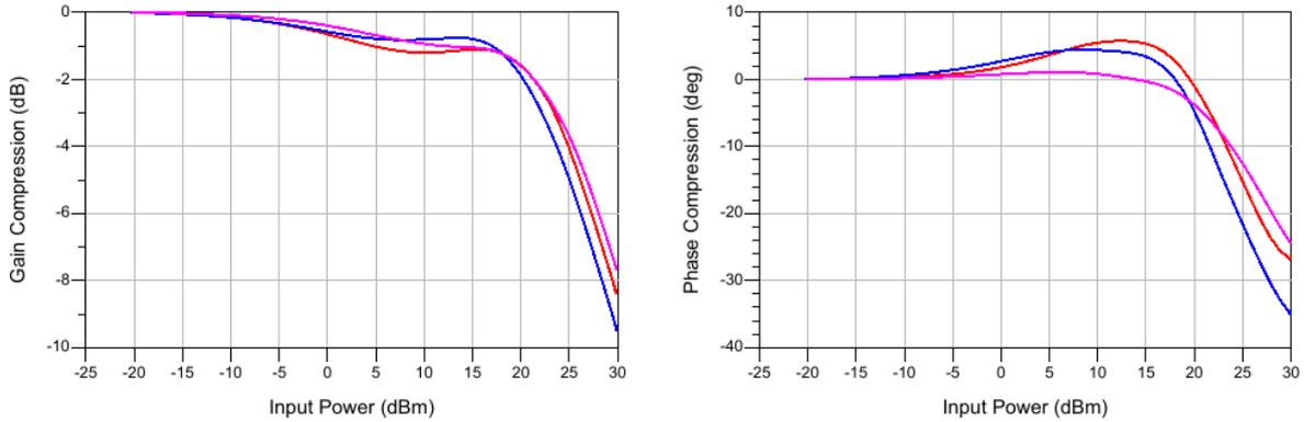
Figure 5-32 : Gain and phase compression at 17.3 GHz (red), 18.8 GHz (blue) and 20.3 GHz (magenta).
