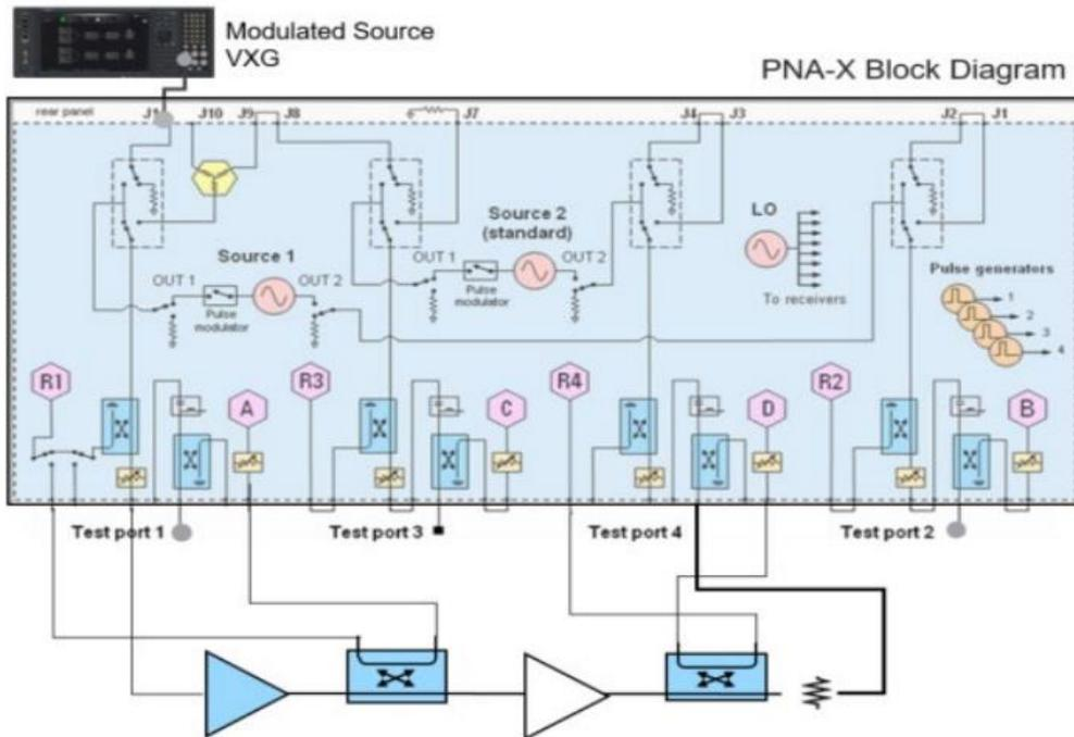
Figure 5-122 : Example of a measurement setup for non-linearity characterization.
