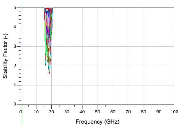
Figure 5-37 : Calculated stability factor from the S-parameter simulation for  $V_d = 2$  to  $20$  V and  $V_g = -5$  to  $-2$  V.
