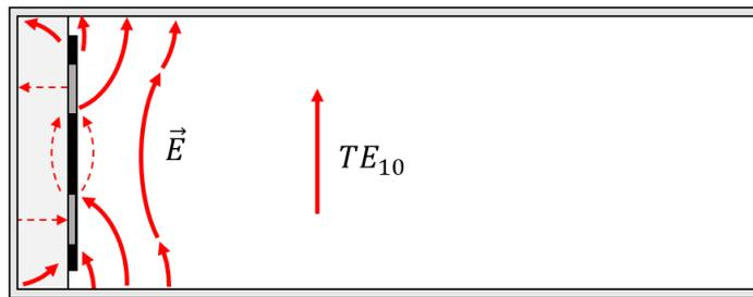
Figure 5-45 : Substrate hosting differential feeding line and patch placed on the back wall of the waveguide interior. Structure is observed looking along the differential line (two light grey rectangles), the differential mode field lines are dashed.
