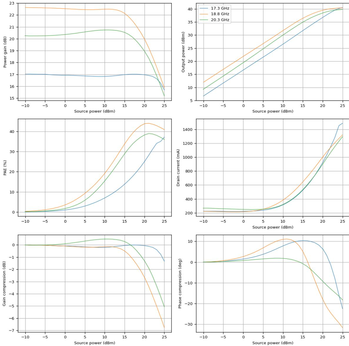
Figure 6-24 : Power sweep measurements at 80°C, at three frequencies, showing also the gain and phase compression for the combined differential output, as input for the IMAL calculations.
