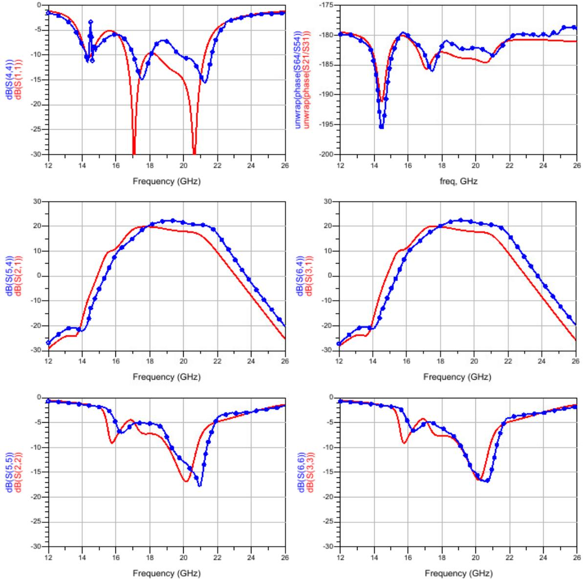
Figure 6-9 : Comparison of simulation (red) and measurement (dotted blue, sample R2C2) at  $V_d=20V$ ,  $I_{dq}\sim 140mA$ ,  $T_a=25degC$ .
