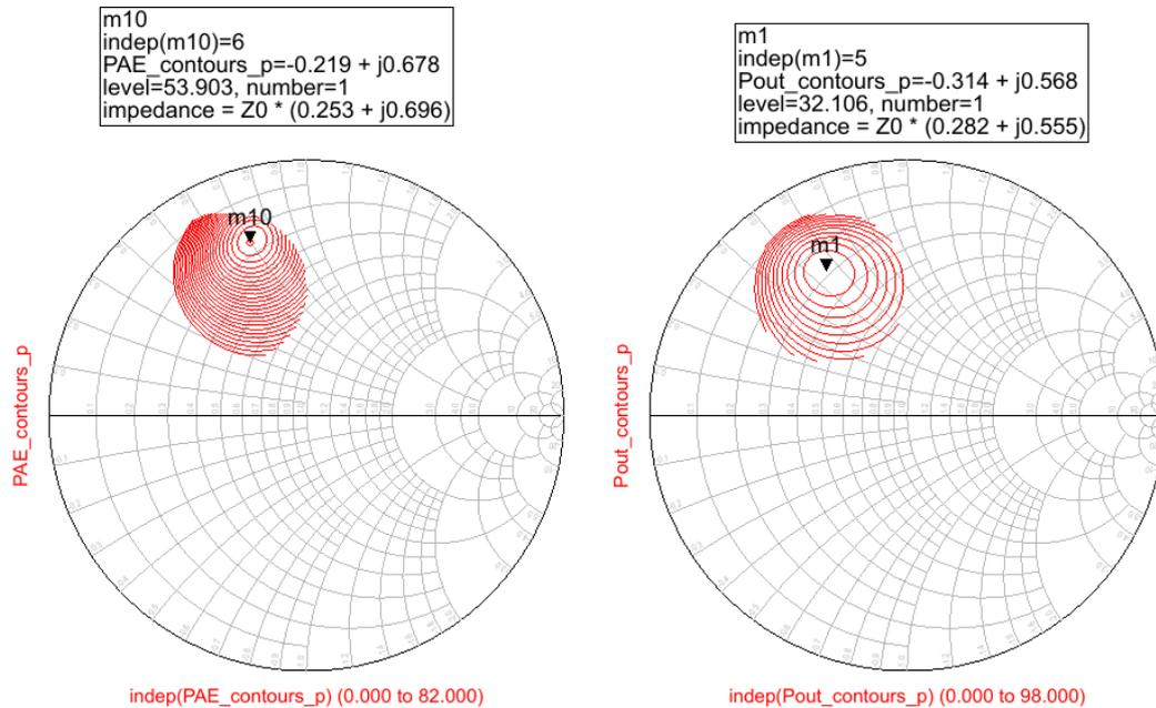
Figure 5-18 : Example load pull simulation of an 8x60um transistor at  $V_d=20V$ ,  $V_g=-3.1V$ ,  $P_{avs}=22dBm$ , 18.8 GHz,  $T_a=80^\circ C$ , no 2<sup>nd</sup> harmonic optimization.
