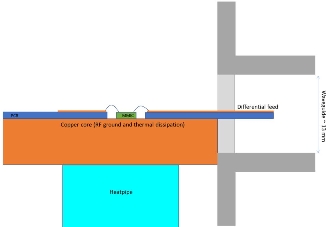
Figure 5-9 : Cross-section example for the case of an E-plane inline waveguide feed (brick architecture), only showing 1 polarization (not fully to scale).
