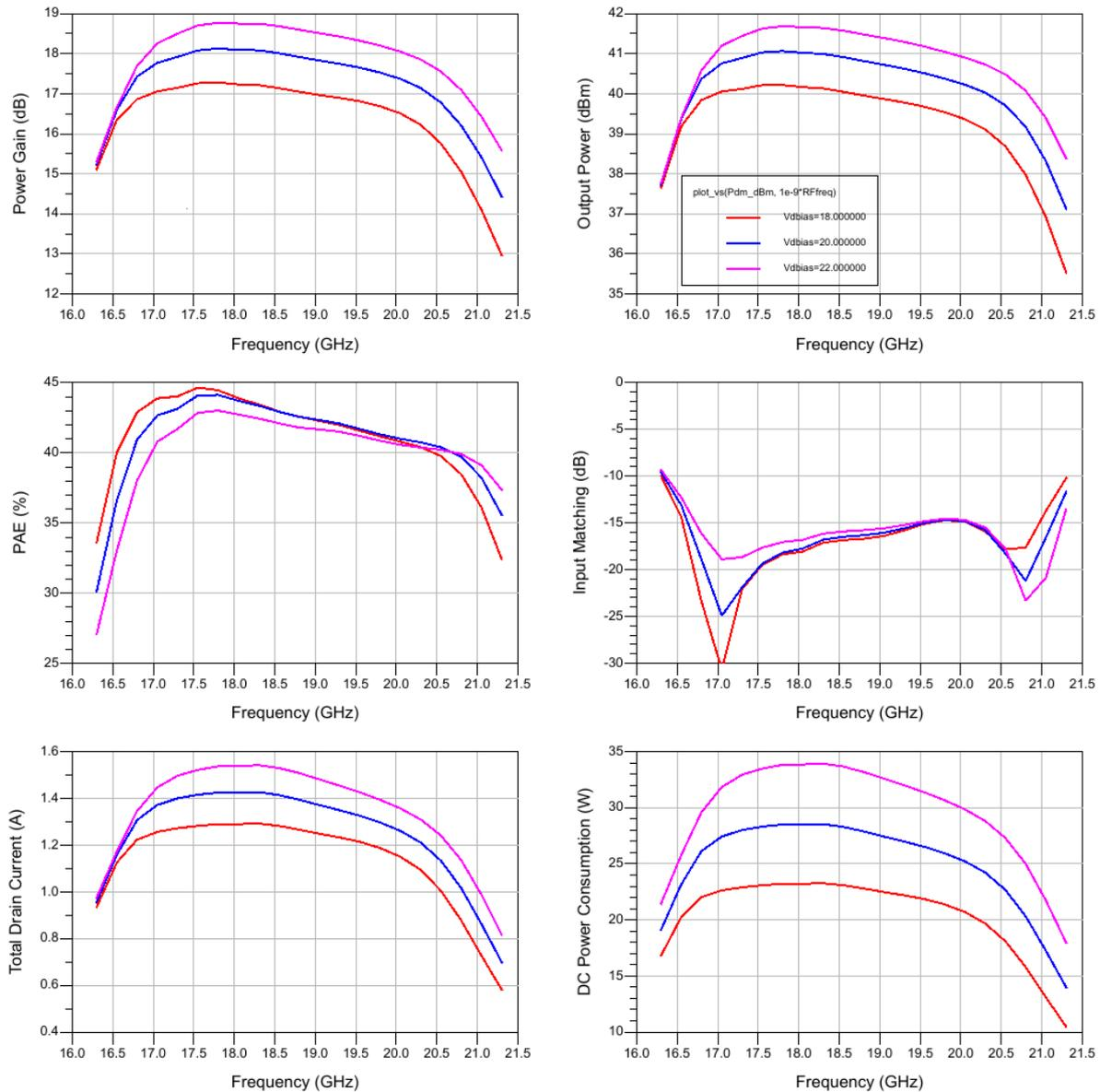
Figure 5-75 : Frequency sweeps at 23 dBm source power for Vd = 18, 20 and 22 V with Vg=-3.1 V.
