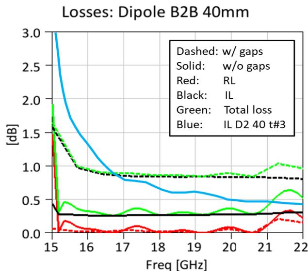
Figure 5-62: Comparison of the losses (see legend) between the structure with and without perfect aluminium connections (i.e. gaps), for the 40mm back-to-back dipole case. Losses in the structure with gaps start to resemble those that were measured. Characteristic are the high roll off at the lower frequency extreme and the counter intuitive monotonic decrease with higher frequency.
