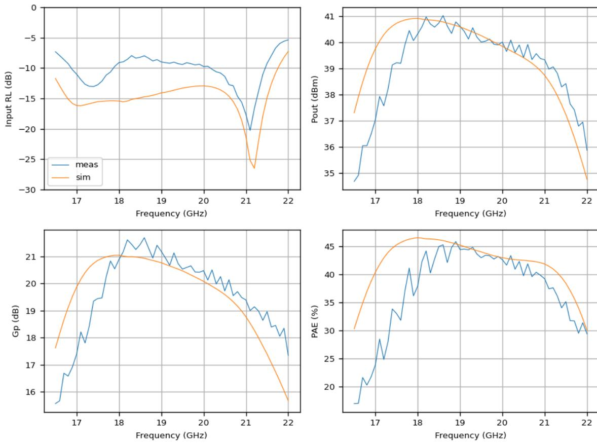
Figure 6-17 : Comparison of the measured and simulated CW frequency sweep for a source power of 20 dBm, at the nominal quiescent bias current of 140 mA and 20V, 25degC, sample R2C1.
