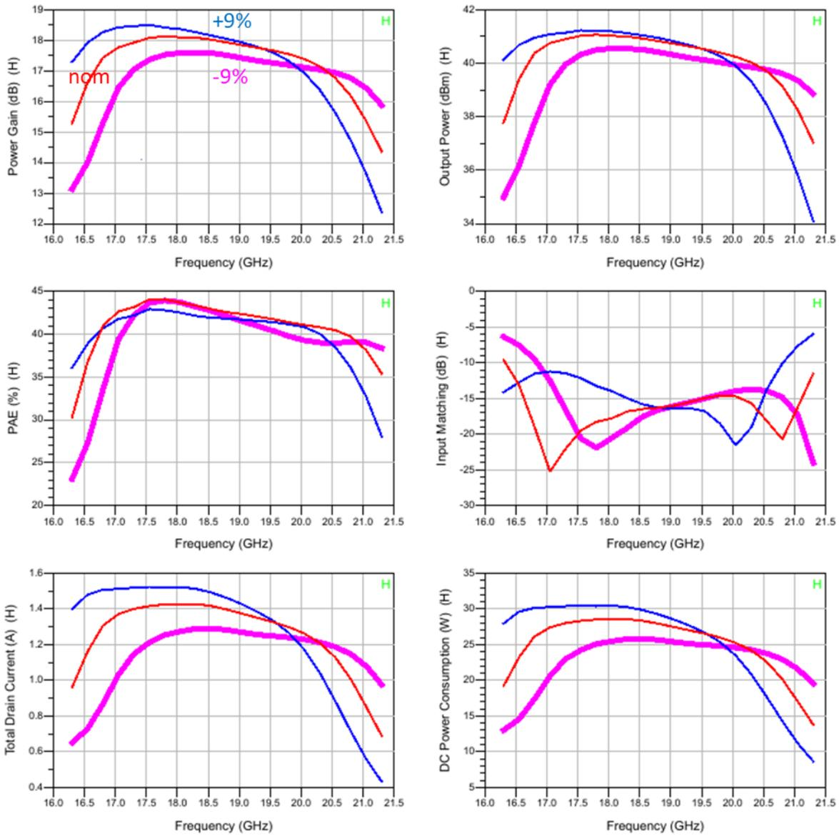
Figure 5-76 : Large-signal performance for 23 dBm source power and a +/- 9% MIM capacitor variation,  $V_g=-3.1$  V,  $V_d=20$  V,  $T_a=80$ degC.
