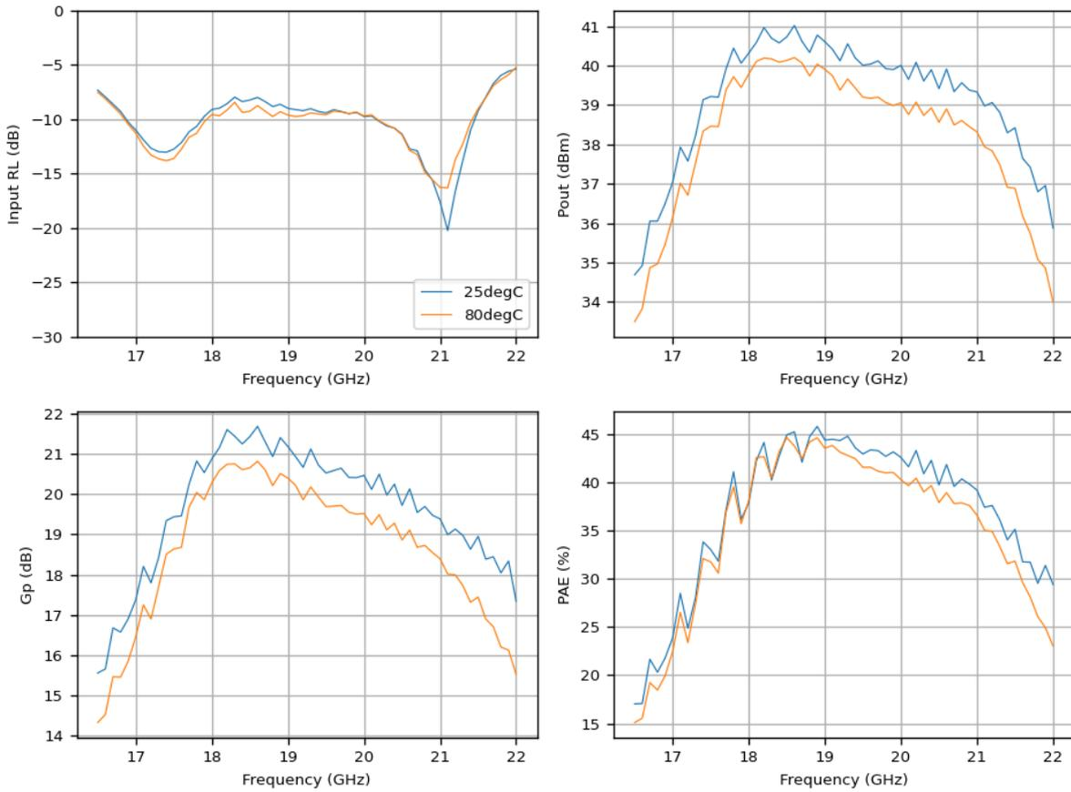
Figure 6-18 : Comparison of measured frequency sweep at 25degC and 80degC, at 20dBm source power for the nominal gate bias (-3.15V) at 20V, 25degC, sample R2C1.
