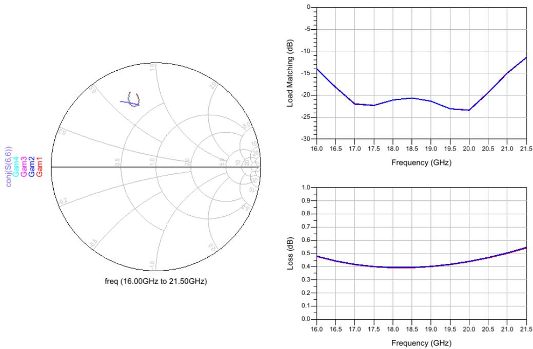
Figure 5-20 : Simulated performance of the initial output matching network.
