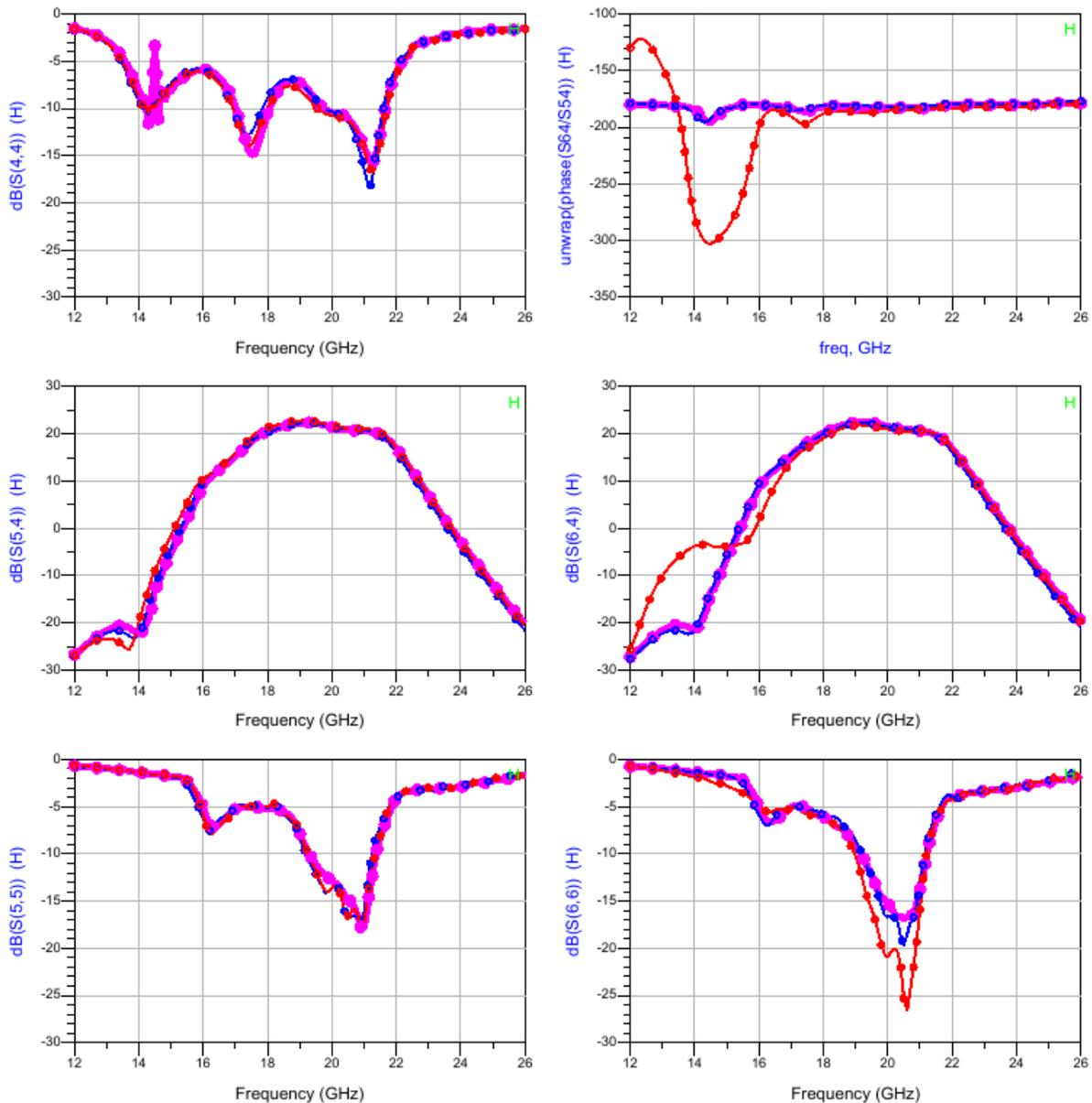
Figure 6-8 : S-parameter measurements of the 3 mounted samples at  $V_d=20V$ ,  $I_d\sim 140mA$ ,  $T_a=25degC$ .
