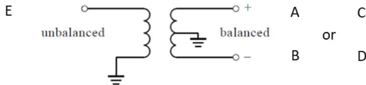
Figure 5-131: Balun outputs connected to either the input port combination A and B, or C and D, for generating the polarisation senses.
