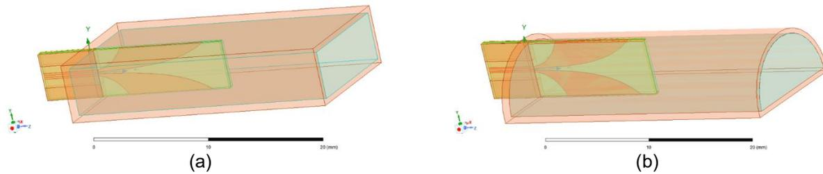
Figure 5-48 : (a) Vivaldi exciter in rectangular, and (b) semi-circular waveguide.
