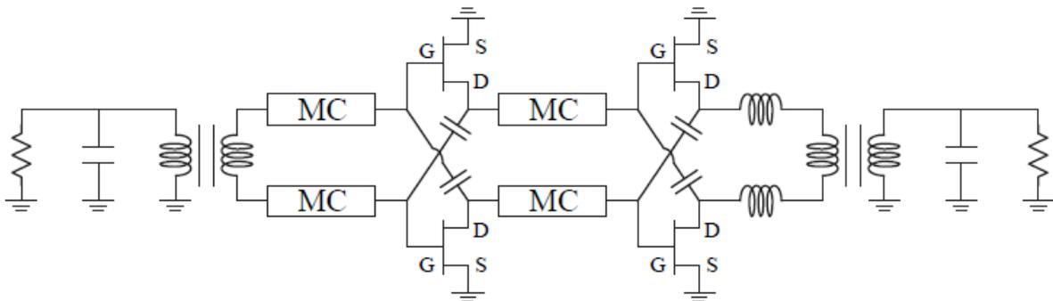
Figure 5-39 : Possible Implementation of the capacitance neutralization.
