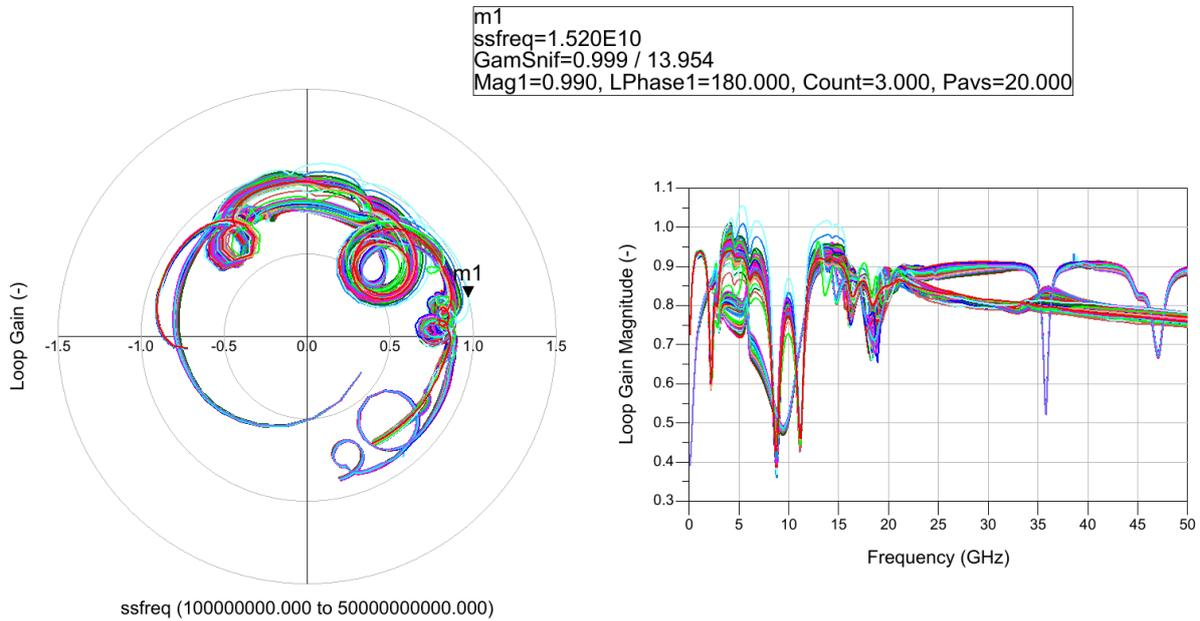
Figure 5-90 : Loop gain analysis for a source power range of -25 to +25 dBm at 18.8 GHz,  $V_g = -3.1V$ ,  $V_d = 20V$ ,  $T_a = 25degC$ , output load sweep magnitude 0.33, 0.66 and 0.99 with phase from 0-360deg, showing the loops at the gates of the input and output stage.
