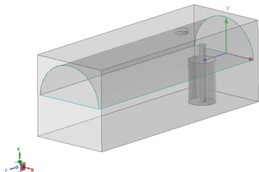
Figure 5-126: CAD-model of the transition from coaxial cable to the semi-circular wave guide.
