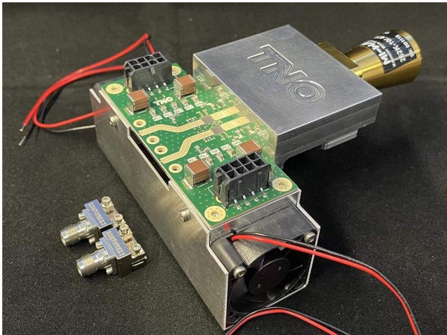
Figure 6-27 DRIFT Demonstrator Assembled and Integrated.
