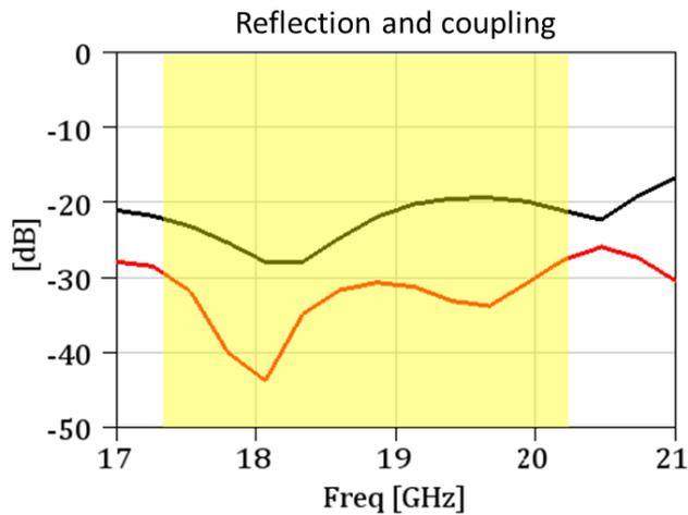
Figure 5-103: Reflection seen at the input of a single exciter (black curve), and coupling between the two exciters (red curve) which is very low.
