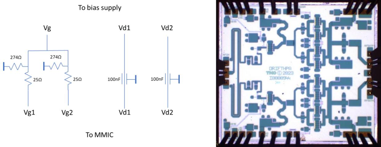
Figure 6-1 Decoupling on the DC probe card and Drift HPA on-wafer measurement
