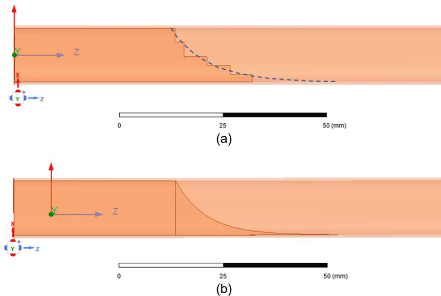
Figure 5-49: Septum simulation models. (a) Discrete steps, (b) continuous.
