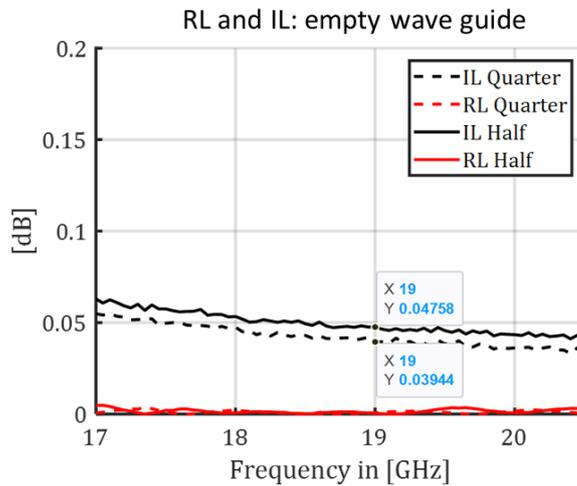
Figure 5-98: Measured losses of the empty  $\lambda_g/4$  and  $\lambda_g/2$  waveguide sections.
