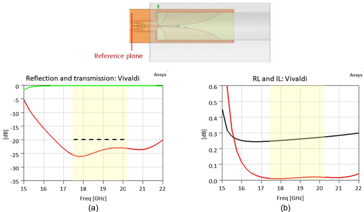
Figure 5-55: Vivaldi exciter tuned performances. (a) Reflection and transmission, and (b) reflection- (red) and insertion (black) losses. Results are valid reference to indicated plane in schematic.
