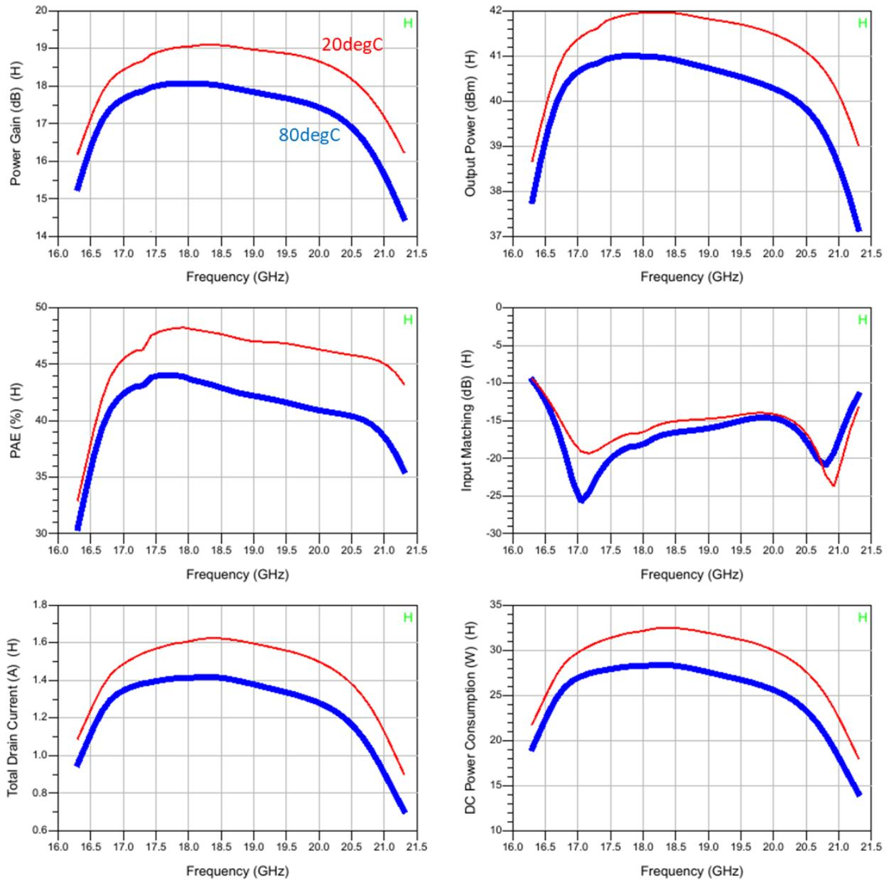
Figure 5-78 : Frequency sweeps at 23 dBm source power at  $V_g = -3.1$  V,  $V_d = 20$  V for  $T_a = 20$  and 80degC.
