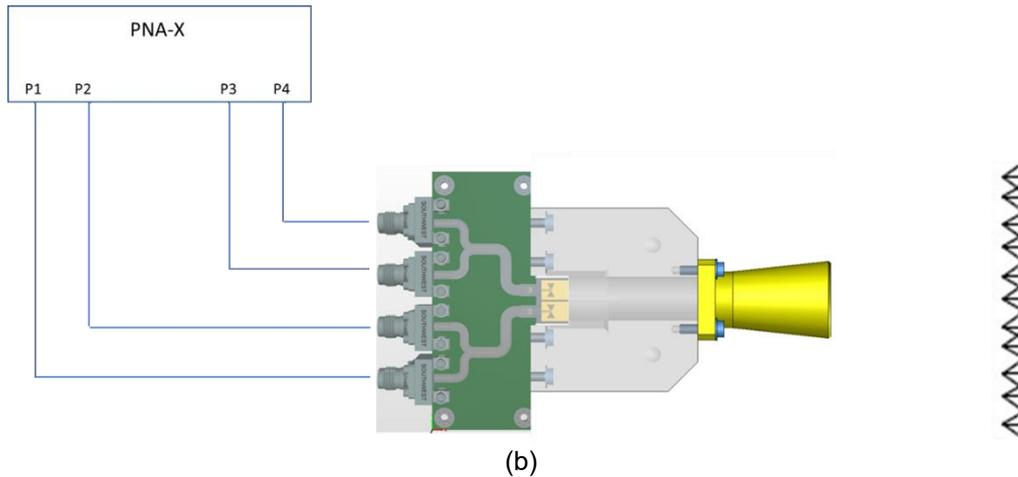
Figure 5-128: (a) Example of the routing for the passive demonstrator test. It will involve 4 Southwest connectors. The dashed red line represents the reference plane. (b) Test setup to measure the scattering parameters of the passive demonstrator.
