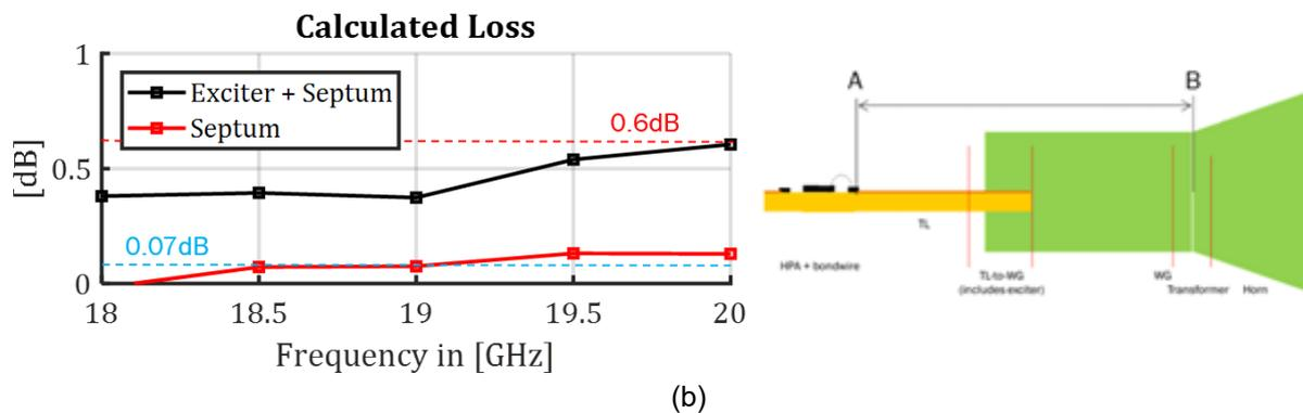
Figure 6-46: (a) Losses calculated from the results shown in Figure 6-45. (b) Losses in the graph relate to the part from A to B.
