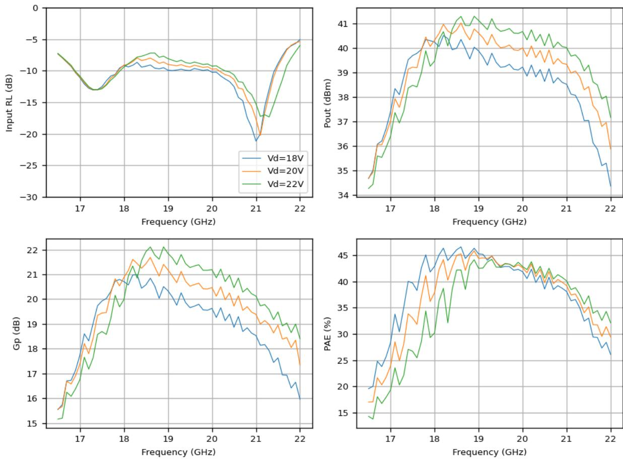
Figure 6-15 : Measured frequency sweep for a source power of 20 dBm, versus drain bias voltage at the nominal gate bias, 25degC, sample R2C1.
