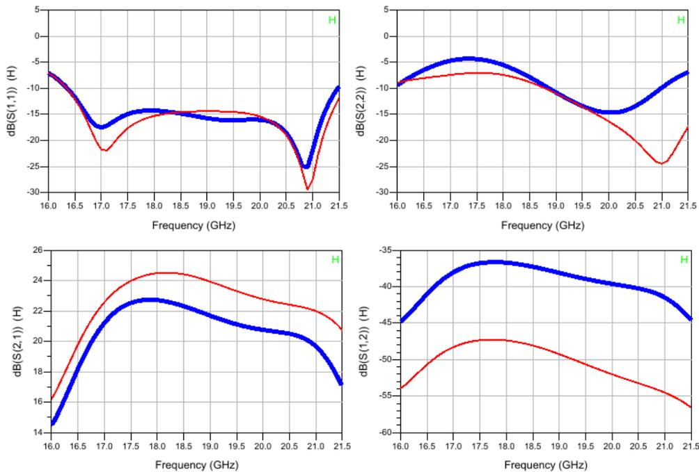
Figure 5-68 : Small-signal S-parameters for the HPA using an ideal balun at the output,  $V_g = -3.0V$  (20degC) and  $V_g = -3.1V$  (80degC),  $V_d = 20V$ ,  $T_a = 20degC$  (red) and 80degC (blue).
