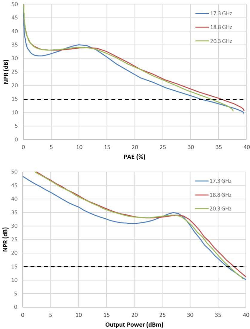
Figure 5-80 : NPR versus efficiency and output power at  $V_g = -3.1V$ ,  $V_d = 20V$ ,  $T_a = 80degC$ .
