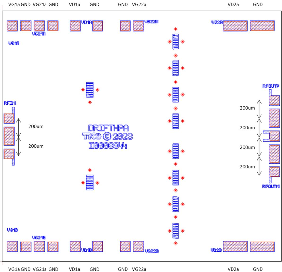
Figure 5-65 : DC and RF probe pad definitions.
