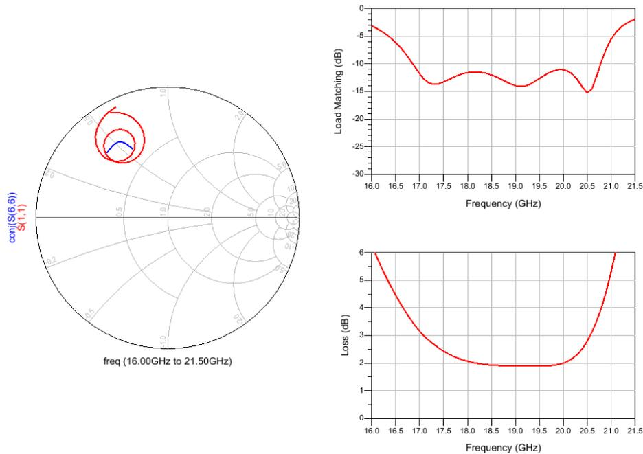
Figure 5-21 : Simulated performance of the initial interstage matching network.
