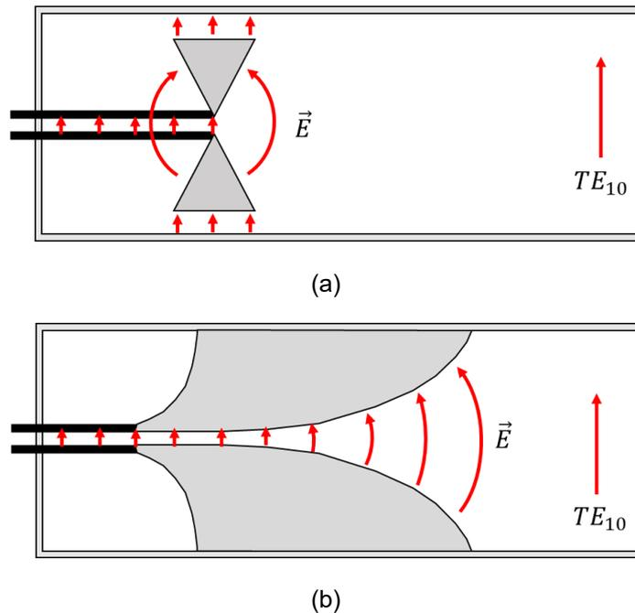
Figure 5-44 : (a) Dipole with feeding differential line entering waveguide to excite the fundamental waveguide mode, and (b) case Vivaldi.
