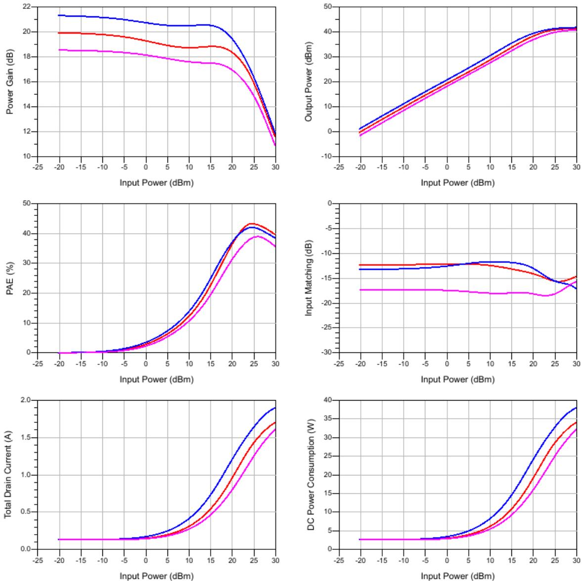
Figure 5-27 : Large-signal power-sweep at 17.3 GHz (red), 18.8 GHz (blue) and 20.3 GHz (magenta).
