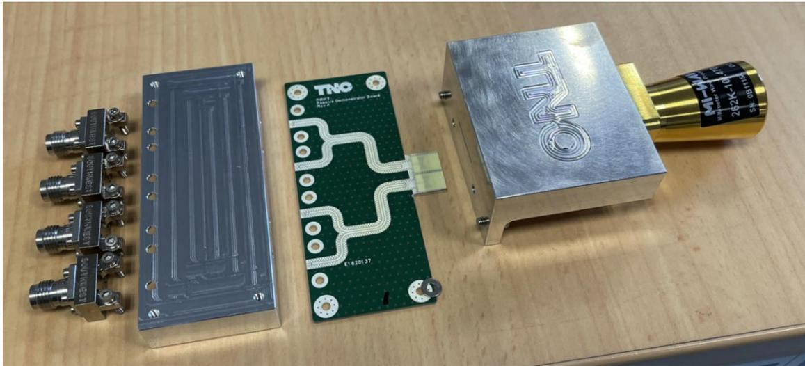
Figure 6-40 DRIFT passive antenna demonstrator components
