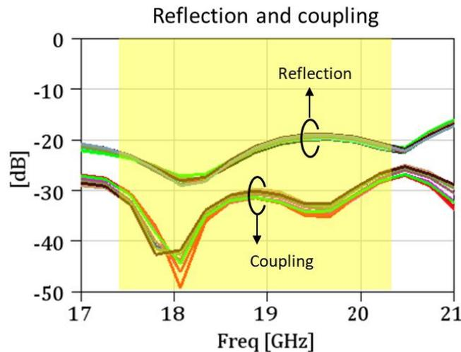
Figure 5-105: Variation in the reflection and coupling due to production tolerance on the polarising septum. Performances are quite clustered indicating tolerance effects are minimal.
