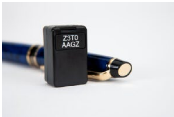
Figure 2-1: QuSpin QZFM Gen-3 OPM
