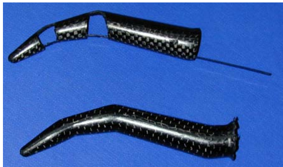
Figure 15: finger prototype before and after the cuts.
