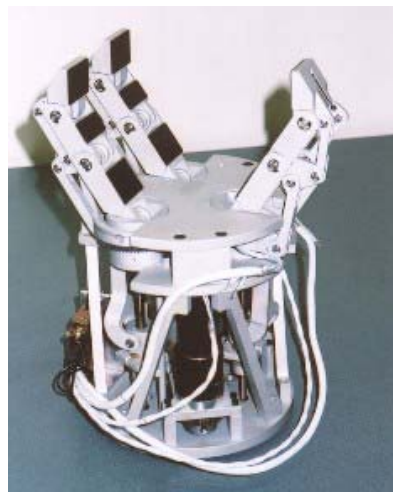
Figure 7: the new version of the underactuated 10-DOF Laval Robotic Hand.
