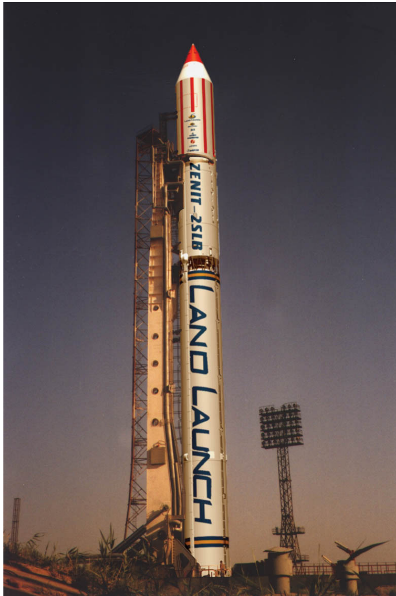
Figure 5.1 – Zenit-2 SLB Two-Stage Integrated Launch Vehicle
