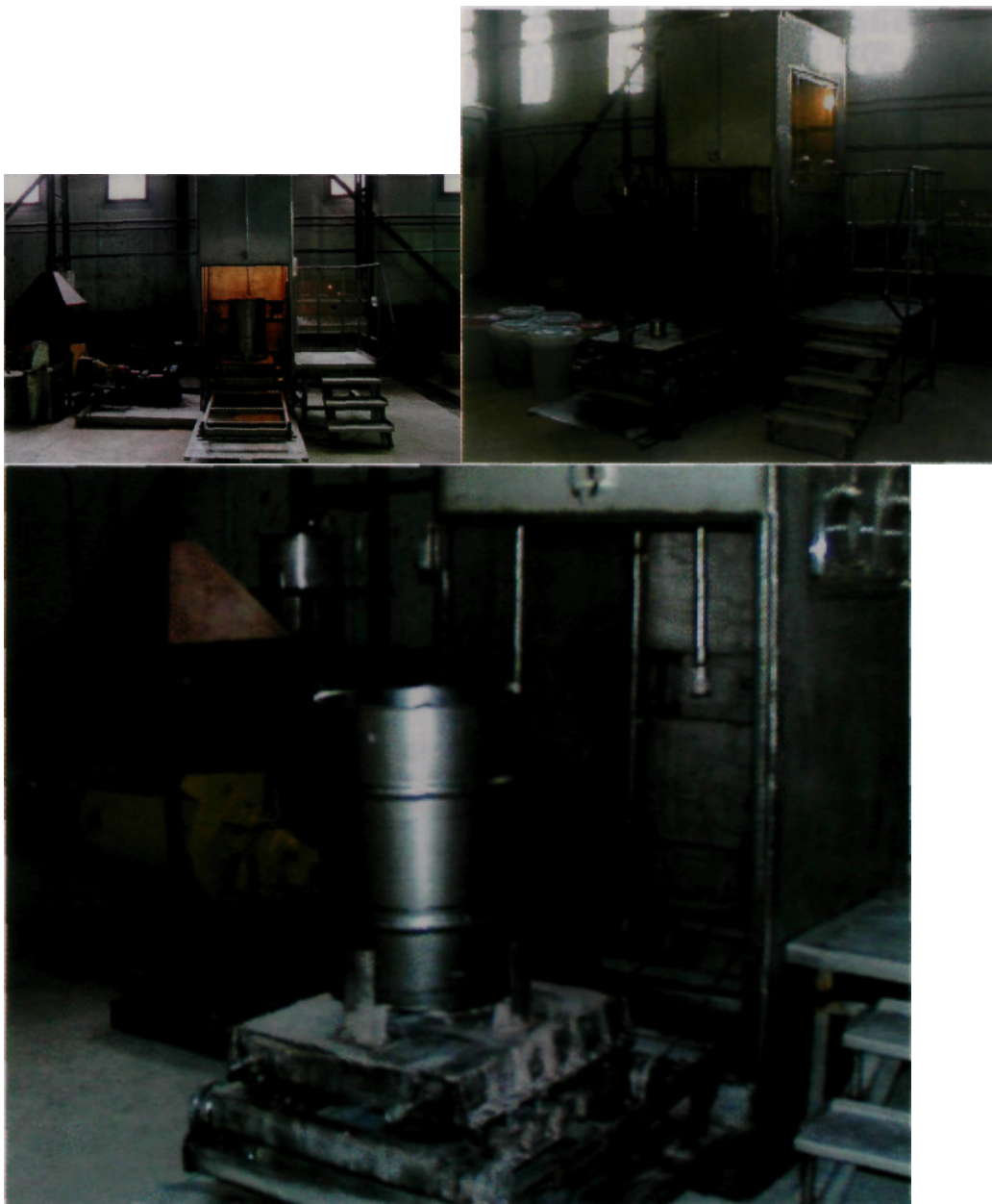
Fig. 2. The plant of cementation of ash remainder from burning of radioactive waste
