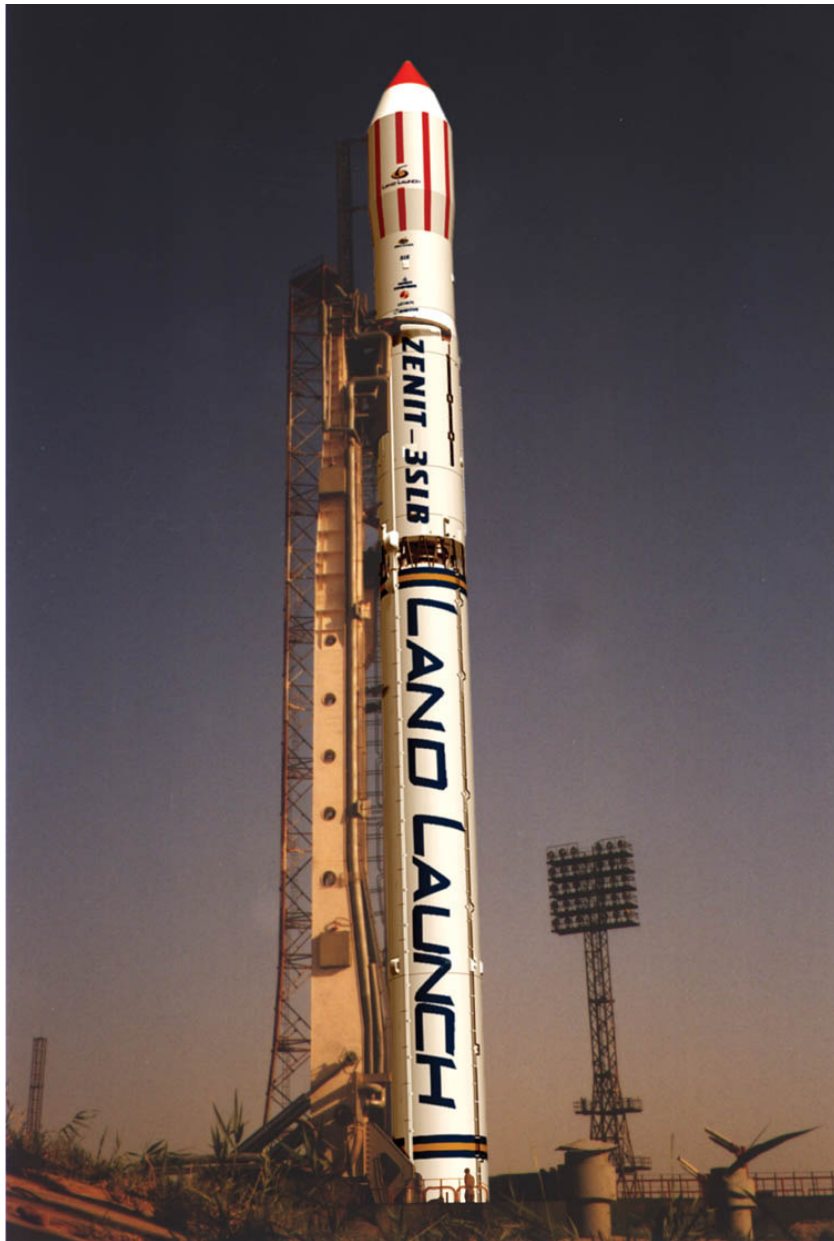
Figure 5.2 – Zenit-3 SLB Three-Stage Integrated Launch Vehicle
