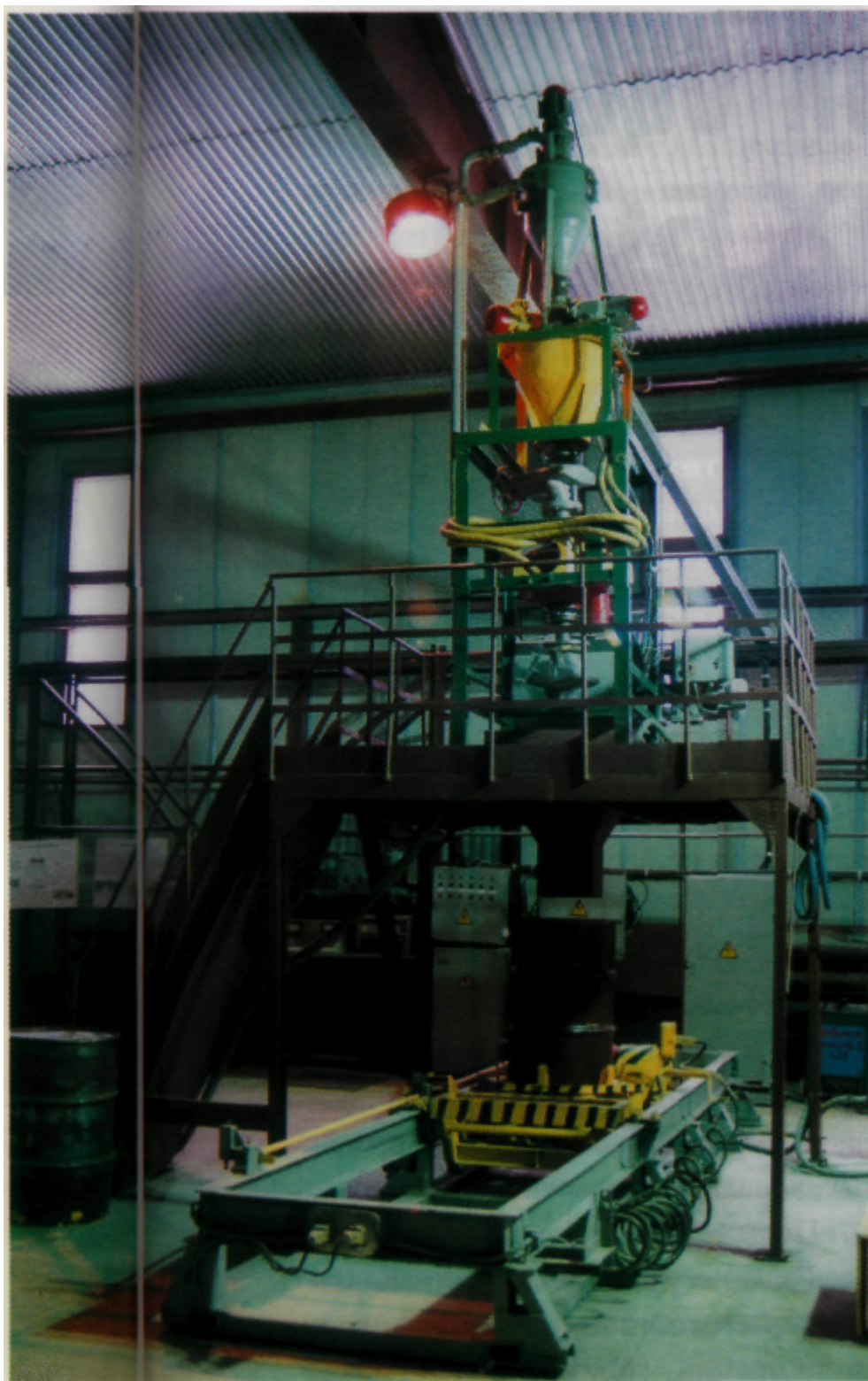
Fig. 5. The plant of cementation of liquid RW with the electromagnetic mixer
